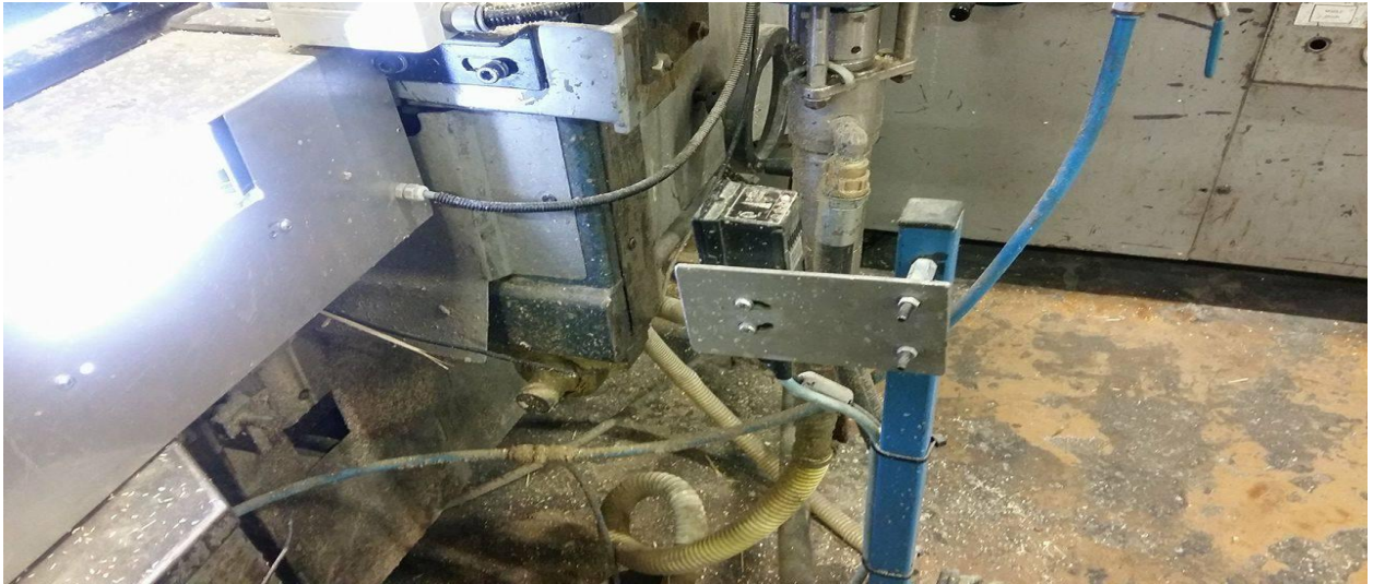
Figure 4.4 Camera stand with external lighting
