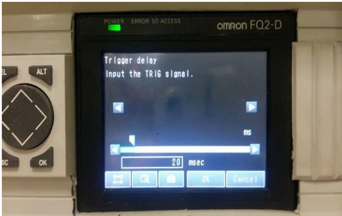
Figure 7.2 Camera triggering delay
