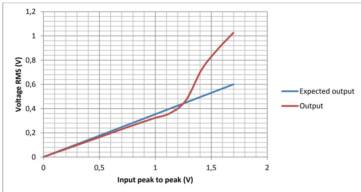
Figure 5.5. LTC1966 output comparison
