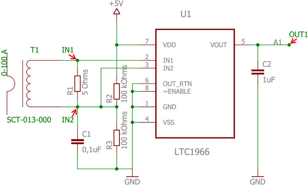
Figure 5.2. LTC1966 connection schematic
