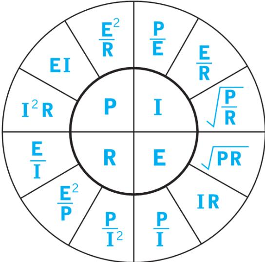
Figure 2.1. Collection of equations to find main electrical parameters [6]
