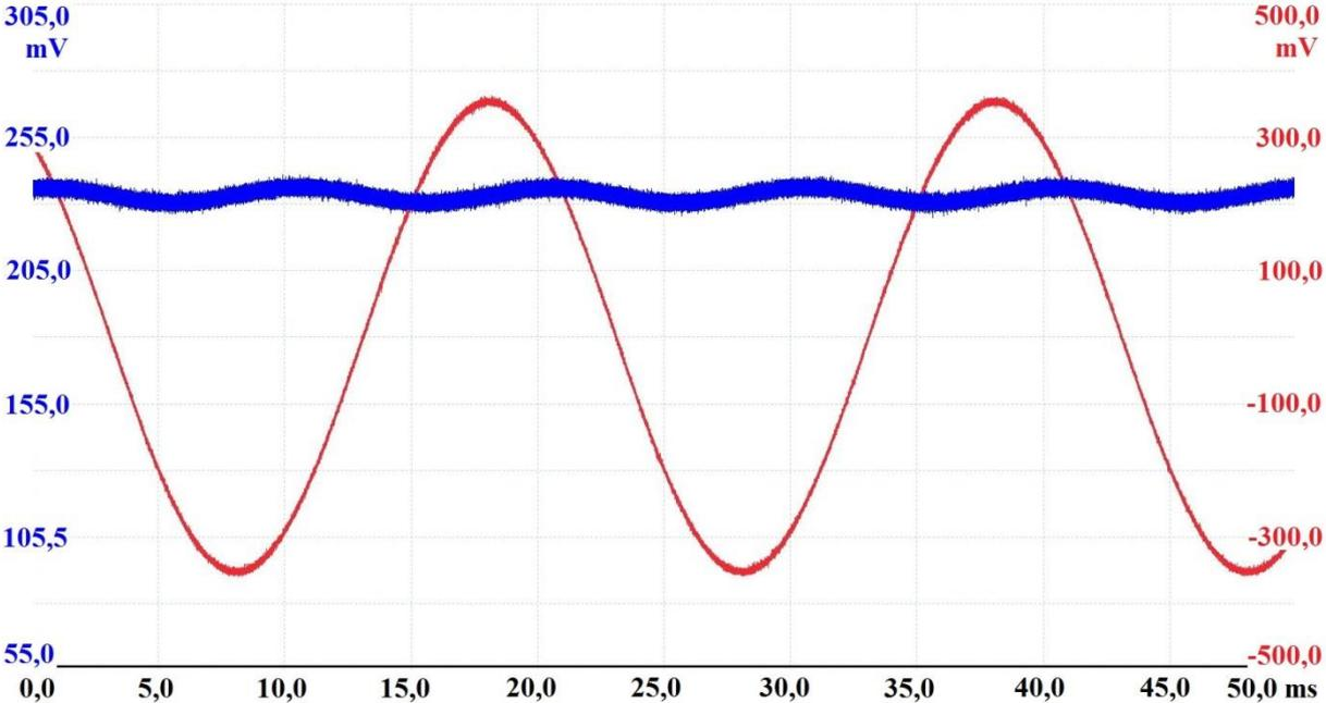
Figure 5.3. LTC1966 test circuit waveform comparison with 1  $\mu$ F averaging capacitor and 0,707 V peak to peak 50 Hz input
