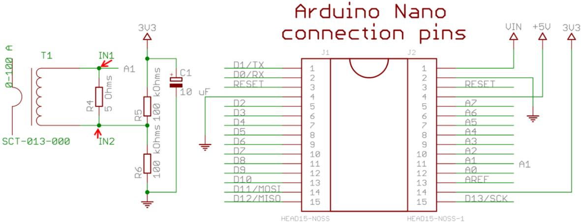
Figure 5.9. RMS measuring circuit based on Arduino Nano
