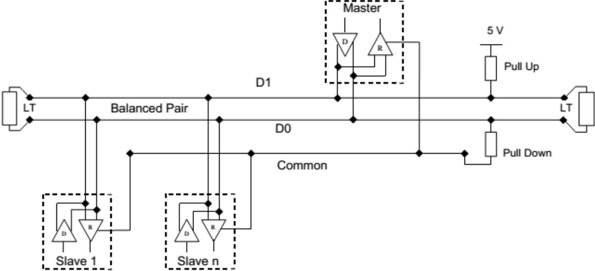
Figure 5.13. RS-485 two-wire (half-duplex) topology [32]
