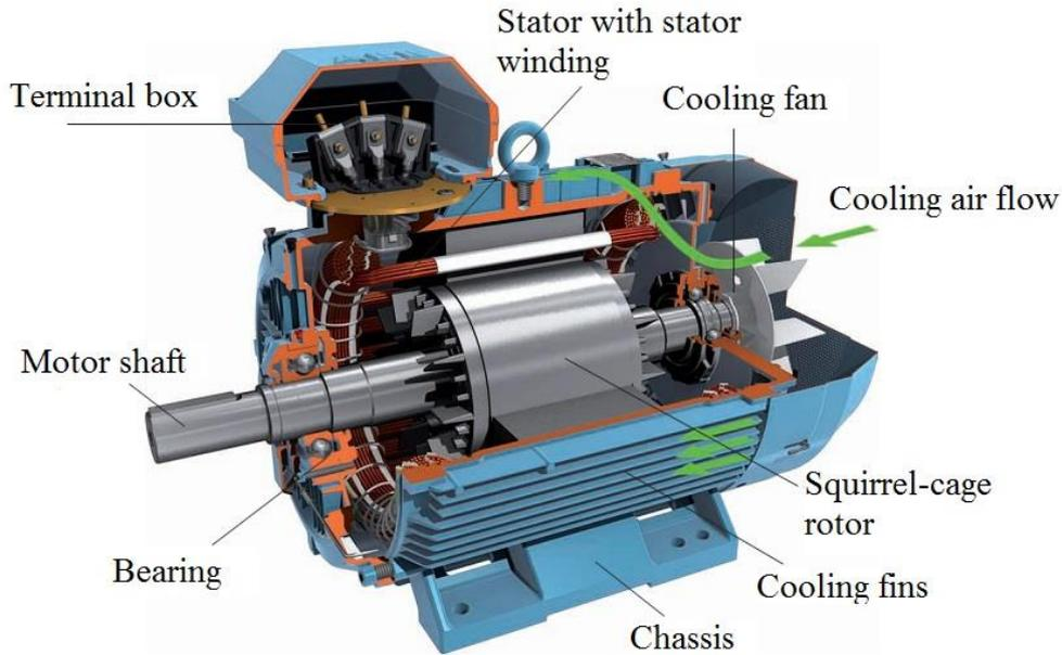
Figure 3.1. Three-phase asynchronous motor view [14]
