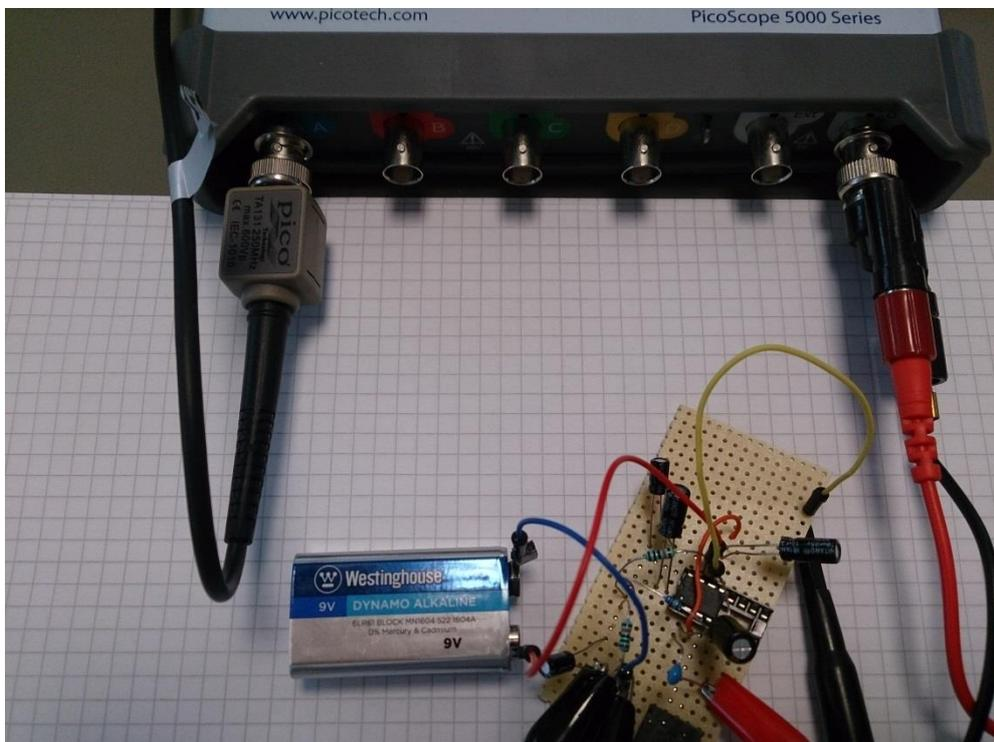
Measuring AD736J RMS to DC converter
