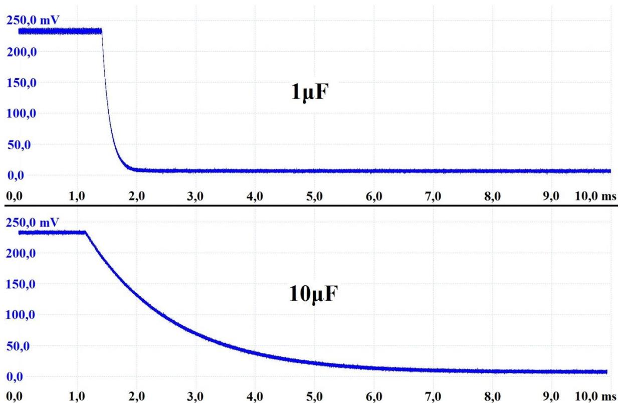
Figure 5.4. LTC1966 circuit output comparison with different capacitors
