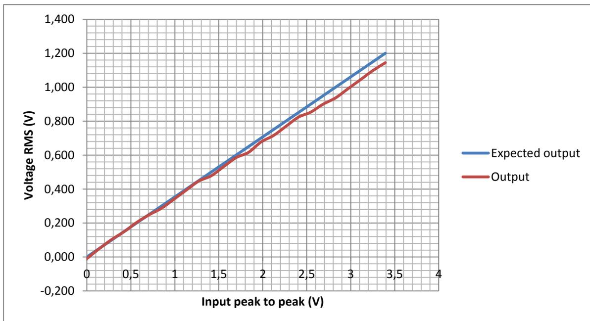
Figure 5.7. AD736J output comparison
