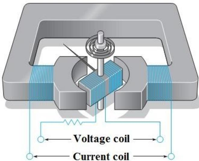
Figure 2.3. Simple wattmeter design [6]
