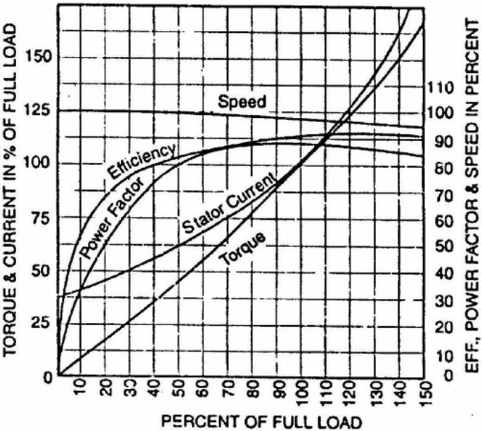
Figure 3.3. Performance curve of a three-phase squirrel cage motor [17]
