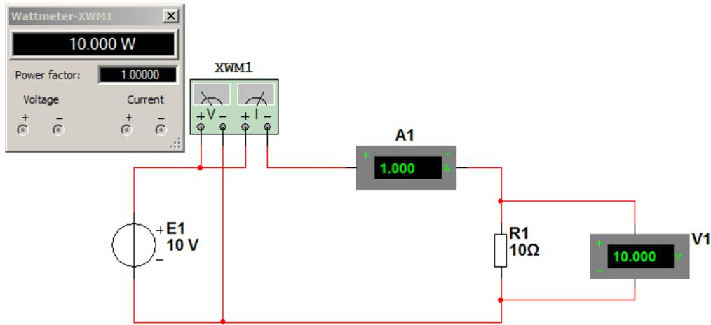
Figure 2.2. Power in simple series circuit
