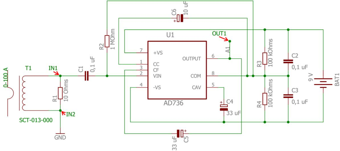
Figure 5.6. AD736J connection schematic
