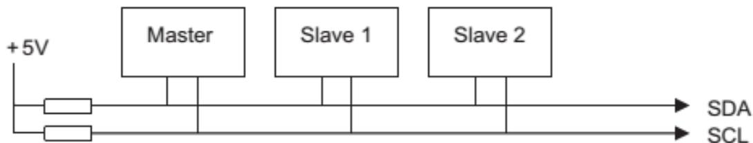
Figure 5.12. I<sup>2</sup>C bus connection [29]
