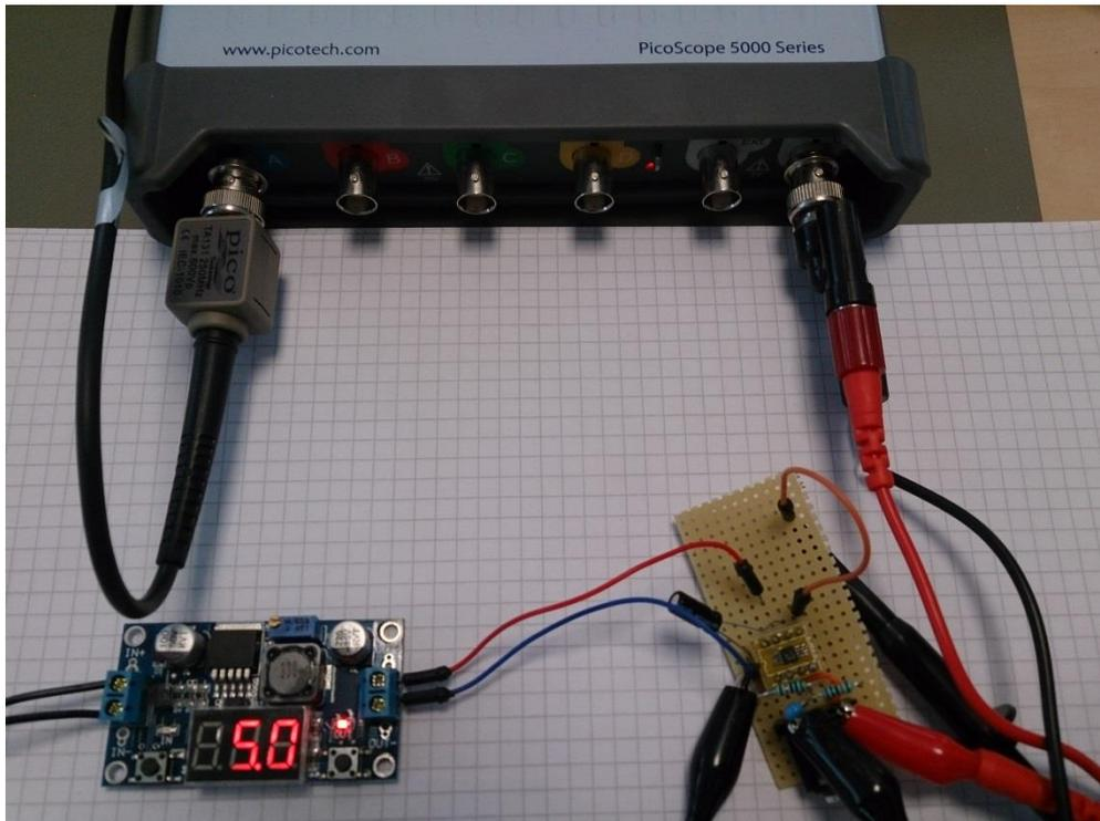
Measuring LTC1966 RMS to DC converter
