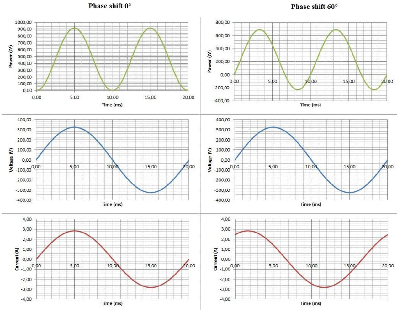
Figure 2.4. Sinusoidal waveforms of AC circuit
