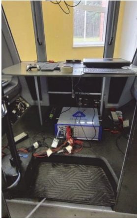
Fig. 7. Measuring setup with DEWETRON data acquisition system
