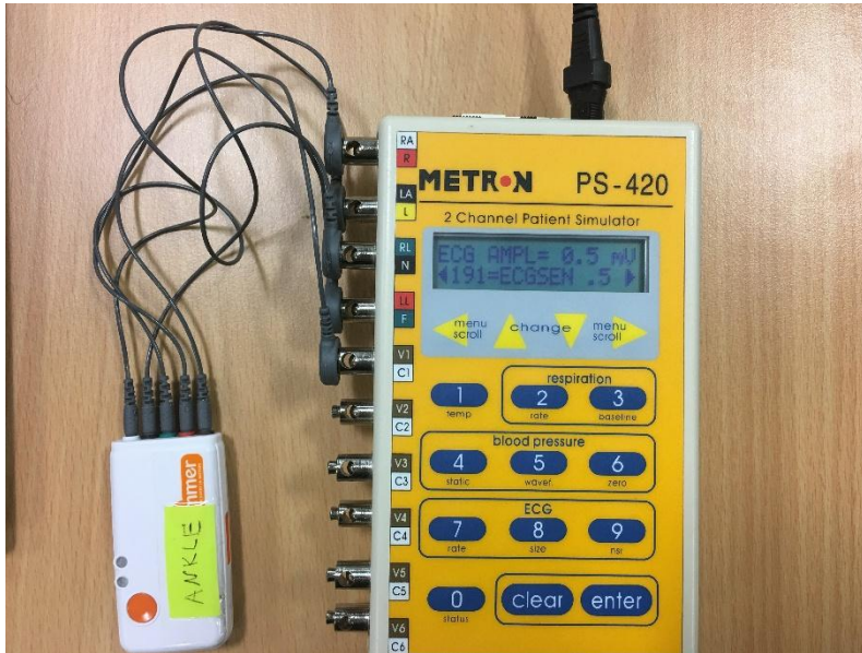
Figure 4. ECG test measurement with Patient Simulator Metron PS-420
