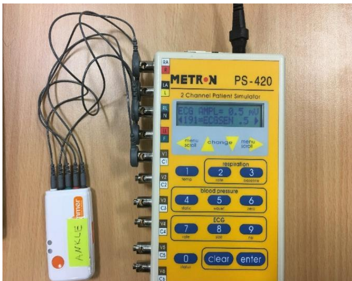
Figure 27. ECG test measurement with Patient Simulator Metron PS-420
