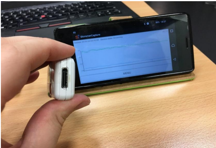
Figure 16. Streaming biosignals from Shimmer3 sensor to android mobile app ShimmerCapture via Bluetooth in real-time.
