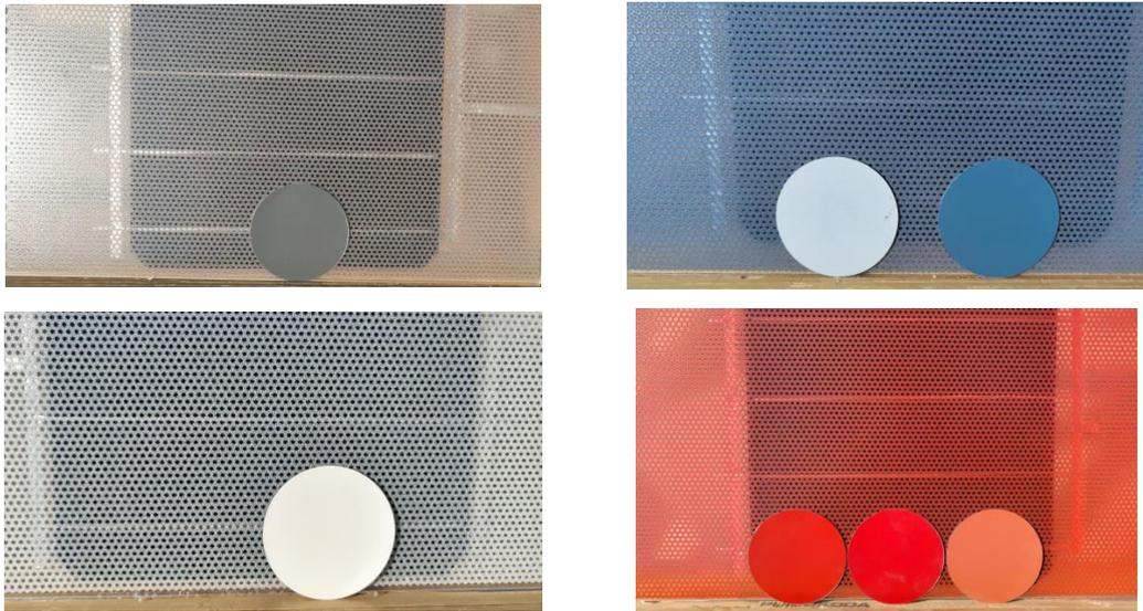
**Figure 27.** Module with digital ceramic printed front glass and coloured metal backsheet RAL code match test
