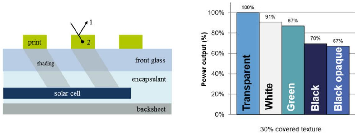
**Figure 16.** Left: Schematic drawing of changes in module optics by application of decorative prints onto the module front cover (M. Mittag et al., 2017). Right: Colour texture effect on power output (%) (P. Bonomo, SUPSI, 2017).
