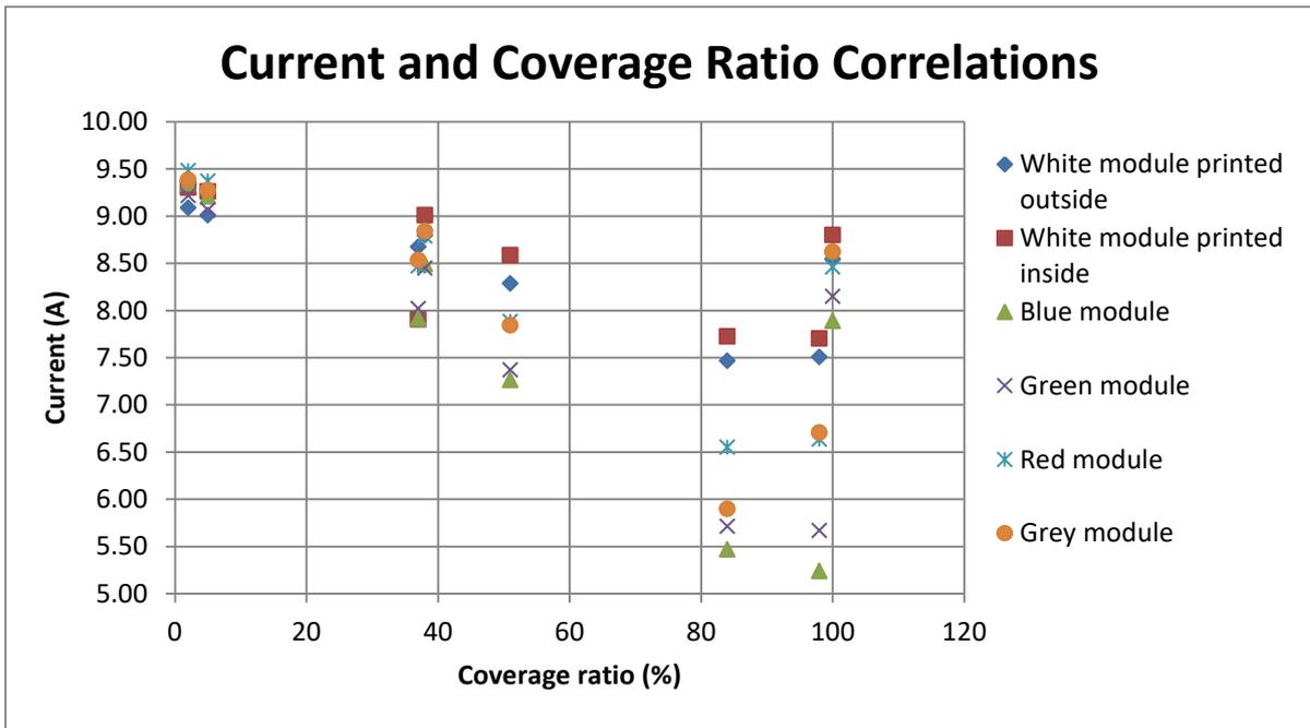
**Figure 31.** Current and coverage ratio correlation for each coloured module with digital ceramic printing front glass.
