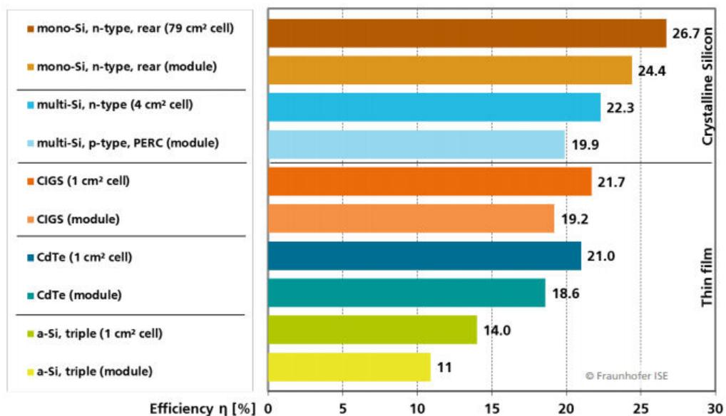
**Figure 4.** PV cell and module efficiencies of different technologies (Source: Fraunhofer Institute for Solar Energy Systems, ISE, 2018).
