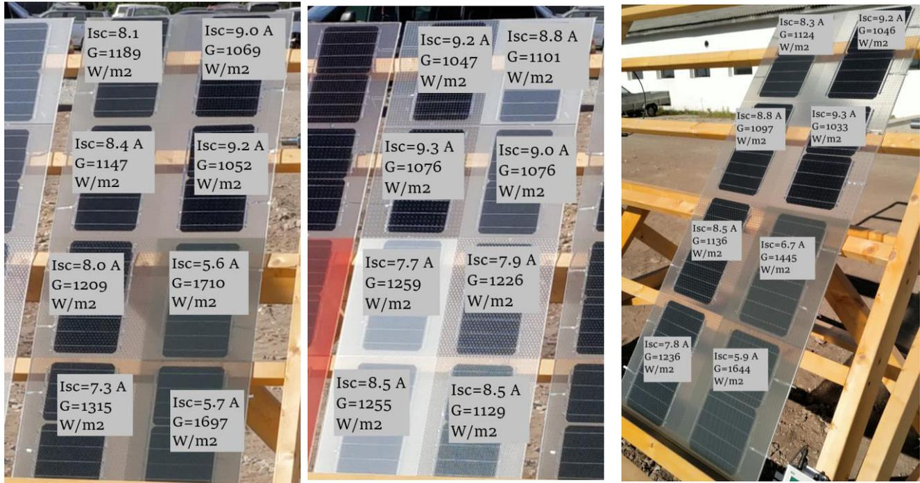
**Figure 30.** Power output assessments for each manufactured module.
