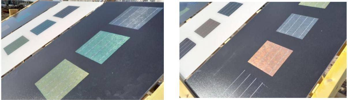
**Figure 21.** Visual changes of coloured multi-crystalline PV cells due to scattering of light, inclination angle of the modules and exposure to sunlight.
