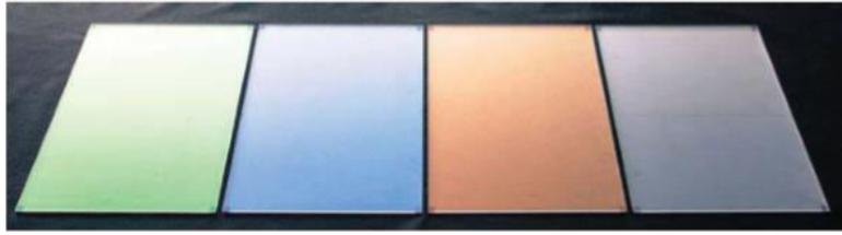
**Figure 11.** Colour coated glass with high transmittance (Source: SwissInso).
