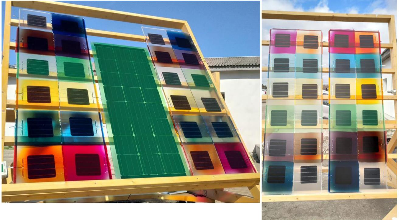
**Figure 24.** Left: Visual differences between laminating active layer of the module by using one layer EVA (on the left) and two layers of EVA foils (on the right) with green EVA encapsulated module. Right: Visual examination due to inclination changes.
