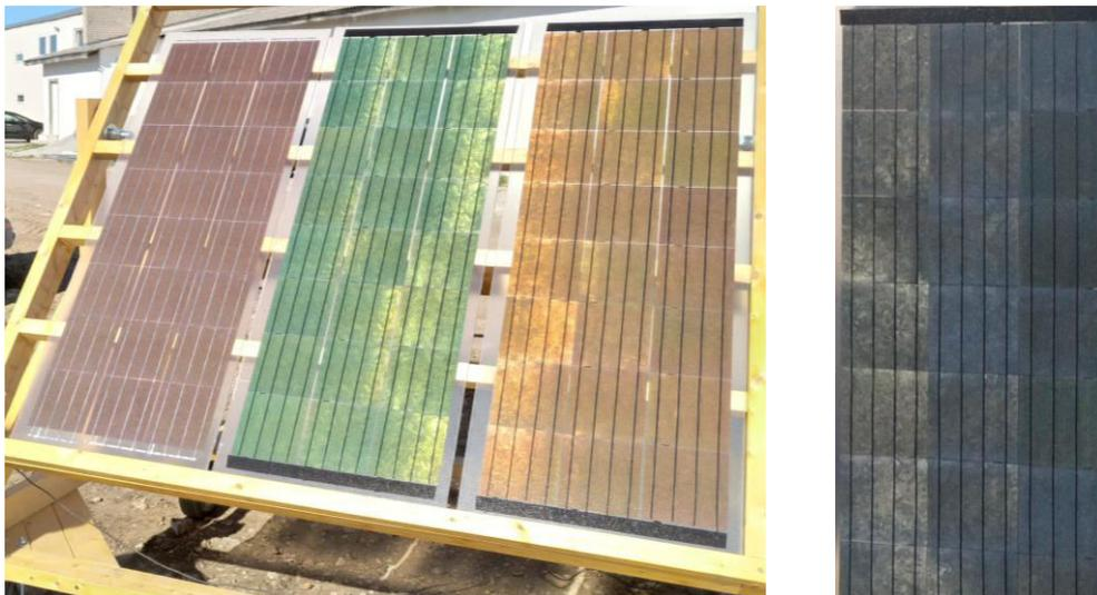
**Figure 22.** Modules with laminated coloured solar cells.
