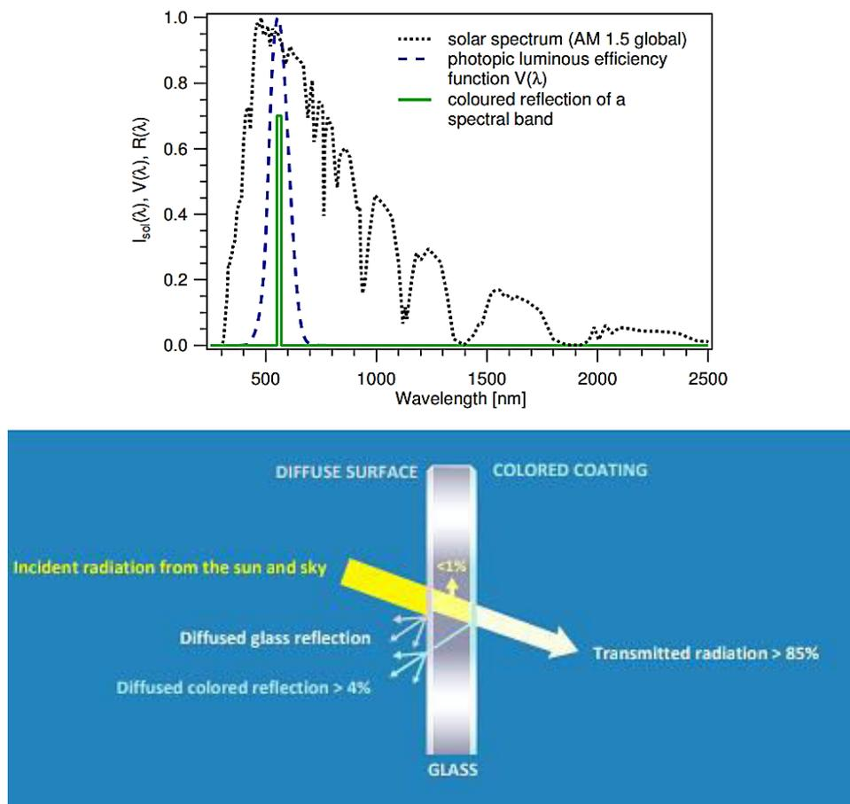
**Figure 10.** Top: Principle of coloured coatings for solar collectors (Mertin, S. (2015)), Bottom: Kromatix™ interference filters principle (Emirates Insolaire LLC).
