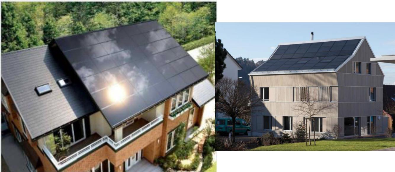
**Figure 6.** Fully covered in-roof installation, Left: (Source: NexPower Technology Corp.) Right: Einfamilienhaus in Glattfelden (Photo: Mirlo Urbano Architekten)
