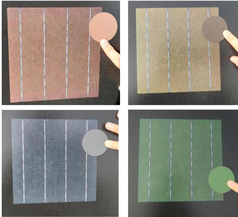
**Figure 20.** Colour matching tests with metal backsheet RAL codes after lamination.
