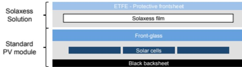
**Figure 28.** Schematic representation for lamination of a special encapsulant foil [55].
