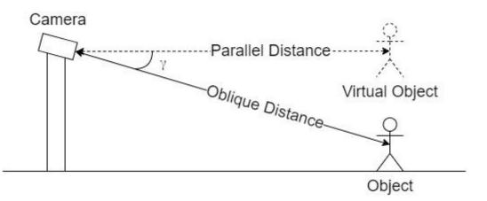
Figure 4. The relationship of the parallel and oblique distances with an inclined camera system.
