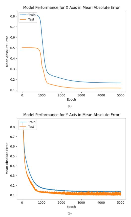
Figure 23. Model performance analysis via mean absolute error for (a) the x-axis estimations and (b) the y-axis estimations.
