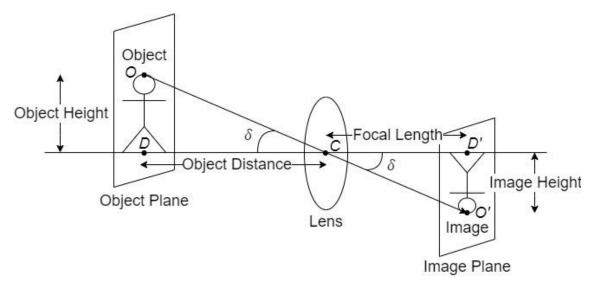
Figure 3. The basic working principle of a camera lens.
