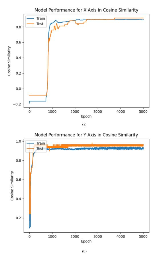
Figure 15. Model performance analysis via cosine similarity for (a) the x-axis estimations and (b) the y-axis estimations.
