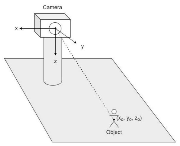
Figure 5. Camera-based coordinate system.
