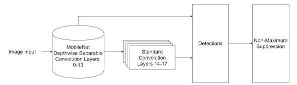
Figure 2. The network architecture of an SSD framework with MobileNet.
