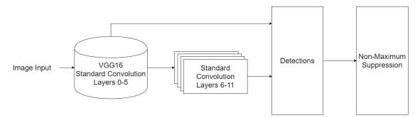
Figure 1. The network architecture of an SSD framework with VGG16.
