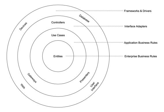
Figure 3. Simplified scheme of Clean Architecture approach
