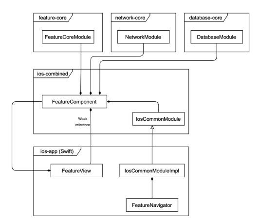
Figure 7. Dependency Injection scheme for iOS
