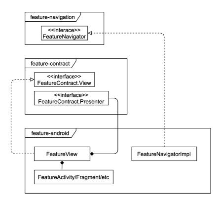
Figure 5. Schematic representation of Android implementation of an abstract feature
