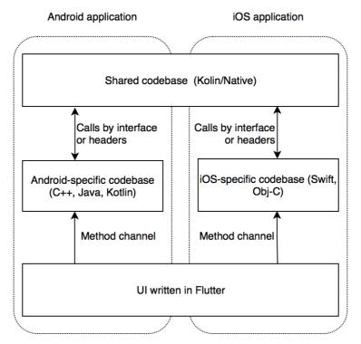
Figure 2. Architecture where both Flutter and Kotlin/Native are used
