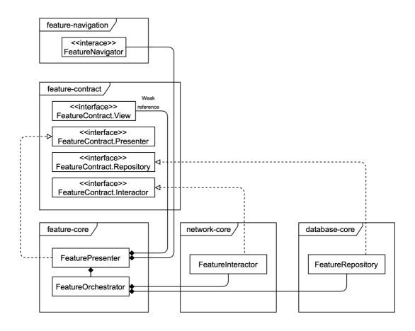
Figure 4. Schematic representation of an abstract feature with some networking and persistence functionality.
