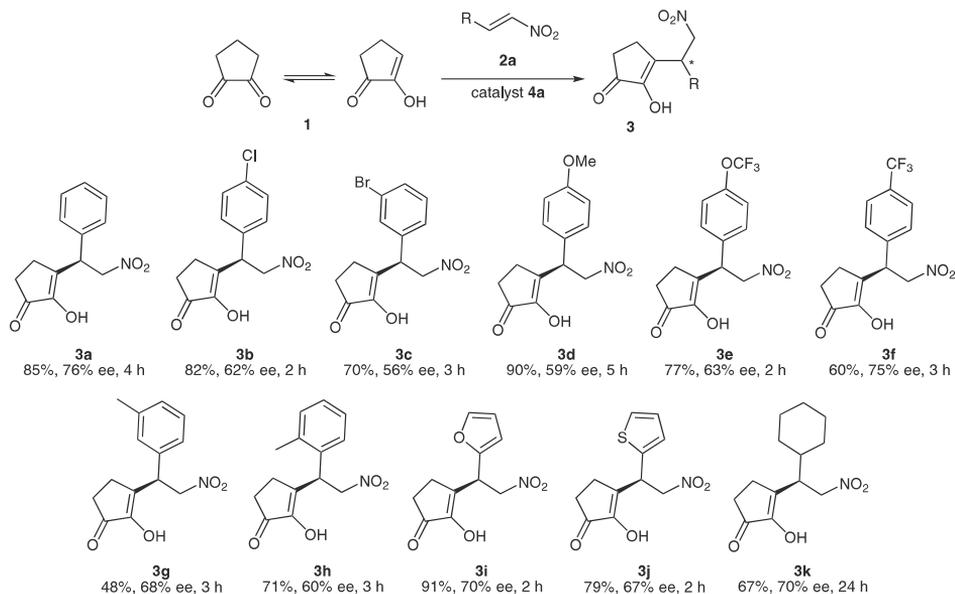
**Scheme 2** Screening of the substrate scope of the Michael addition. *Reagents and conditions:* **1** (0.24 mmol), **2** (0.2 mmol), **4a** (5 mol%),  $\text{CH}_2\text{Cl}_2$  (0.7 mL). Isolated yields are given; ee values were determined by HPLC analysis on a chiral stationary phase.
