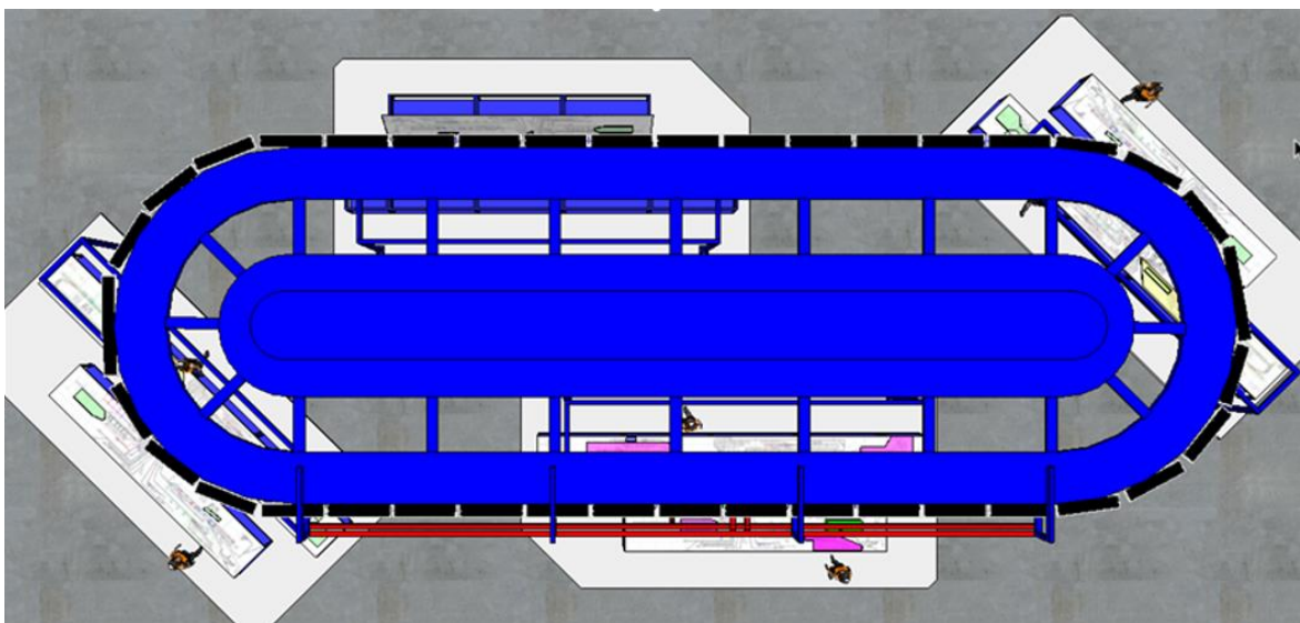
Figure 5.4 SFTP XVK81 chassis harness assembly conveyor top view
