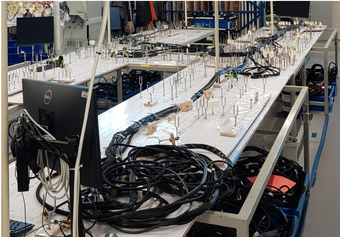
FOT build workstation with product - XVK81 chassis harness for Daimler Actros truck [10]
