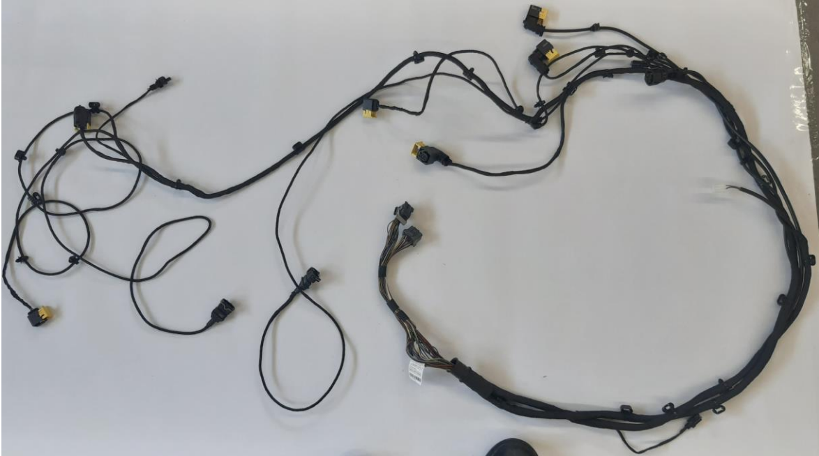
XVK82 front bumper harness for Daimler Actros truck [10]
