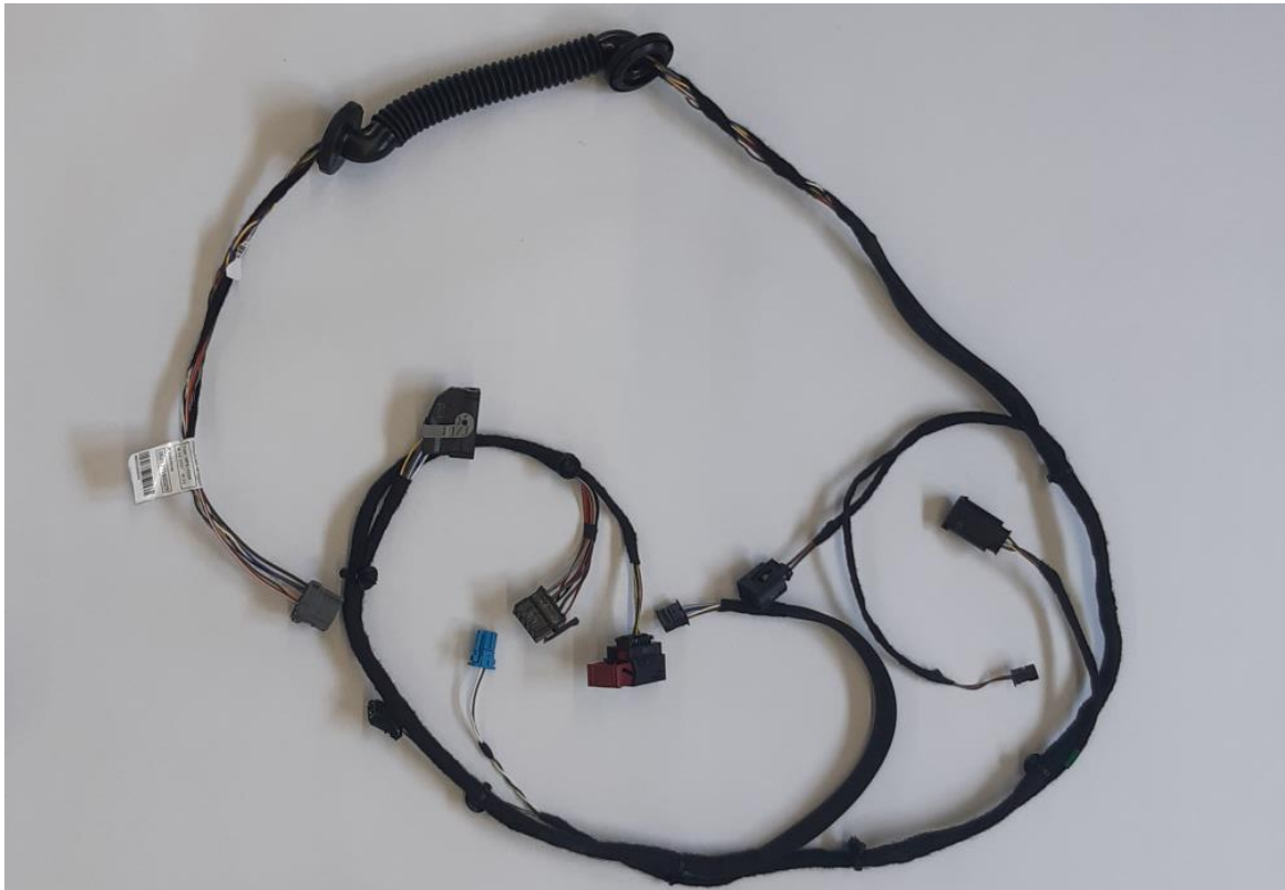
XVK87 door harness for Daimler Actros truck [10]
