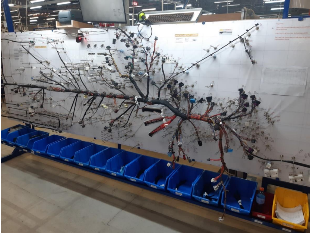
FOT build workstation with product - XVK84 dashboard harness [10]
