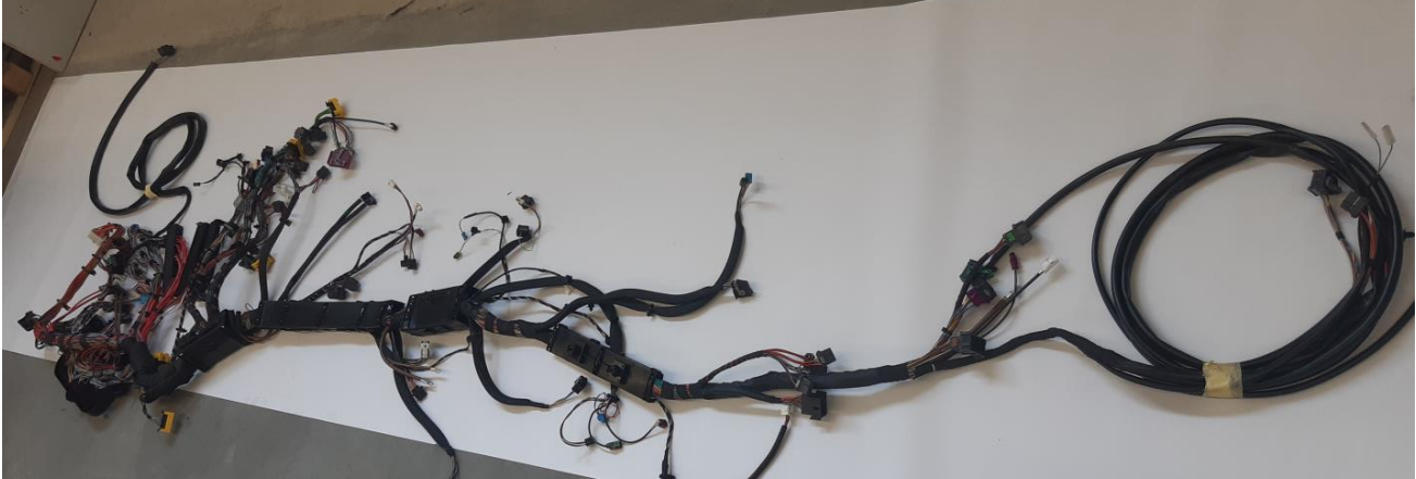
XVK84 dashboard harness for Daimler Actros truck [10]
