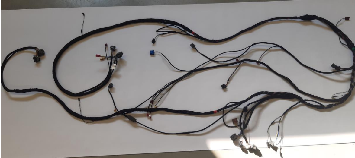
XVK86 roof harness for Daimler Actros truck [10]
