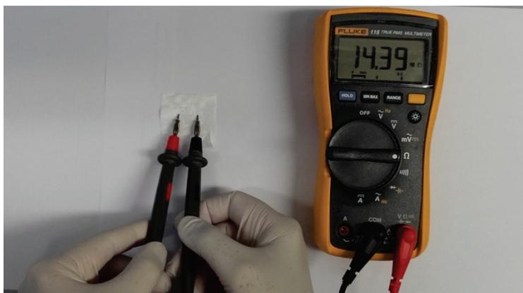
*Figure 3. Experimental validation of the conductivity using a lab scale method (prior to adding GO).*
