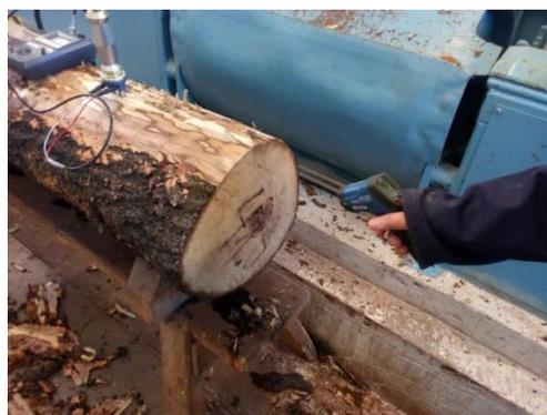
Figure 3.2. 2 Moisture Content and Temperature Measurement
