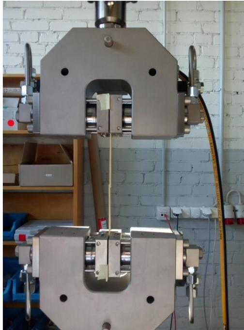
Figure 3.5.3. 1 Bonding quality test specimen and Zwick/Roell Z050 machine
