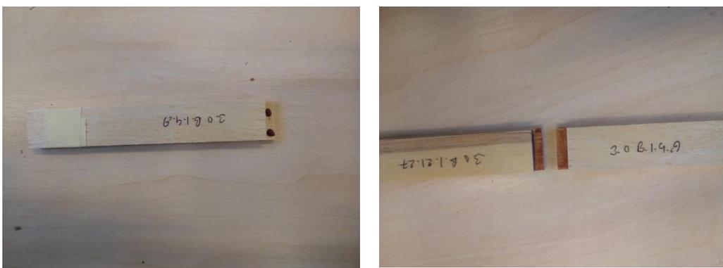
Figure 3.5.2. 1 Adhesive drops and Uniform distribution of Adhesive
