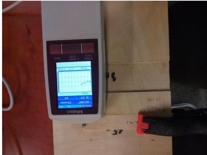
Figure 3.4. 2 Surface roughness measurement procedure
