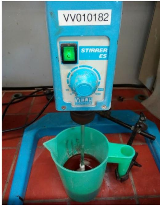
Figure 3.5.1. 1 Mixing of adhesive
