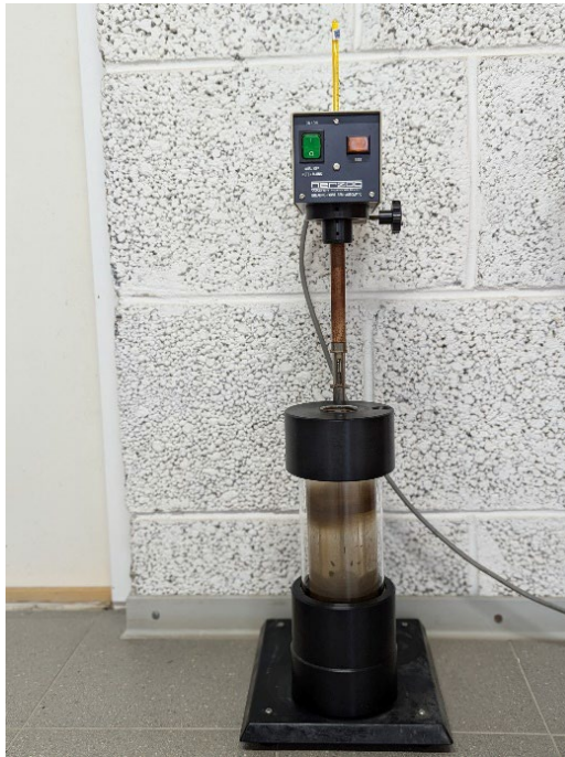
Figure 13. Semi-automatic Fraass apparatus used in this study [Road Technology Centre]
