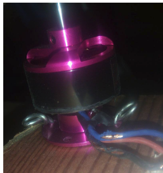
FIGURE 4.2: Broken wires due to grub screw failure.
