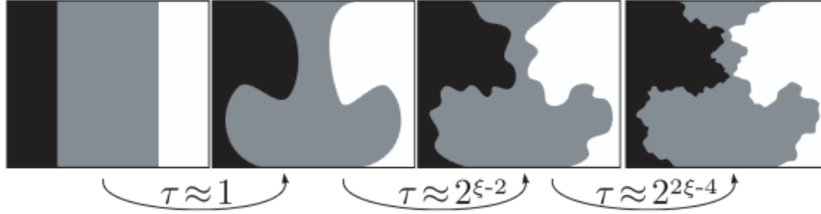
Figure 1. Simplified scheme of the formation of tracer discontinuities, reproduced from [1]. The characteristic time of eddies of size a scales as \tau \approx a^{2-\xi} . Due to the combined effect of large and small eddies, low- and high-density regions are brought into contact within a finite time.
