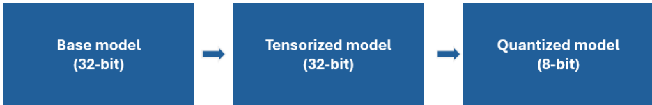
Figure 3: An illustration of the trainable pipeline for model compression using the ensemble of Tensor Train Decomposition (TTD) and 8-bit quantization. The pipeline begins with a trained base model, followed by TTD applied to dense layers, and concludes with 8-bit quantization of the resulting tensor trained model. Appendix 2, Figure 3
