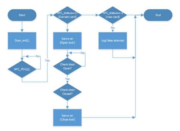
Figure 11 Software logic diagram
