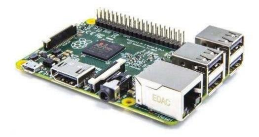
Figure 5 Single-board computer Raspberry PI [25]
