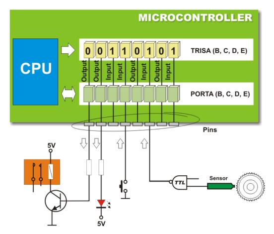
Figure 2 Example of microcontroller I/O [23]
