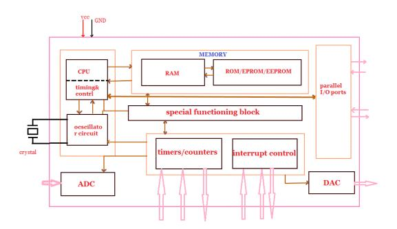
Figure 1 Structure of a microcontroller [6]
