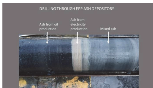
Figure 1. Drill core from ash disposal site at the Eesti Power Plant, north-eastern Estonia.
