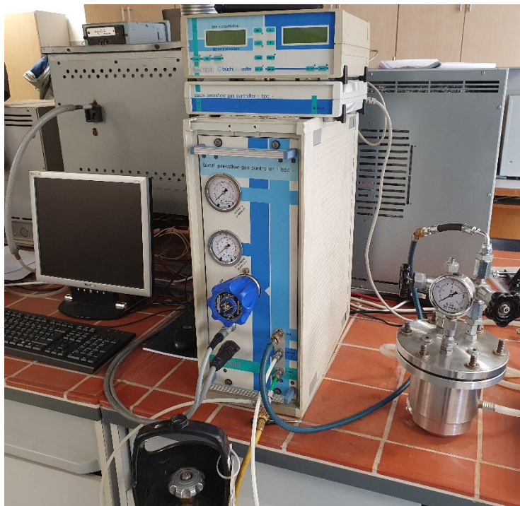
Figure 4 Experimental setup comprising gas monitoring device, computer, CO 2 gas cylinder and climate-regulated autoclave.
