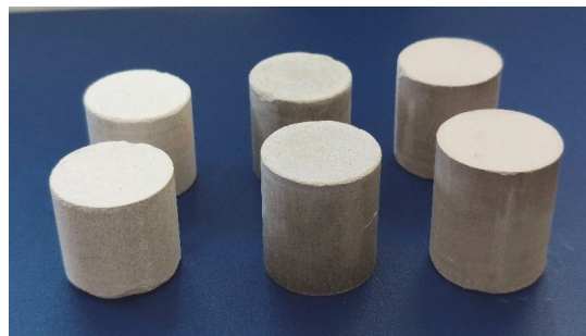
Figure 3. Prepared cylindrical compacts of LFA (left), WA (middle), and OSA (right).
