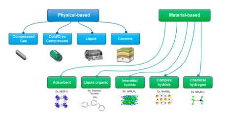
Fig. 19 Hydrogen storage technologies [35]
