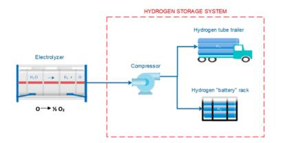
Fig. 21 Hydrogen storage system [35]
