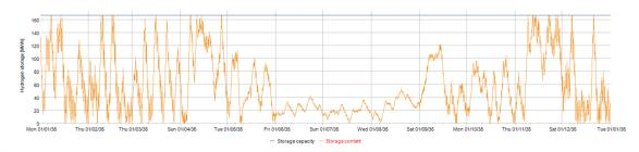
Fig. 39 Concept 1 - storage if H2 is 120 MJ/kg, storage capacity 175 MWh
