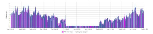
Fig. 38 Concept 1- PEM electrolyser production and hydrogen demand
