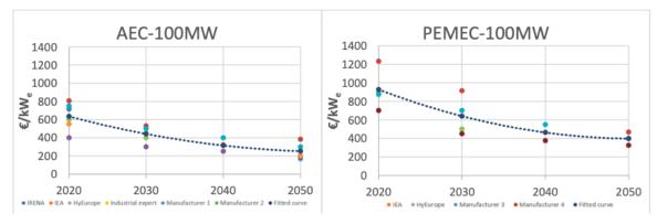
Fig. 18 CAPEX values: 100 MW AEC and PEMEC [33]
