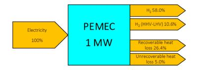
Fig. 15 PEMEC energy balance
