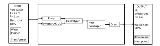
Fig. 16 Systems of AEC and PEM electrolysers [33]
