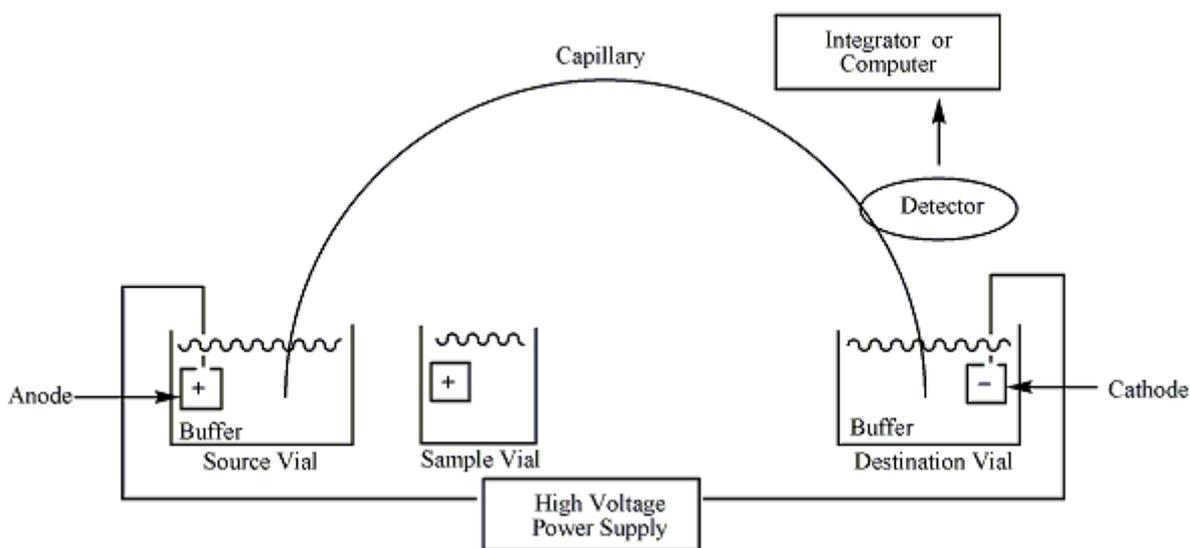
Figure 4. Diagram of a basic capillary electrophoresis system [21]
