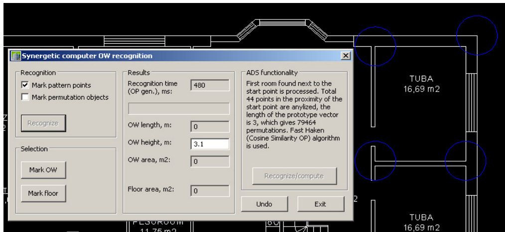
Fig. 4 AutoCAD graphics screen – “Mark pattern points” option selected
