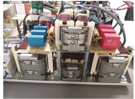
Fig. 9. NZEB EMS grid and load-side LCL filters.
