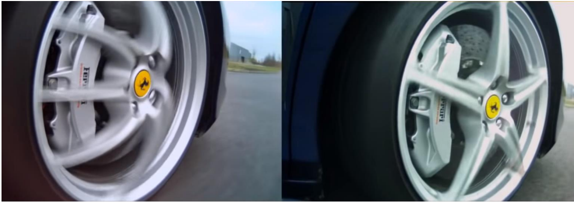
Figure 7. Comparison of rolling and global shutter [12].
