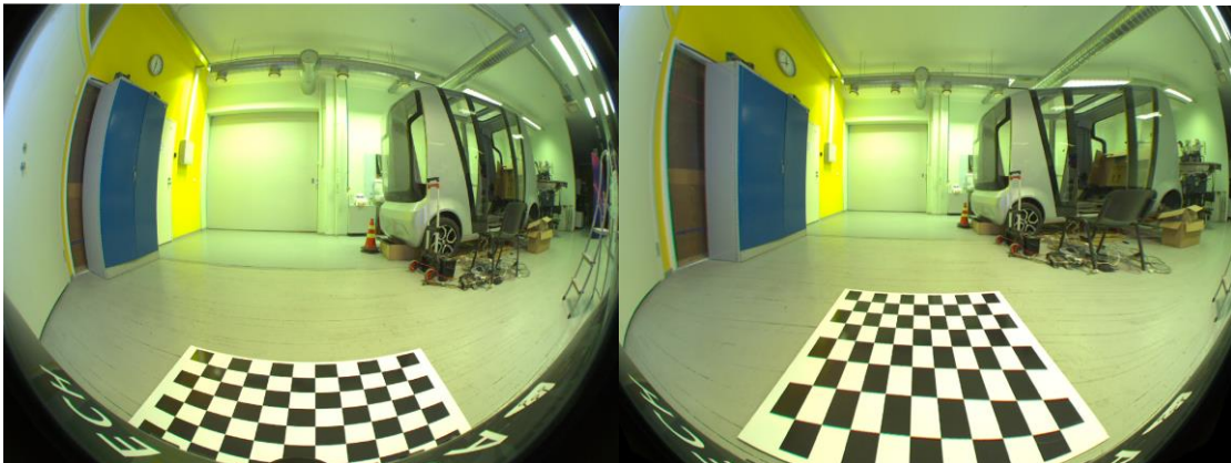
Figure 16. Before and after calibration. Lines that should be straight are straight now.
