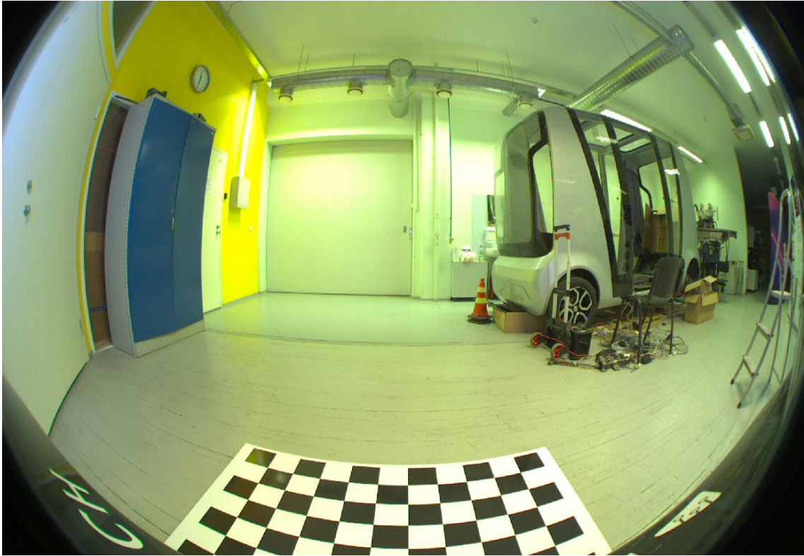
Figure 14. Distorted image from the camera. Notice the curved lines that should be straight.
