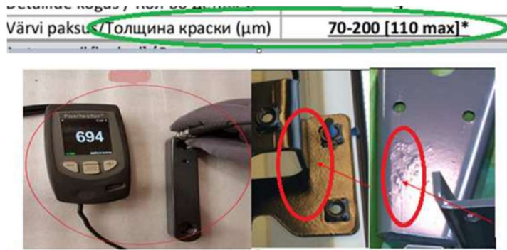
Figure 3.23: Large number of thickness due to wrong speed on the powder line
