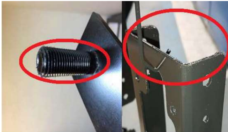
Figure 3.5: Sharp edges on undemagnetized surfaces after ED coating
