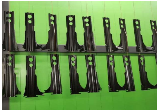
Figure 3.6: Example of heavy parts hanging method for powder line
