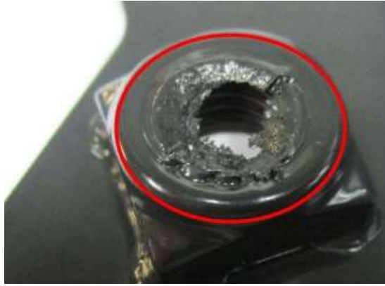
Figure 3.19: Defect caused by dirty mask
