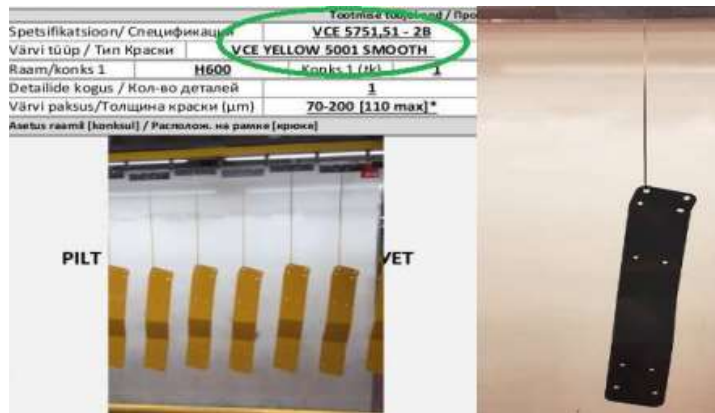
Figure 3.24: Wrong type of colour was used for the powder coating
