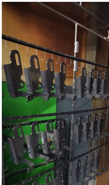
Figure 3.8: Example of light parts hanging method for the powder line
