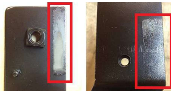
Figure 3.25: Inadequate distance between parts on the ED coating line
