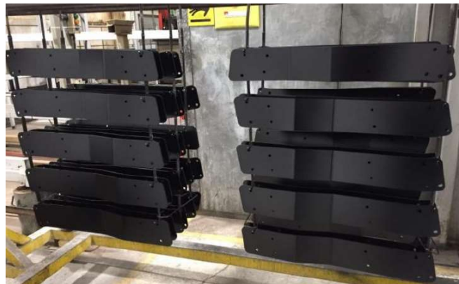
Figure 3.7: Example of heavy parts hanging method for the ED coating line
