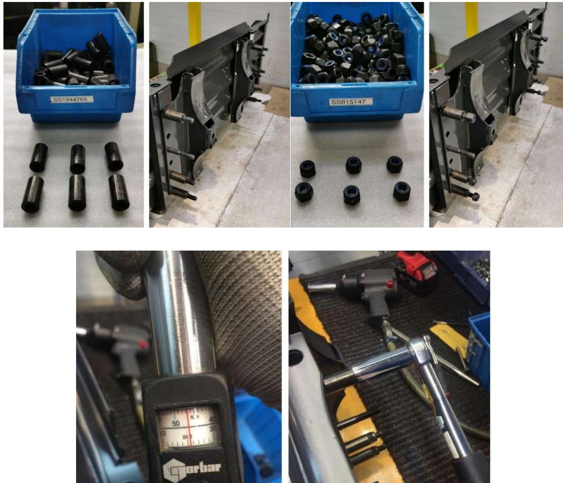
Figure 3.17: Assembly process for the Scania battery box
