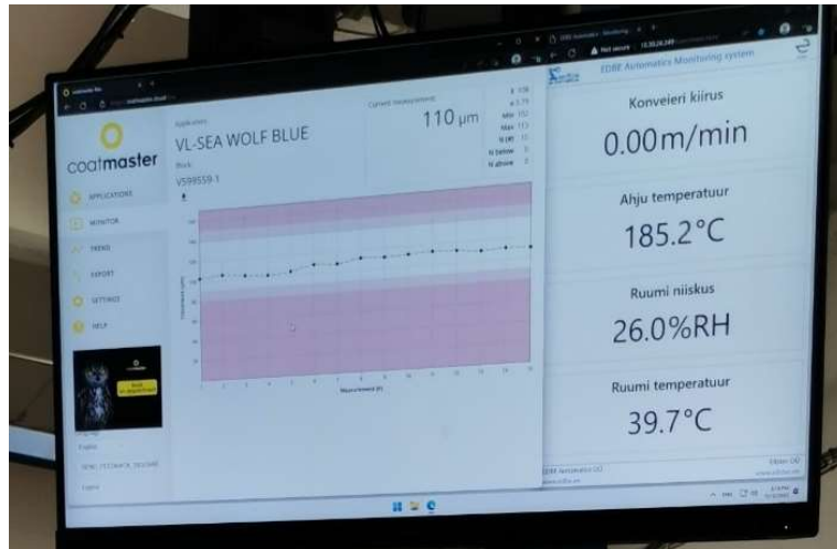
Figure 4.6: Powder coating monitoring with all needed information for the painters
