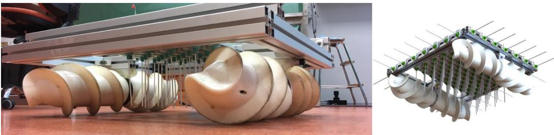
Figure 1. Robominer test platform with drive screw actuators and whisker sensor array attached. Left figure shows a small-scale prototype. Right figure shows a CAD assembly of the prototype.
