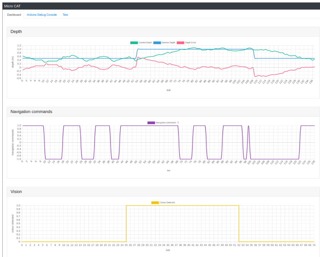
Figure 17. Dashboard visualizing the depth data, navigation commands and vision data of \mu -CAT v2 in simulation.
