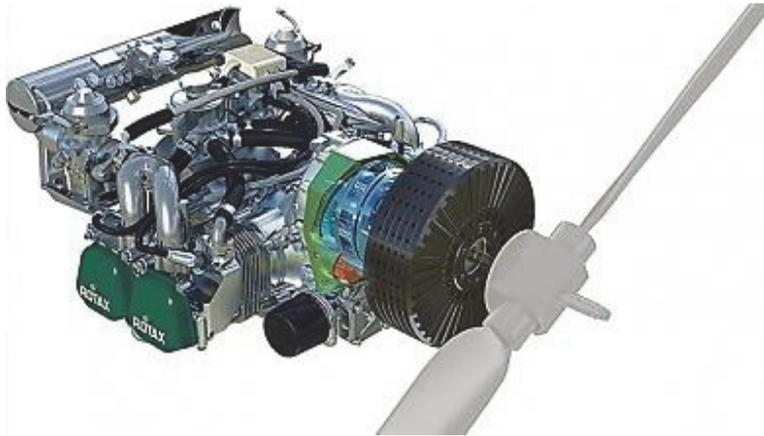
*Fig. 1.8. A hybrid-electric drive prototype by Rotax Aircraft Engines [22].*
