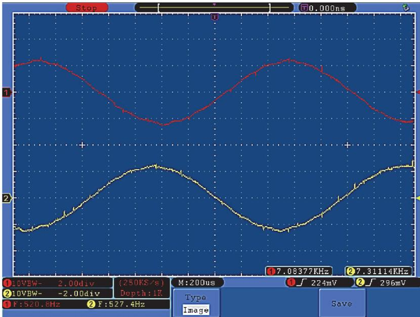
Fig. 5.8. Waveform of the FESM phase voltage  $U_{ph}$  at  $n = 1500$  rpm.
