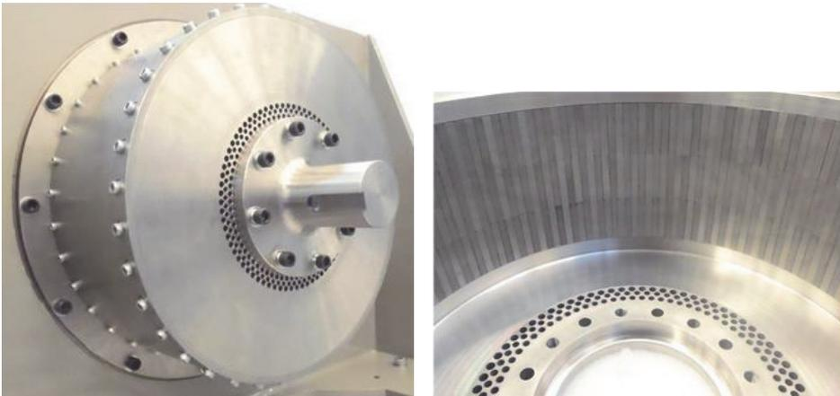
*Fig. 1.4. High torque density PMSM developed by PEMC [18].*
