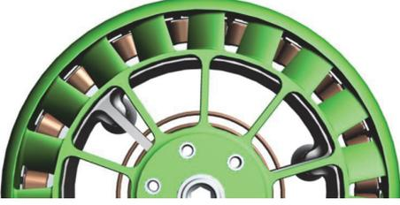
Fig. 2. The air cooling system with an impeller on the rotor.
