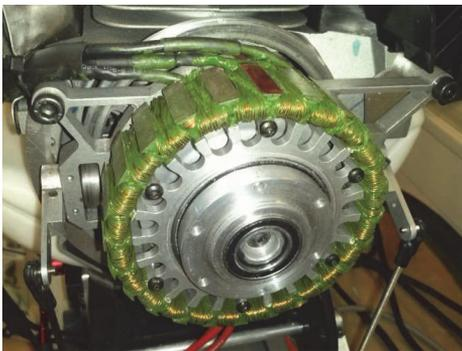
Fig. 3. View of the wound stator.
