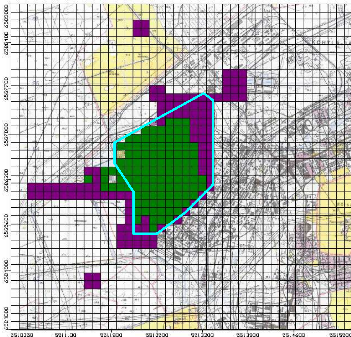
Fig.3.5.1.17. Constant Concentration boundary condition in the 1 st layer (Quaternary deposits) of the Kohtla-Järve phenols transport model. Sum of phenols, mg/L: violet – 1.0, green – 20.0, light grey – 400.0, light olive – 500.0, light violet – 1000. Other graphical symbols – see the Fig. 3.5.1.1, and 3.5.1.2.
