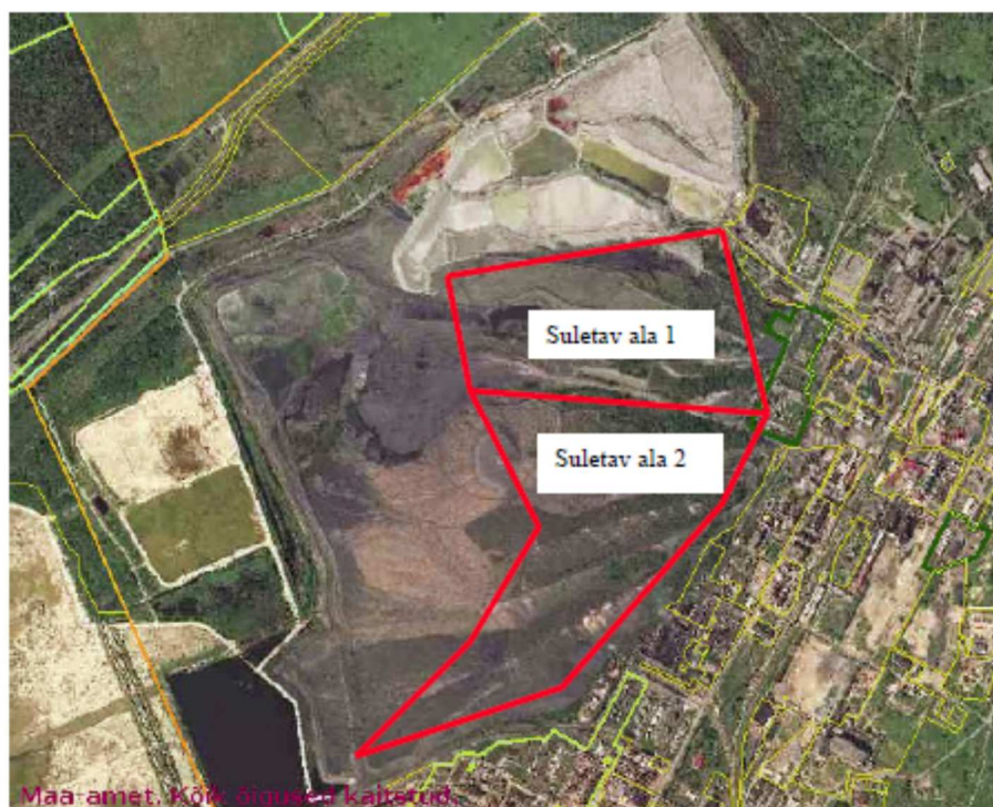
Fig. 4.1.1. Orthophoto of the Kohtla-Järve landfill (the area of the ash landfill is light grey). The portion of the landfill determined for closing up (92 ha) has been surrounded by a red contour in the figure (Tööstusjäätmete ja...2007).
