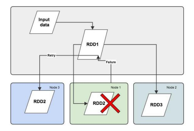
Figure 3. RDD recovery via lineage data.
