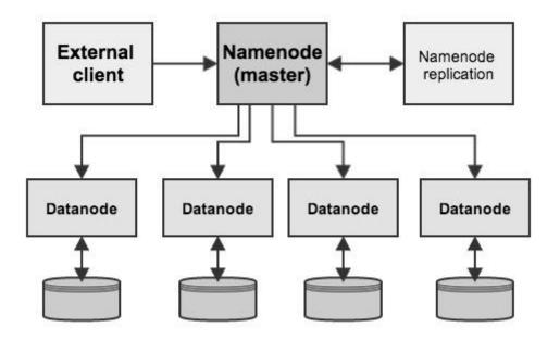
Figure 1. Master node and data nodes.
