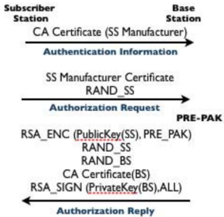
Figure 7: WiMax PKMv2 message flow for authentication [5]
