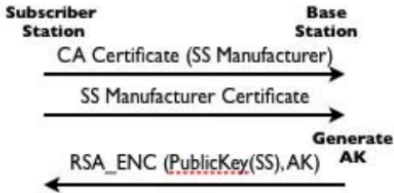
Figure 6: WiMax PKMv1 message flow for authentication [5]
