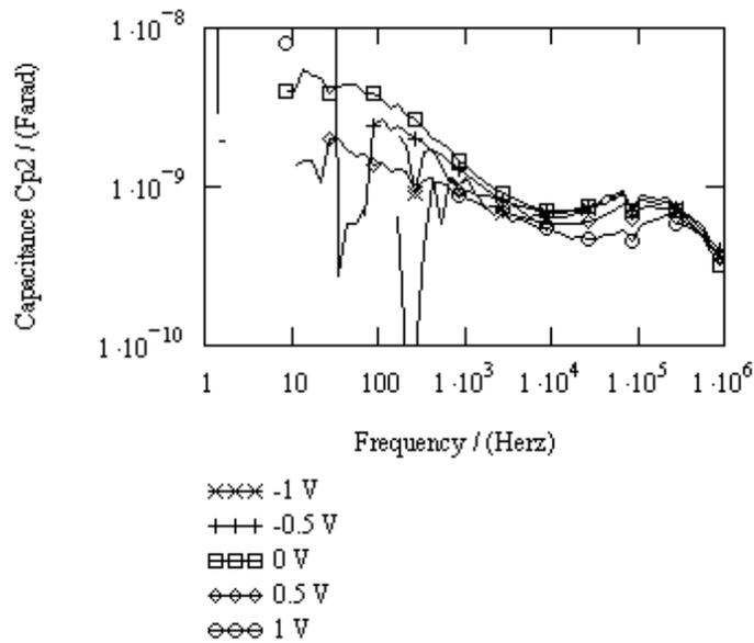
**Fig. 3.2.5c.** Results of the circuit calculation there impedances of two similar (difference is a half of the decade) frequencies were used for circuit evaluation ( $C_{p2}$  vs. frequency)
