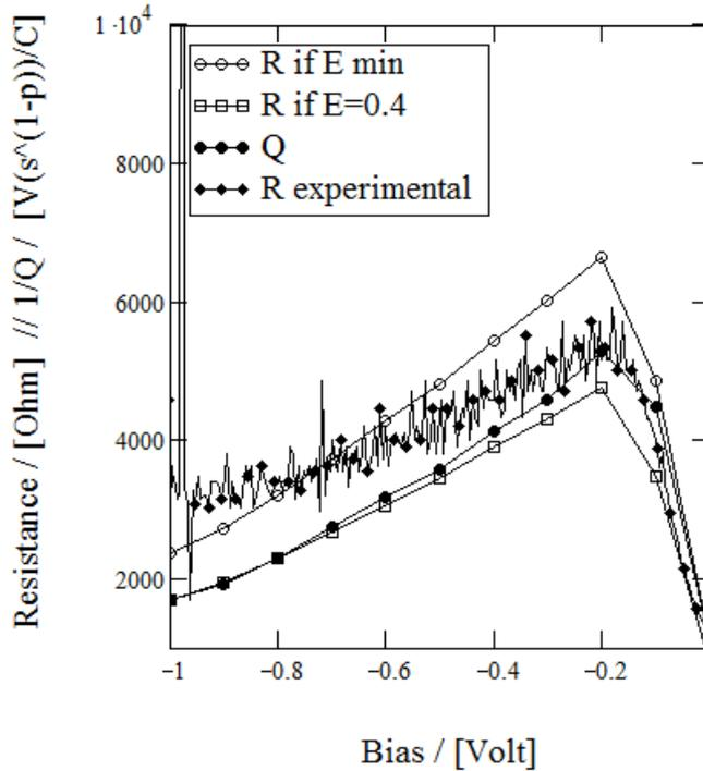
Fig. 3.5.5.3. Comparison of  $I$ - $V$  measurement (reverse bias) based differential resistance with the resistance predicted from Eq. 1.7.1.6 and Eq. 1.7.1.7, and the  $Q$  of the resistance-like CPE (measurement frequency 200 Hz)
