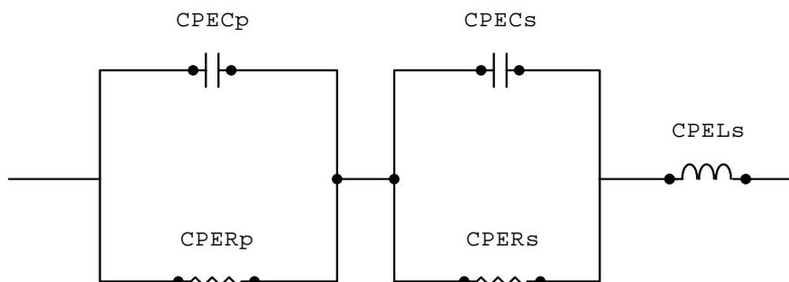
**Fig. 3.4.3. Equivalent circuit found to describe the impedance behavior of the glass/ITO/CISE/graphite structure. CPE notation in names of circuit elements of CPECp, CPERp, CPECs, CPERs and CPELs points to the circumstance that these elements are CPE elements resembling either capacitors, resistors or inductors**
