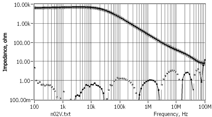
**Fig. 3.5.2.3. Modeling of the impedance amplitude response of the glass/ITO/CISE/graphite structure: -0.2 V (square dots correspond to the experimental result, solid line corresponds to the fit, line with the smoother filled dots report the error percentage)**
