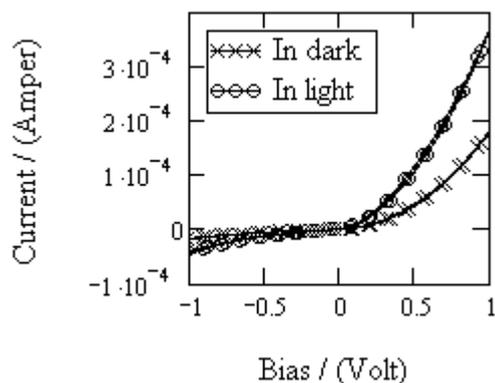
**Fig. 3.2.1.**  $I$ - $V$  curves of glass/ITO/PLD- $\text{CuIn}_3\text{Se}_5$ /ZnPc in dark and light conditions (the contacting area is  $2 \text{ mm}^2$ )
