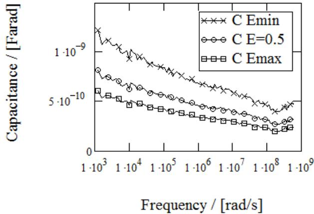
**Fig. 3.5.3.1. Capacitance calculated according to two limiting conditions of  $E$  ( $E_{\min}$  and  $E_{\max}$ ) and at  $E=0.5$  (curve of  $E_{\max}$  corresponds to the situation, then  $E=1$ , curve of  $E_{\min}$  is then Eq. 1.6.14c is used, reverse bias  $-0.2$  V)**
