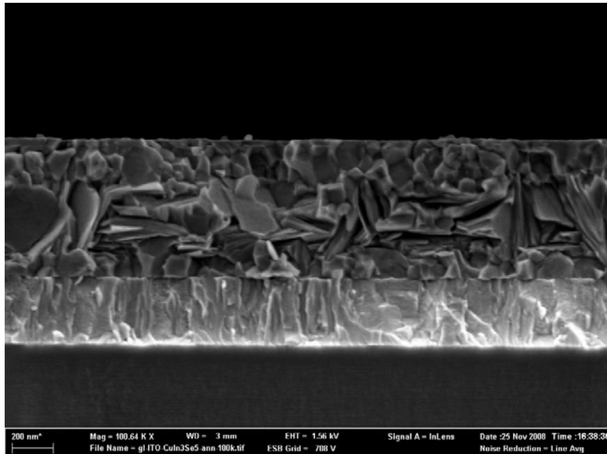
**Fig. 3.3.2.** SEM micrograph of the ITO/ HfV  $\text{CuIn}_3\text{Se}_5$  annealed at  $450^\circ\text{C}$  for 1 hour in argon atmosphere
