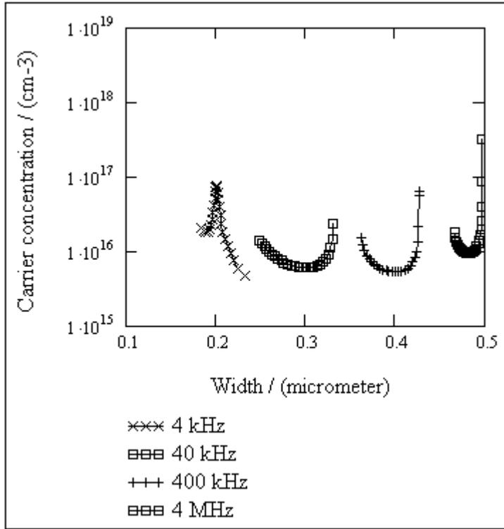
**Fig. 3.5.7.3a. Carrier concentration profiles of the glass/ITO/CuIn<sub>3</sub>Se<sub>5</sub>/graphite structure calculated at forward biases and at different frequencies of the ac signal**
