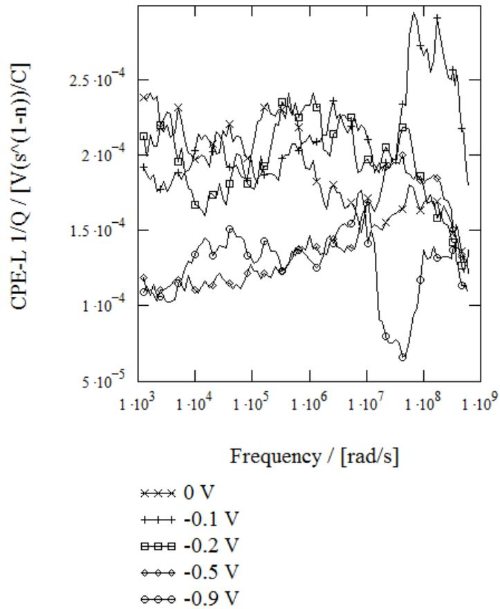
**Fig. A1.9.** Equivalent circuit (Fig. 3.4.3 in main text) element CPE-Ls parameter  $1/Q$  frequency dependence on different applied reverse biases
