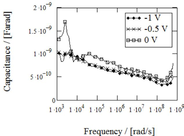
**Fig. 3.5.7.1. Frequency dependences of the depletion layer capacitance at different reverse biases**
