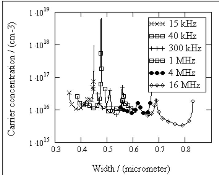
**Fig. 3.5.7.3. Carrier concentration profiles of the glass/ITO/CuIn<sub>3</sub>Se<sub>5</sub>/graphite structure calculated at reverse biases and at different frequencies of the ac signal**
