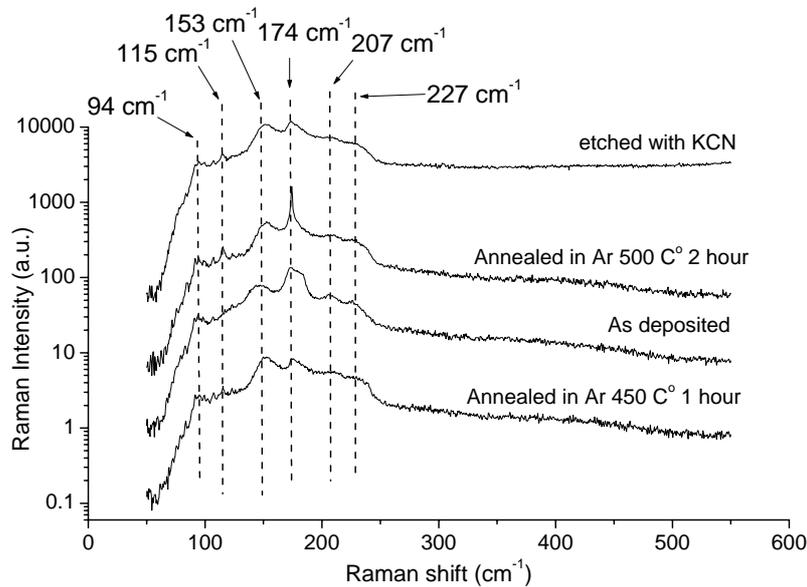
**Fig. 3.3.5. Raman spectra of glass/ HVE  $\text{CuIn}_3\text{Se}_5$  structures**
