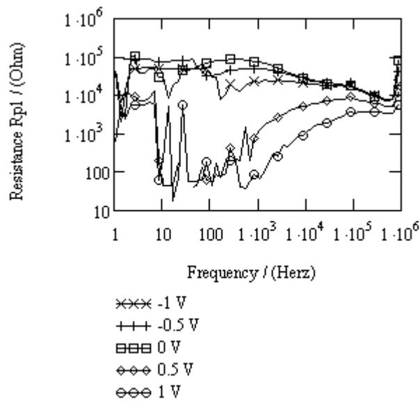
**Fig. 3.2.5b.** Results of the circuit calculation there impedances of two similar (difference is a half of the decade) frequencies were used for circuit evaluation ( $R_{p1}$  vs. frequency)
