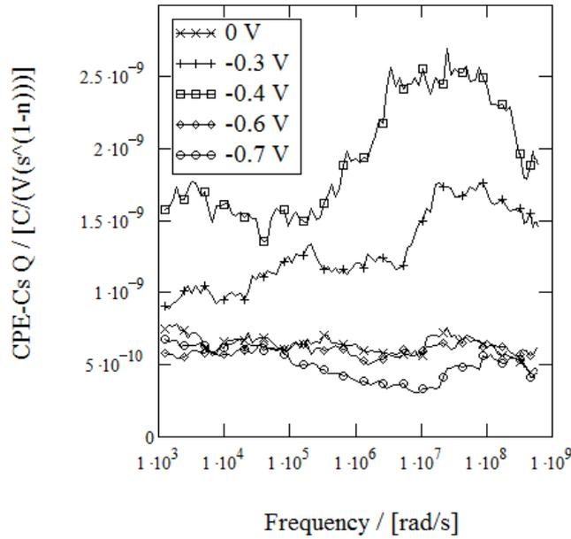
Fig. A1.7. Equivalent circuit (Fig. 3.4.3 in main text) element CPE-Cs parameter  $Q$  frequency dependence on different applied reverse biases
