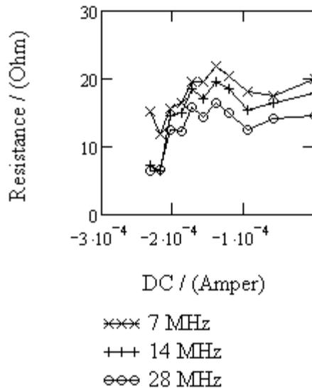
**Fig. 3.5.8.1. Differential series resistance dependences on reverse dc at different frequencies**
