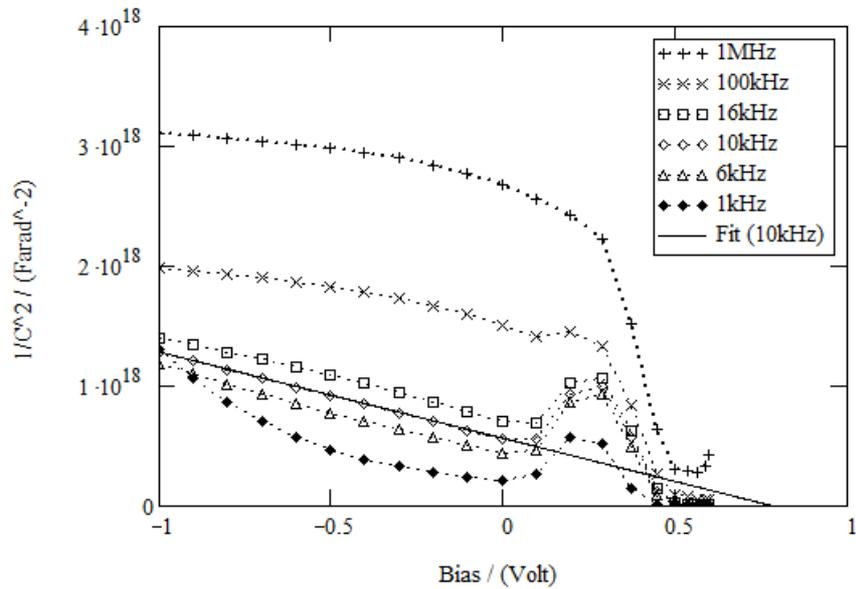
**Fig. 3.4.8. Mott-Schottky curves of the glass/ITO/CuIn<sub>3</sub>Se<sub>5</sub> annealed at 450°C for 1 hour**
