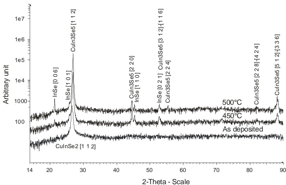
**Fig. 3.3.4. XRD spectra of glass/ HVE  $\text{CuIn}_3\text{Se}_5$  structures**
