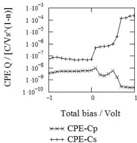
Fig. 3.4.5. Dependence of the  $Q$  of the CPE-Cp and CPE-Cs on total bias applied on structure of glass/ITO/CuIn<sub>3</sub>Se<sub>5</sub> annealed at 450°C for 1 hour with following deposition of the graphite dot-contacts
