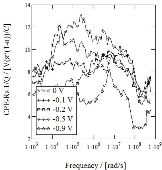
**Fig. A1.5.** Equivalent circuit (Fig. 3.4.3 in main text) element CPE-Rs parameter  $1/Q$  frequency dependence on different applied reverse biases
