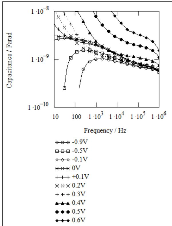
**Fig. 3.4.7. Parallel differential capacitance vs. frequency dependencies of the glass/ITO/CuIn<sub>3</sub>Se<sub>5</sub>/graphite structures annealed at 450°C for 1 hour, measured at different applied potentials (reverse biases marked with transparent margins, forward with crosses and filled margins)**
