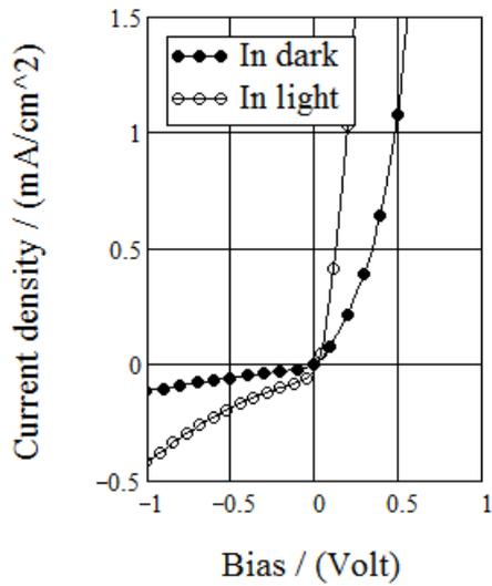
**Fig. 3.3.7.**  $I$ - $V$  curves of the aged glass/ITO/HVE  $\text{CuIn}_3\text{Se}_5$ /graphite structures annealed at  $450^\circ\text{C}$
