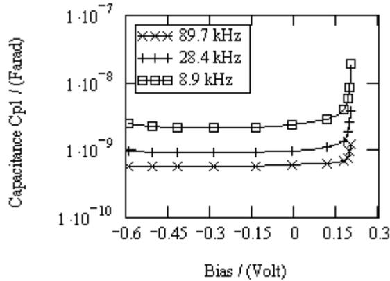
**Fig. 3.2.8.** *C-V* curves constructed according to the bias distribution calculations of Eq. 3.2.1
