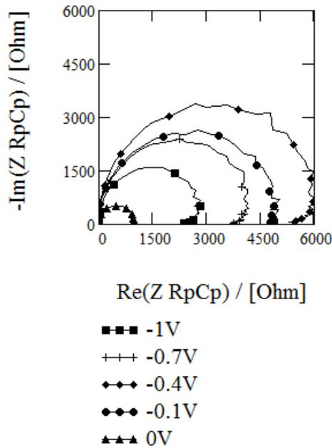
**Fig. 3.5.6.3. Nyquist plots of the impedance of the resistance and capacitance in parallel calculated according to the transformation schematically reported on Fig. 3.5.6.1**
