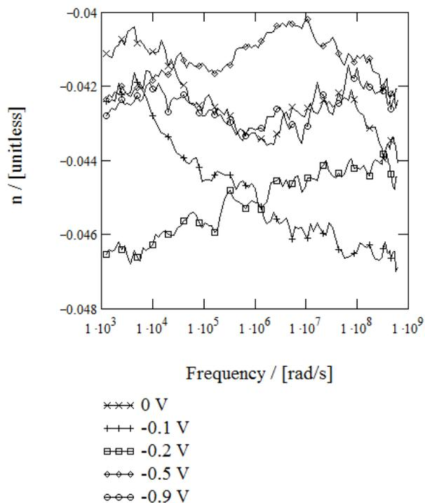
**Fig. A1.6.** Equivalent circuit (Fig. 3.4.3 in main text) element CPE-Rs parameter  $n$  frequency dependence on different applied reverse biases
