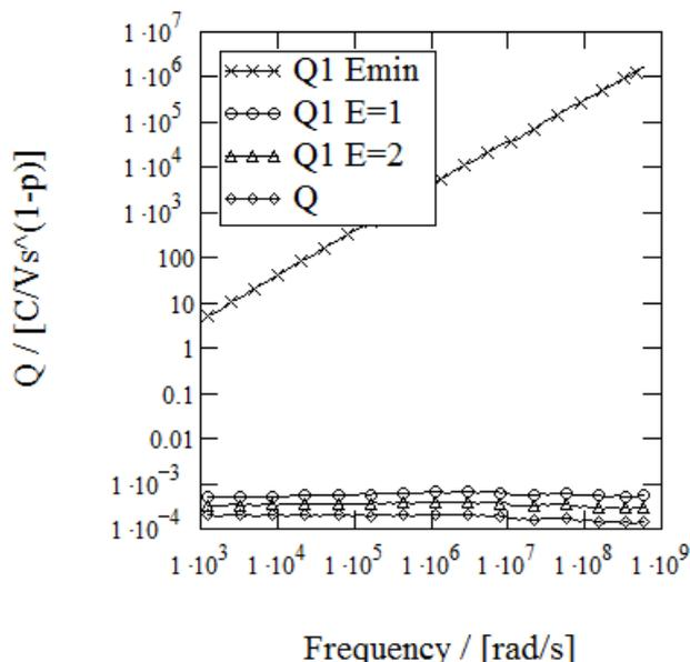
**Fig. 3.5.4.3.**  $Q_I$  of modula CPE calculated in case of different values of proportionality factor  $E$  (curve of  $E_{\min}$  corresponds to the situation, then  $E$  is calculated according to Eq. 1.7.1.8a, reverse bias -0.2 V)
