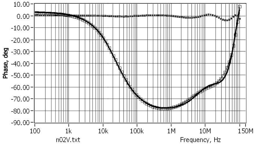
**Fig. 3.5.2.4. Modeling of the impedance phase response of the glass/ITO/CISE/graphite structure: -0.2 V (empty square dots correspond to the experimental results, solid line corresponds to the fit, line with the smoother filled dots reports the error percentage)**
