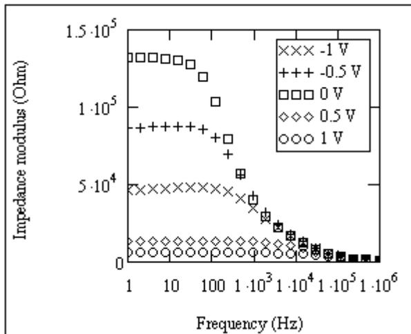
**Fig. 3.2.3.** Dependence of the impedance modulus on ac frequency in case of the structure of glass/ITO/PLD-CISE/ZnPc
