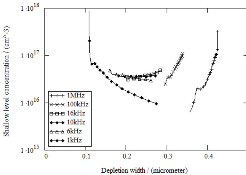
**Fig. 3.4.9. Free charge carriers profiles for the glass/ITO/CuIn<sub>3</sub>Se<sub>3</sub> annealed at 450°C for 1 hour, calculated at different measurement frequencies**
