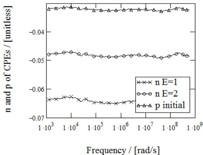
Fig. 3.5.4.2. Exponential parameters ( $n$ ) of the modula CPE calculated according different values of  $E$  and compared with the curve of initial CPE exponential parameter ( $p$ ) (reverse bias -0.2 V)
