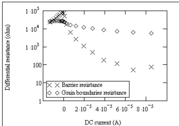
**Fig. 3.2.6.** A dependency of parallel resistances of  $R_{p1}$  and  $R_{p2}$  on dc current if the frequency is 1 kHz
