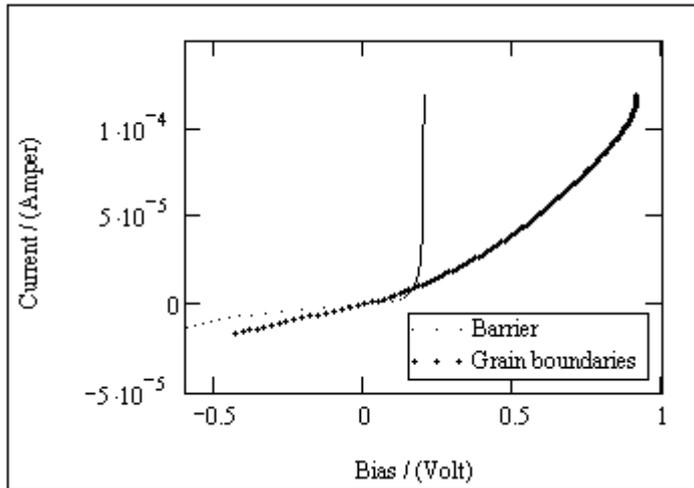
**Fig. 3.2.7.** A bias distribution calculated according to the Eq. 3.2.1 distinguishing two separate regions in the structure of glass/ITO/PLD-CuIn<sub>3</sub>Se<sub>5</sub>/ZnPc
