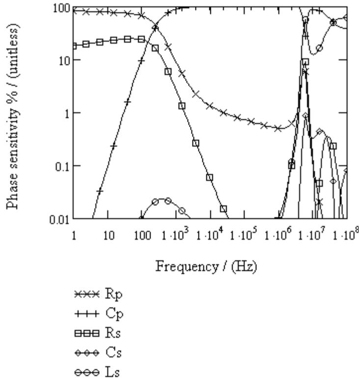
**Fig. 3.5.2.6a. Sensitivity analysis of the impedance phase according to the formula of the circuit represented on the Fig. 3.5.2.1 (forward bias 0.1 V)**
