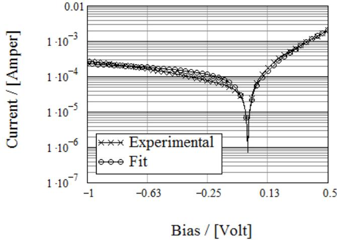
**Fig. 3.5.5.1.**  $I$ - $V$  curve of the structure of glass/ITO/CuIn<sub>3</sub>Se<sub>5</sub>/graphite measured in dark conditions (contact area 2 mm<sup>2</sup>)
