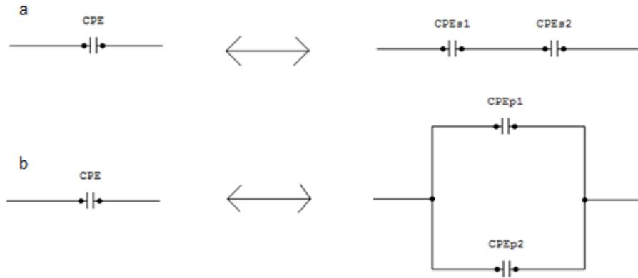
**Fig. 1.6.1. Transformation of the CPE impedance or admittance into series (a) or parallel (b) configuration of two CPE-s (This transformation is invariant and reversible if the exponential parameters of the two new CPE-s can be fixed)**
