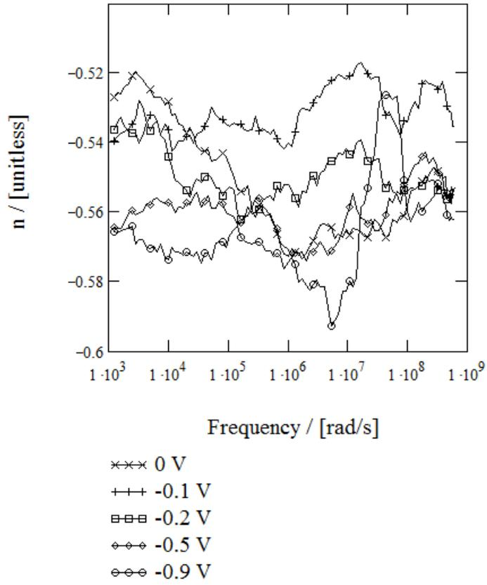
**Fig. A1.10.** Equivalent circuit (Fig. 3.4.3 in main text) element CPE-Ls parameter  $n$  frequency dependence on different applied reverse biases
