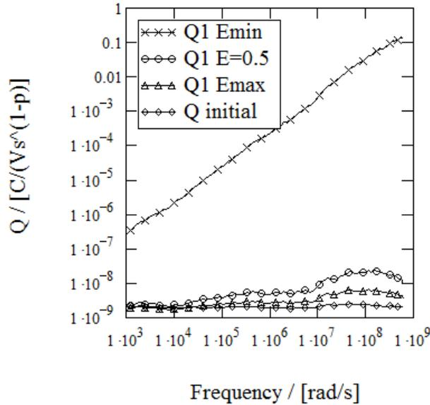
**Fig. 3.5.3.3.**  $Q_I$  of CPE calculated according to two limiting conditions and compared with the  $Q_I$  values of the condition with an arbitrary  $E=0.5$  and with the curve of  $Q$  of initial CPE (curve of  $E_{\max}$  corresponds to the situation, then  $E=1$ , curve of  $E_{\min}$  is then Eq. 1.6.14c is used, reverse bias  $-0.2$  V)
