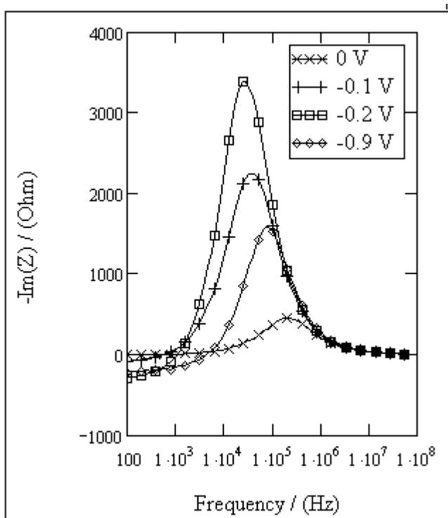
**Fig. 3.5.1.2. Structure of glass/ITO/CISE/graphite impedance imaginary part dependence on measuring signal frequency at zero and reverse biases**
