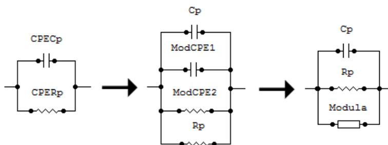
Fig. 3.5.6.1. Conversion of the experimentally found parallel connection of CPE-Cp and CPE-Rp into the parallel connection of capacitance, resistance and modula impedance
