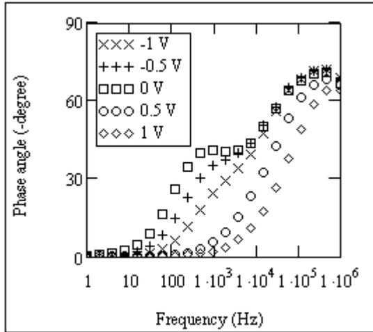
**Fig. 3.2.2.** Dependence of the impedance phase angle on ac frequency in case of the structure of glass/ITO/PLD-CISE/ZnPc
