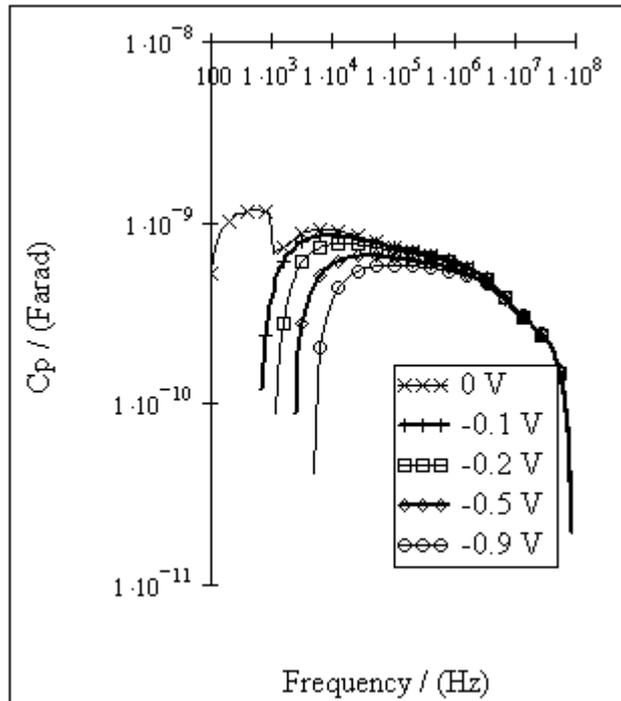
**Fig. 3.5.1.5. Structure of glass/ITO/CISE/graphite parallel capacitance vs. frequency plots at zero and reverse biases**
