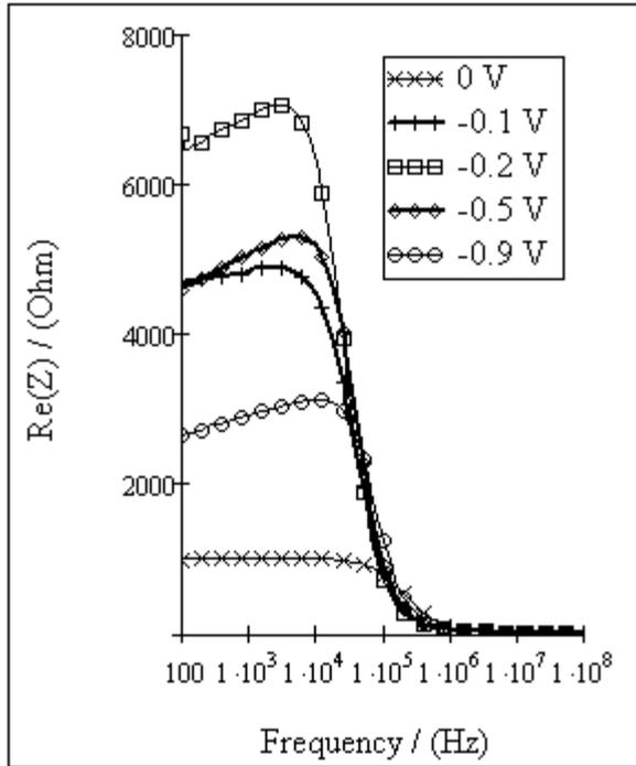
**Fig. 3.5.1.1. Structure of glass/ITO/CISe/graphite impedance real part dependence on measuring signal frequency at zero and reverse biases**
