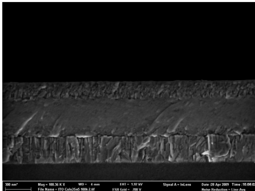
Fig. 3.3.1. Cross-sectional SEM micrograph of glass/ITO/HVE  $\text{CuIn}_3\text{Se}_5$  as-deposited
