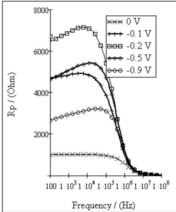
**Fig. 3.5.1.4. Structure of glass/ITO/CISE/graphite parallel resistance vs. frequency plots at zero and reverse biases**
