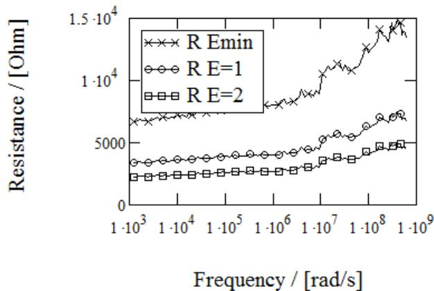
Fig. 3.5.4.1. Resistance calculated at different values of  $E$  for converting a resistive-like CPE into resistance and modula CPE (curve of  $E_{\min}$  corresponds to the situation, and then  $E$  is calculated according to Eq. 1.7.1.8a, reverse bias -0.2 V)
