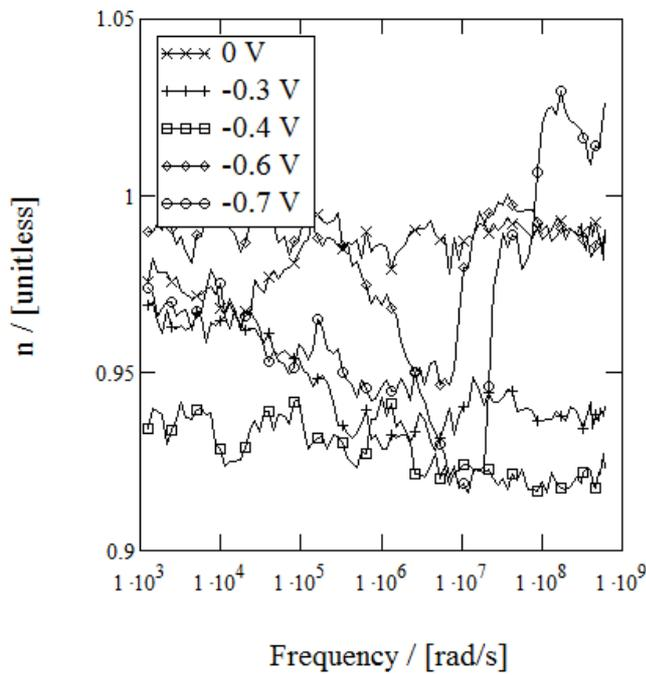
Fig. A1.8. Equivalent circuit (Fig. 3.4.3 in main text) element CPE-Cs parameter  $n$  frequency dependence on different applied reverse biases
