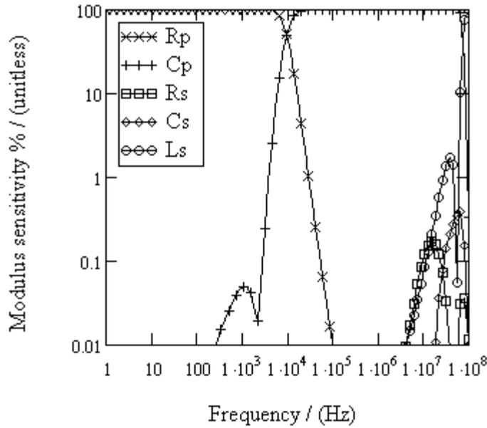
Fig. 3.5.2.5. Sensitivity analysis of the impedance modulus according to the formula of the circuit represented on the Fig. 3.5.2.1 (reverse bias -0.3 V as an example)
