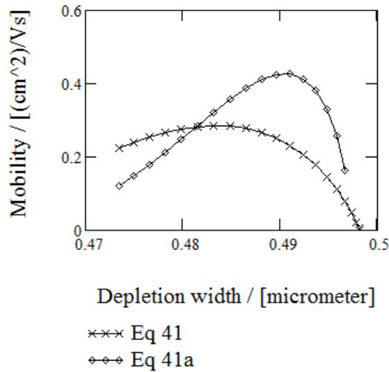
**Fig. 3.5.8.2a.** Estimation of the mobility of holes in the structure of glass/ITO/CuIn<sub>3</sub>Se<sub>5</sub> according to the measurements at forward bias
