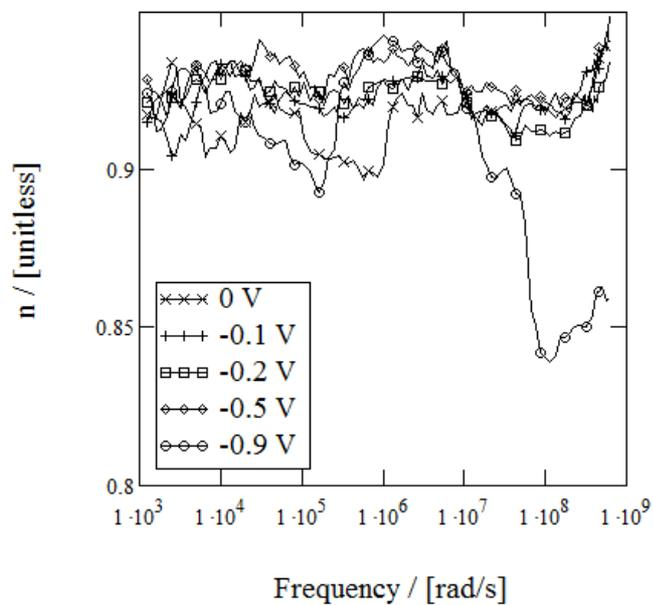
Fig. A1.4. Equivalent circuit (Fig. 3.4.3 in main text) element CPE-Cp parameter  $n$  frequency dependence on different applied reverse biases
