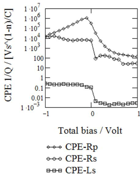
**Fig. 3.4.4.** Dependence of the  $1/Q$  of the CPE-Rp and CPE-Rs vs. total bias applied on structure of glass/ITO/CuIn<sub>3</sub>Se<sub>5</sub> annealed at 450°C for 1 hour with following deposition of the graphite dot-contacts ( $1/Q$  is the parameter of CPE element with the dimension of  $V \cdot s^{(1-n)}/C$ )
