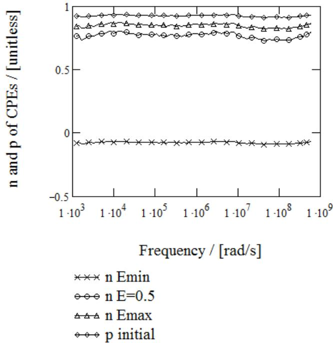
**Fig. 3.5.3.2. Exponential parameters ( $n$ ) of CPE calculated according to two limiting conditions, with  $E=0.5$  and compared with the curve of initial CPE exponential parameter ( $p$ ) (curve of  $E_{max}$  corresponds to the situation, then  $E=1$ , curve of  $E_{min}$  is then Eq. 1.6.14c is used, reverse bias  $-0.2$  V)**
