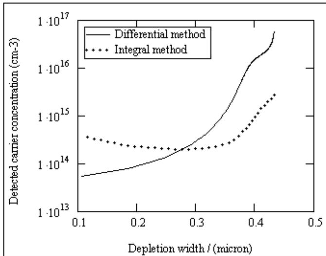
**Fig. 3.2.9.** Concentration profiles of the shallow level defects in the structure of glass/ITO/PLD-CuIn<sub>3</sub>Se<sub>5</sub>/ZnPc calculated using two different methods
