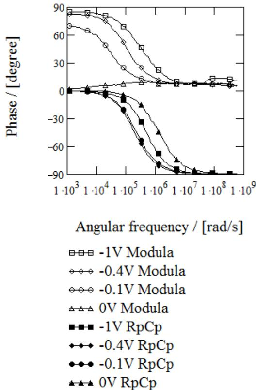
**Fig. 3.5.6.5.** Comparison of phases of the impedance of the connection where the resistance and the capacitance are in parallel, and that of the modula impedance. (responses corresponding to the same bias are marked with similar margins: empty margins for modula phase, filled for the phase of the parallel resistance and capacitance)
