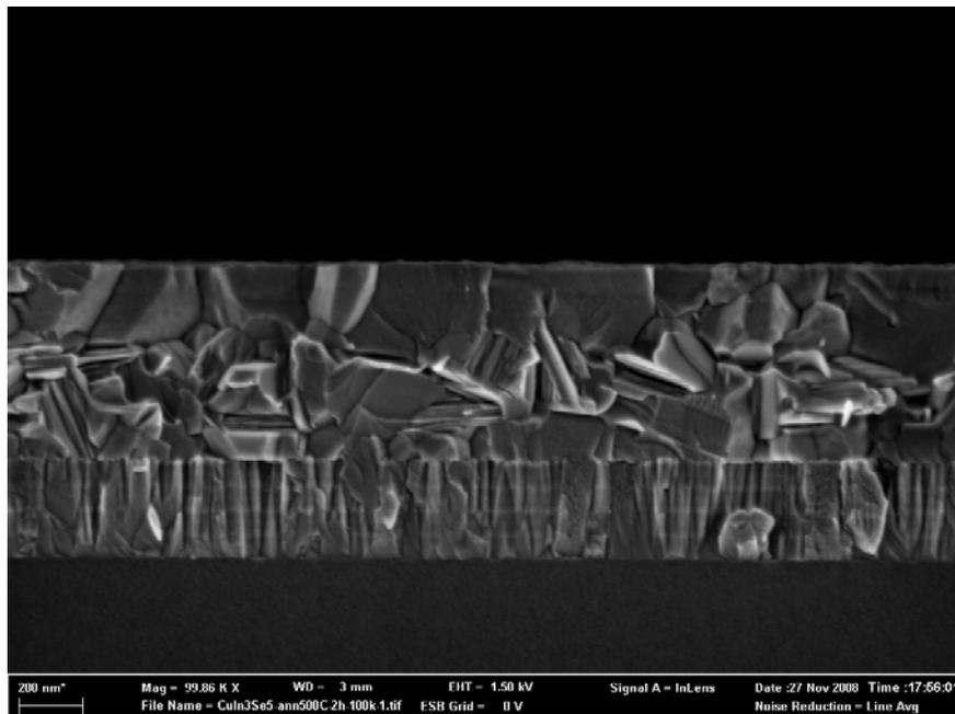
**Fig. 3.3.3.** SEM micrograph of the ITO/ HfV  $\text{CuIn}_3\text{Se}_5$  annealed at  $500^\circ\text{C}$  for 2 hour in argon atmosphere
