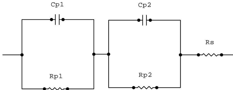
**Fig. 3.2.4.** The equivalent circuit applied for the analysis of the IS data for glass/ITO/PLD-CISE/ZnPC ( $C_{p1}$  and  $C_{p2}$  are capacitors while the  $R_{p1}$  and  $R_{p2}$  are the resistors of the two subcircuits in series connection,  $R_s$  is a series resistor)
