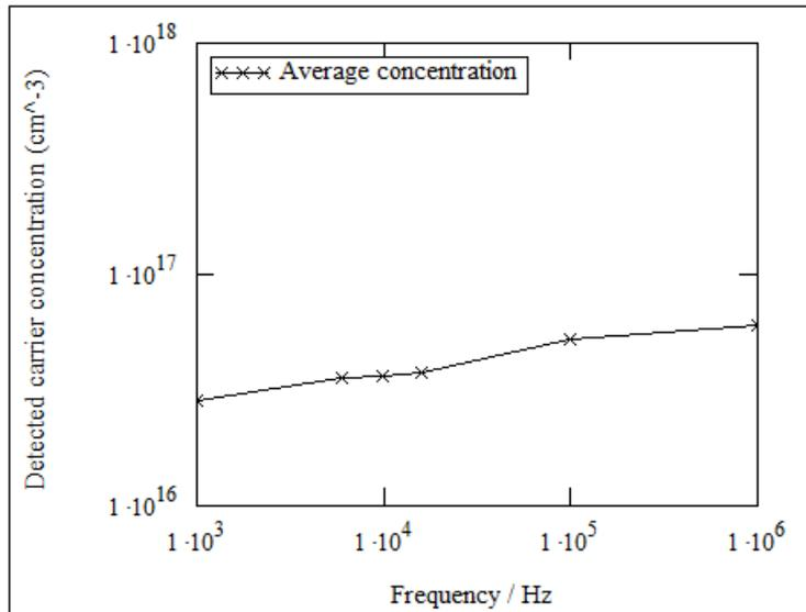
**Fig. 3.4.10.** Free charge carriers averaged concentrations for the glass/ITO/CuIn<sub>3</sub>Se<sub>5</sub> annealed at 450°C for 1 hour, calculated at different measurement frequencies
