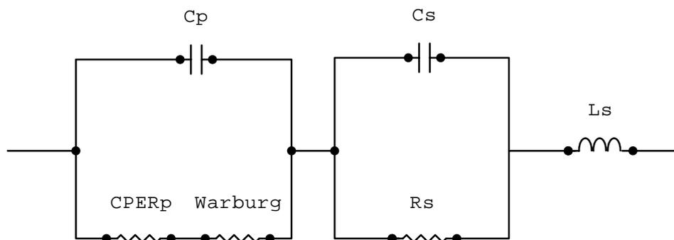
**Fig. 3.5.2.2. Equivalent circuit found to describe the impedance behavior of the glass/ITO/CISE/graphite structure (CPE notation in the name of circuit element CPE  $R_s$  points to the circumstance that this element is a CPE element resembling a resistor, Warburg is the CPE element with  $n=0.5$ )**
