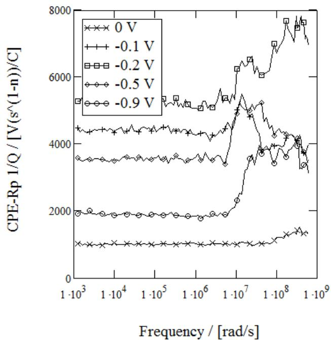
Fig. A1.1. Equivalent circuit (Fig. 3.4.3 in main text) element CPE-Rp parameter  $1/Q$  frequency dependence on different applied reverse biases
