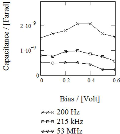
**Fig. 3.5.7.2a.  $C$ - $V$  curves of the glass/ITO/CuIn<sub>3</sub>Se<sub>5</sub>/graphite structure measured at forward biases and at different frequencies of the ac signal**
