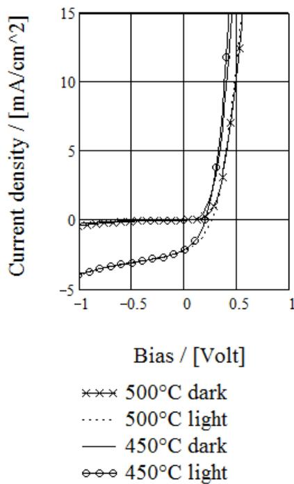
**Fig. 3.3.6.  $I$ - $V$  curves of the glass/ITO/HVE  $\text{CuIn}_3\text{Se}_5$ /graphite structures annealed at 450 and 500 °C**
