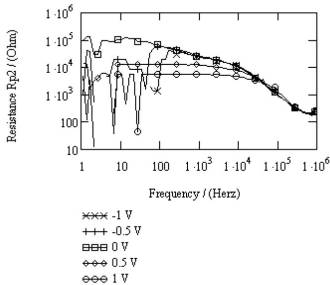
**Fig. 3.2.5d.** Results of the circuit calculation there impedances of two similar (difference is a half of the decade) frequencies were used for circuit evaluation ( $R_{p2}$  vs. frequency)
