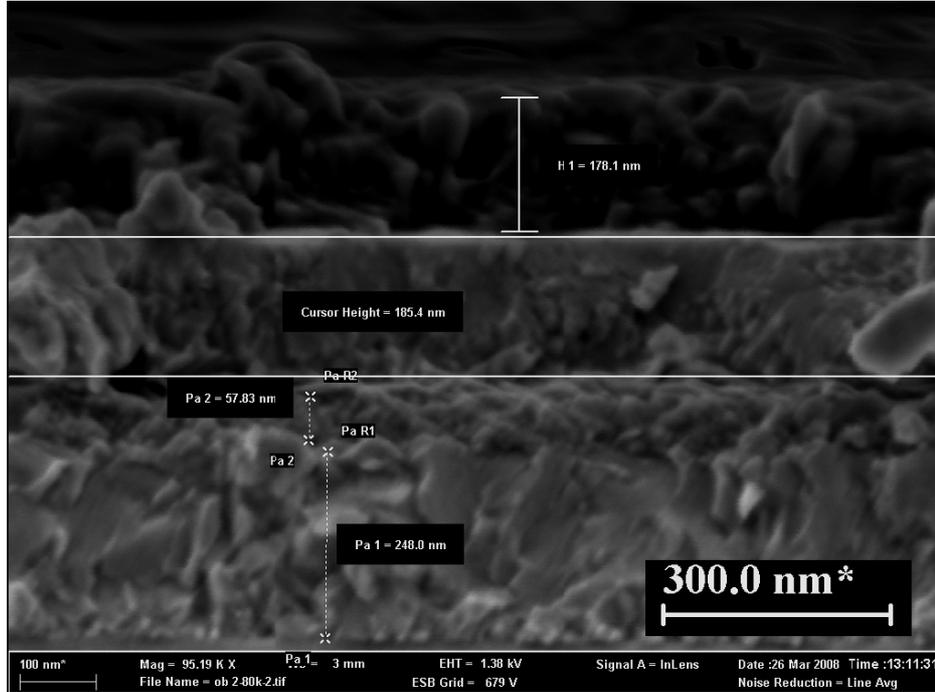
Fig. 3.1.1. SEM micrograph of the glass/ITO/ $\text{CuIn}_3\text{Se}_5$ /ZnPc
