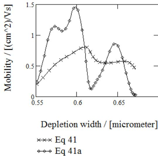
**Fig. 3.5.8.2. Estimation of the mobility of holes in the structure of glass/ITO/HVE CuIn<sub>3</sub>Se<sub>5</sub> according to the measurements at reverse bias**
