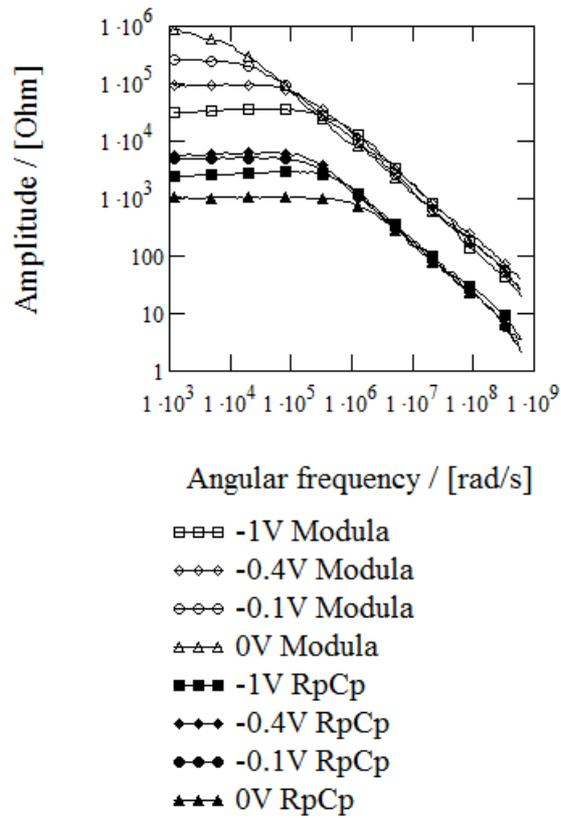
**Fig. 3.5.6.4. Comparison of amplitudes of the impedance of the connection there the resistance and the capacitance are in parallel, and that of the modula impedance. (responses corresponding to the same bias are marked with similar margins: empty margins for modula impedance, filled for the impedance of the parallel resistance and capacitance)**
