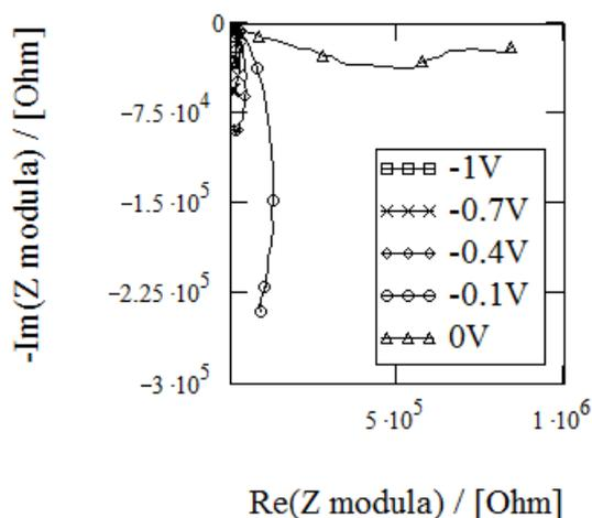
Fig. 3.5.6.2. Nyquist plots of the modula impedance calculated according to the transformation schematically reported on Fig. 3.5.6.1
