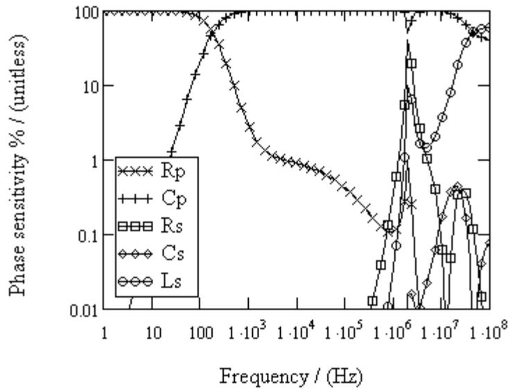
Fig. 3.5.2.6. Sensitivity analysis of the impedance phase according to the formula of the circuit represented on the Fig. 3.5.2.1 (reverse bias -0.3 V as an example)
