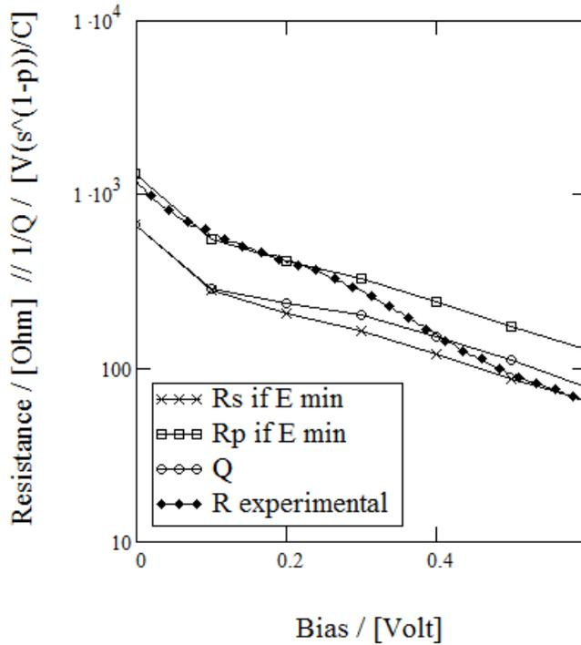
Fig. 3.5.5.4. Comparison of  $I$ - $V$  measurement (forward bias) based differential resistance with the resistance predicted from Eq. 1.7.2.10 and the  $Q$  of the resistance-like CPE (measurement frequency 200 Hz)
