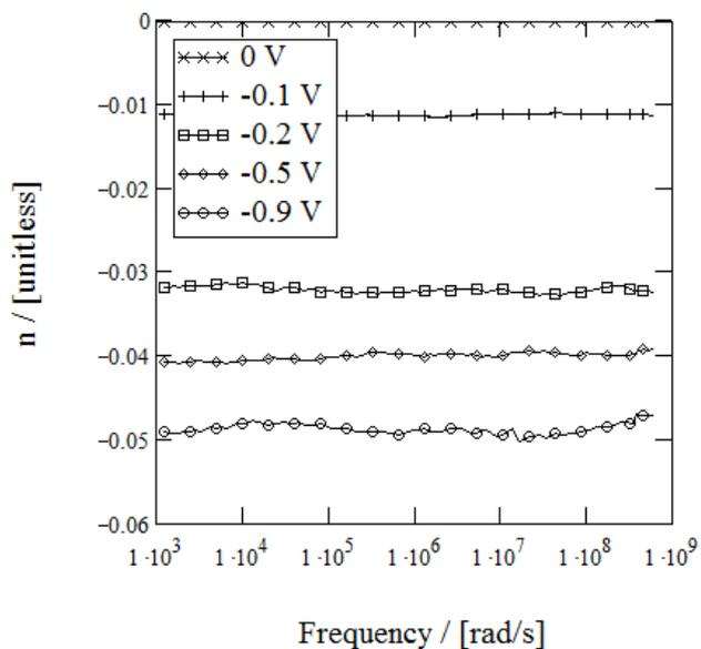
Fig. A1.2. Equivalent circuit (Fig. 3.4.3 in main text) element CPE-Rp parameter  $n$  frequency dependence on different applied reverse biases
