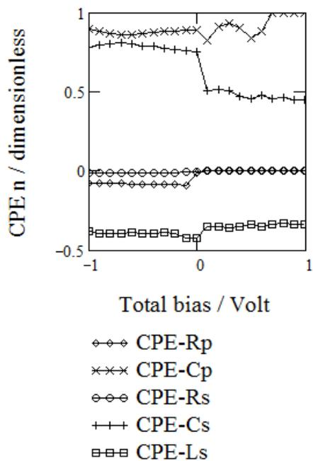
Fig. 3.4.6. Dependence of the  $n$  of the CPE-s on total bias applied on structure of glass/ITO/CuIn<sub>3</sub>Se<sub>5</sub> structures annealed at 450°C for 1 hour with following deposition of the graphite dot-contacts
