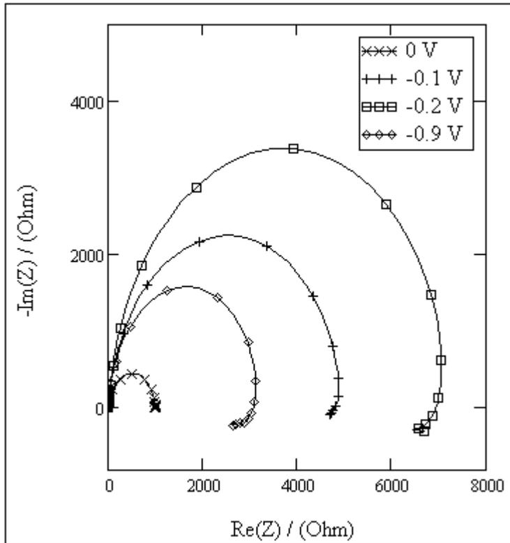
**Fig. 3.5.1.3. Structure of glass/ITO/CISE/graphite Nyquist plots at zero and reverse biases**
