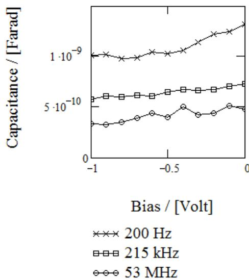
**Fig. 3.5.7.2.  $C$ - $V$  curves of the glass/ITO/CuIn<sub>3</sub>Se<sub>5</sub>/graphite structure measured at reverse biases and at different frequencies of the ac signal**
