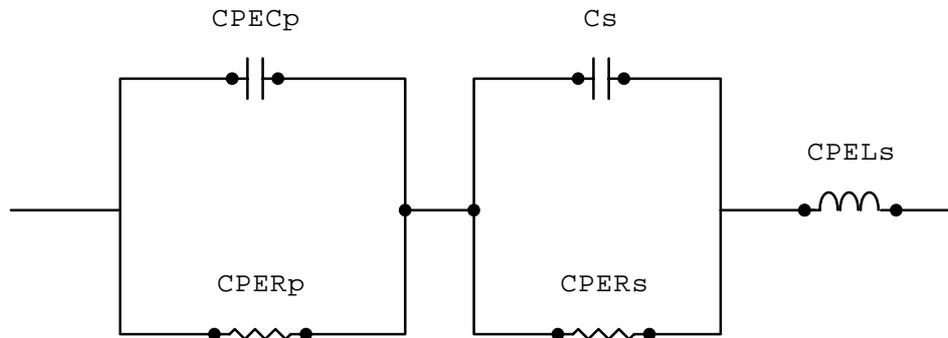
**Fig. 3.5.2.1. Equivalent circuit found to describe the impedance behavior of the glass/ITO/CISE/graphite structure (CPE notation in names of circuit elements of CPE  $C_p$ , CPE  $R_p$ , CPE  $R_s$  and CPE  $L_s$  points to the circumstance that these elements are CPE elements resembling either capacitors, resistors or inductors)**
