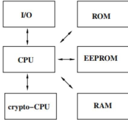
Figure 1. Components of smart cards [5].
