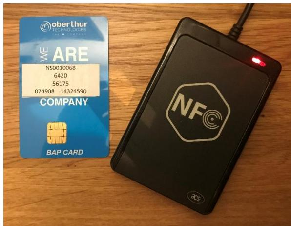
Figure 10. Test ID-Card and ACR1251U contactless USB reader.
