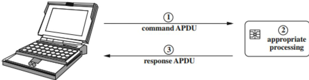
Figure 2. Smart card communication model [5].
