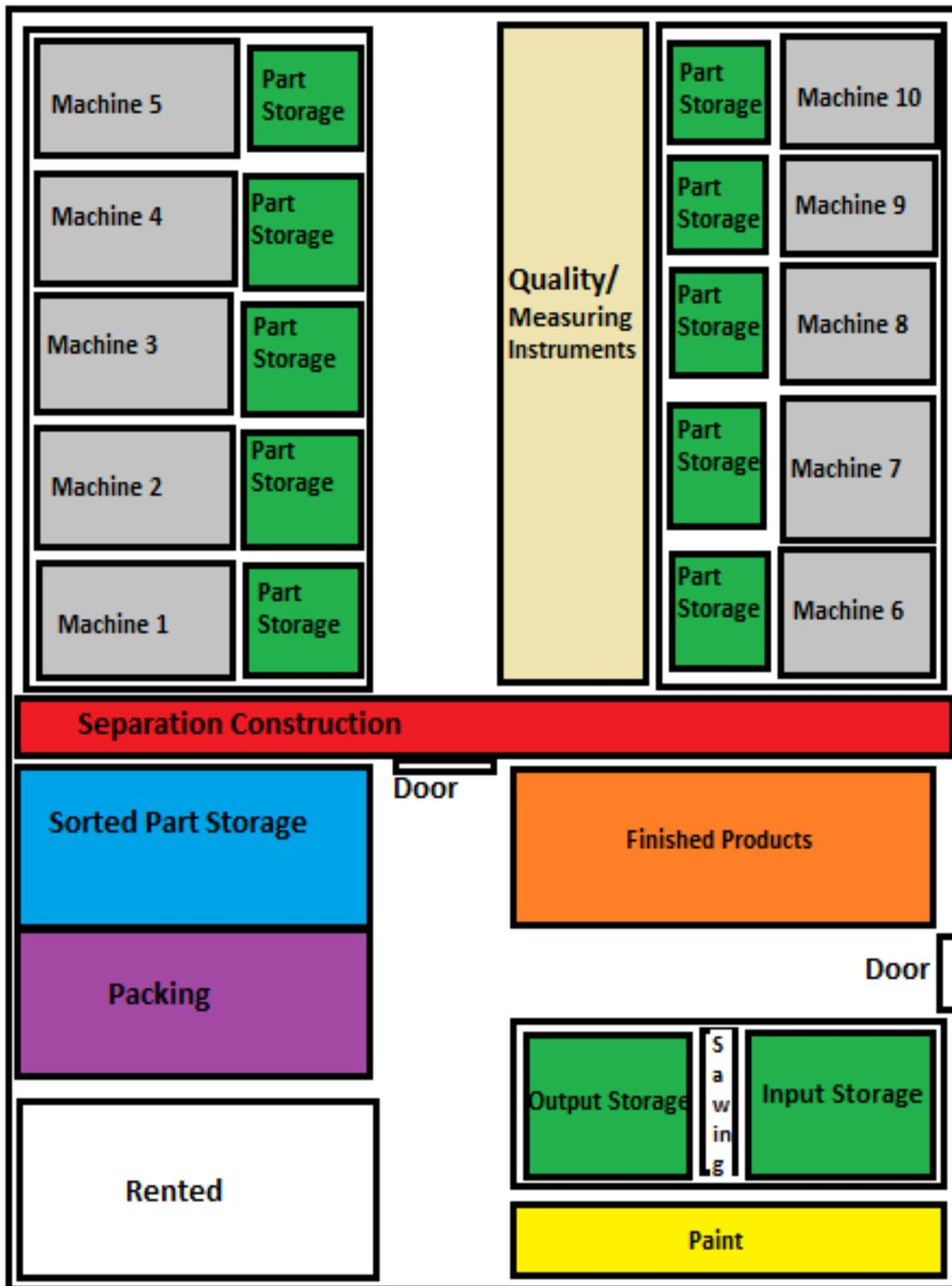
Figure18 Proposed floor plan of the workshop
