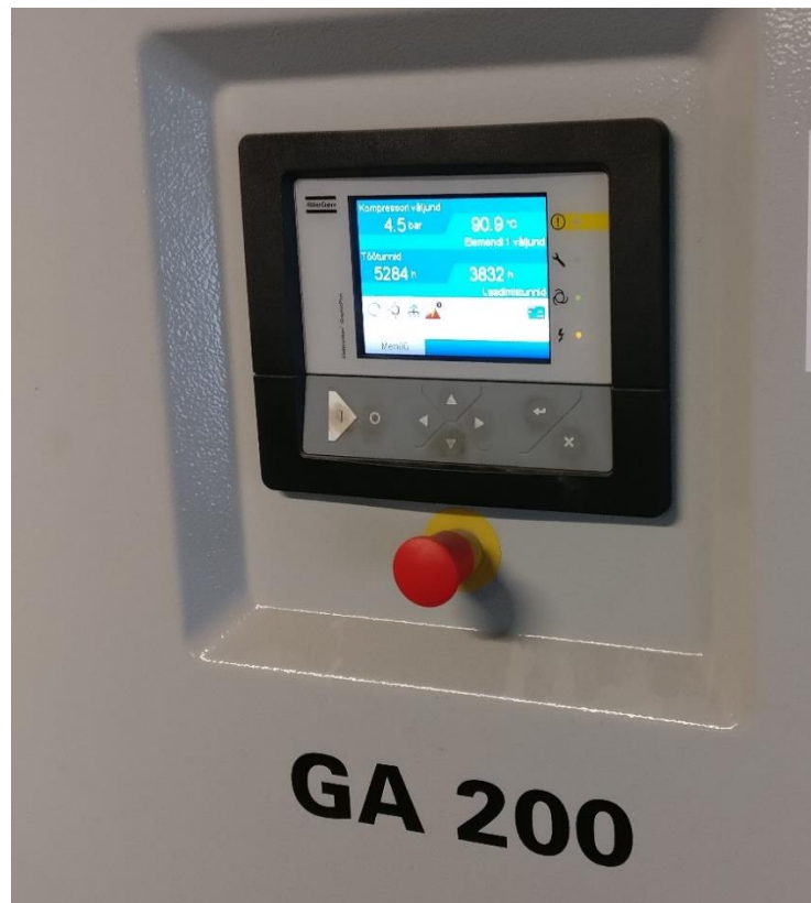
Figure 5.2 Atlas Copco GA 200 interface with IoT integration
