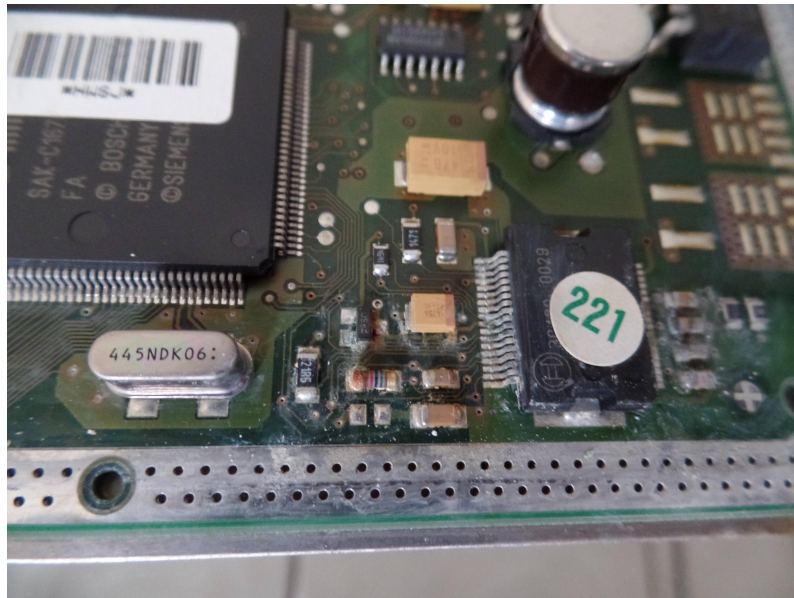
Figure 4. Water damage to the PCB and corrosion [10].
