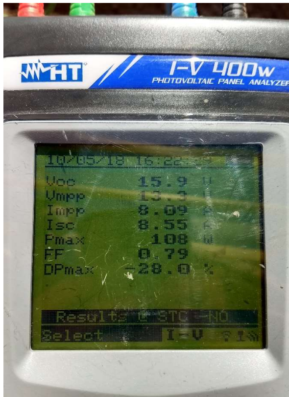
Figure 2.7. Characteristics of second module, measured by PV analyzer HT I-V 400w
