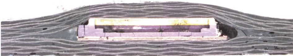
Figure 4.2 Tensile specimens after delamination failure
