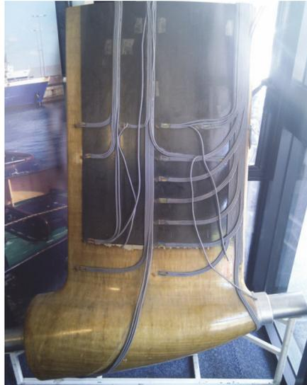
Figure 1.1 Strain gauge rosettes mounted on a ship's underwater appendage structure
