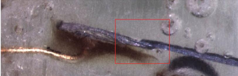
Figure 13: Sensor failure due to cracking
