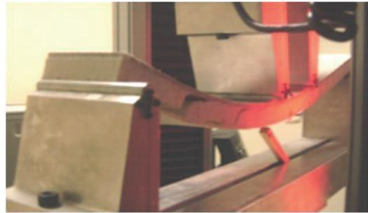
**Fig. 4.** Shear failure of sandwich panel with PET core in 4-point bending test
