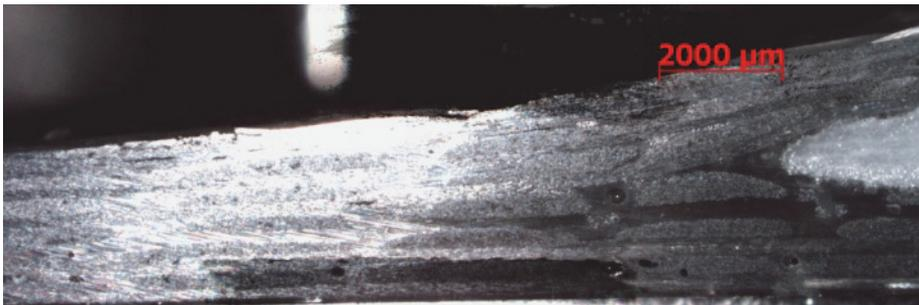
Figure 4.16 Specimen number 5 cross-section image. Foreign object visible at the right side of the image.
