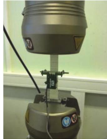
**Fig 2.** Tensile test of the GFRP laminate
