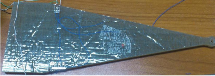
Figure 1: Vinylester specimen during wire soldering process
