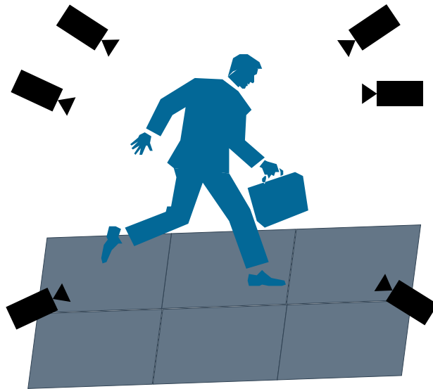
Figure 2: Modern gait analysis laboratory. Cameras are located for 3-dimensional capture of kinematic and temporal-spatial data. Also uses force plates in walkways.
