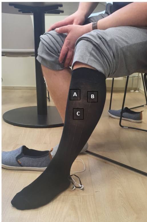
Figure 5: Example of the wearable electrodes integrated into the sock
