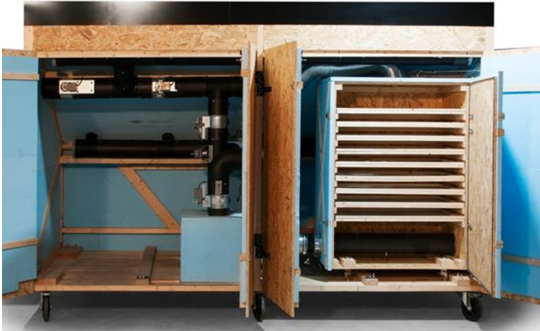
Figure 6. The test bench of food dehydrator (view from the back)
