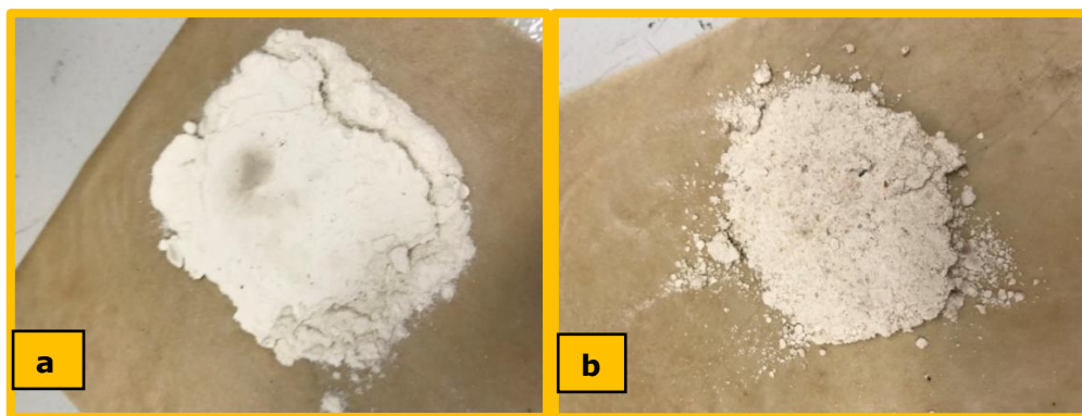
Figure 23. (a) The compression moulded CA sample with the molar ratio of 1:1, (b) CA sample with the molar ratio of 1:2
