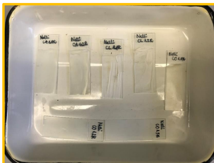
Figure 25. The prepared solution cast film samples, two CA samples are presented in the left upper corner of the figure
