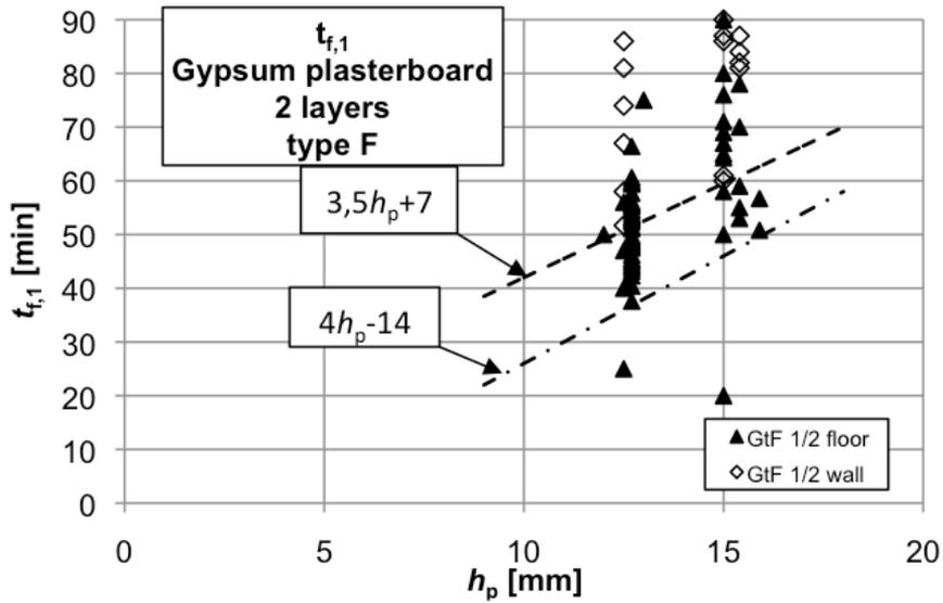
Figure 10 – Fall off of first layer of two for gypsum plasterboards type F. Equations provided by this study.
