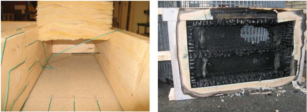
Figure 2.6. Assembly of a test specimen at SP Trätekt (left). Test specimen after fire test (right)
