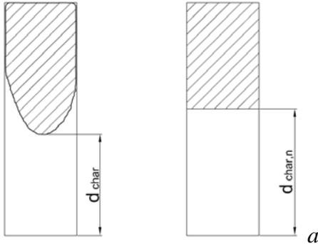
Figure 3 – Description of charring depths of cross-sections.
