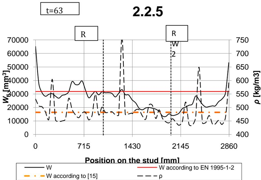
**Figure 10** – Variability of section modulus of charred cross-sections and density for stud 2.2.5.
