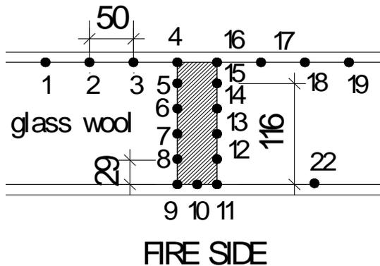
Figure 2. Test set-up for floor structures
