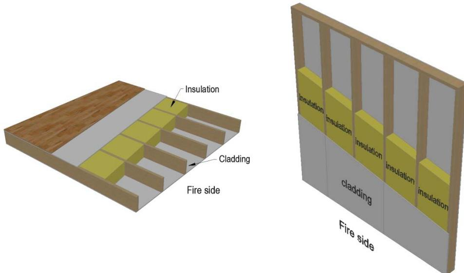
Figure 1.1. Timber frame assemblies: floor (left) and wall (right)
