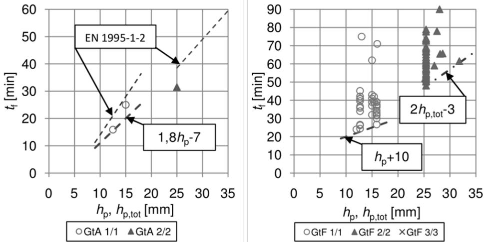
The database consists of test walls with timber studs and steel studs. Difference of failure times can not be seen. According to test results in database it can be stated that the failure times of gypsum boards on steel studs and on wooden studs are similar. A distance between floor beams or resilient channels can be neglected when creating conservative equations. However the use of the results presented here are restricted to a spacing of 600 mm.
