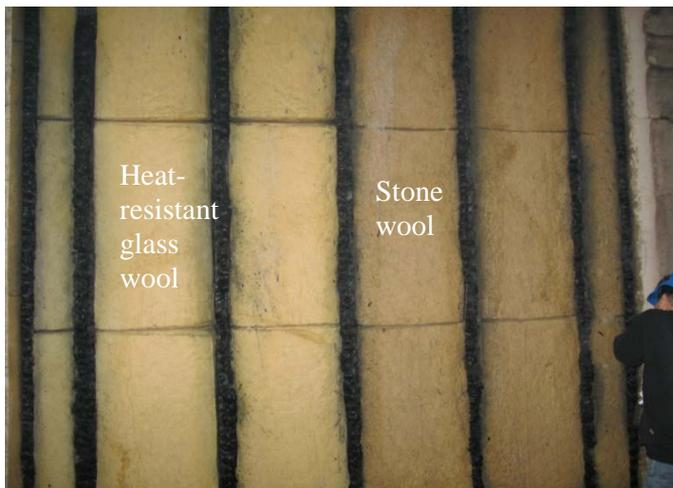
Figure 3.9. Insulation after the 60 minutes fire test. Heat-resistant glass wool (left) and stone wool (right)
