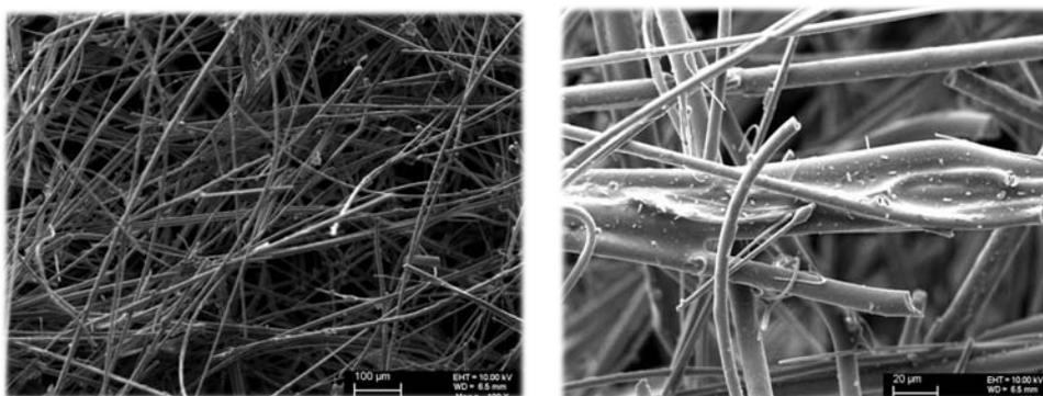
Figure 1.9. Structure of glass wool at 100µm (left) and 20 µm scale (right)
