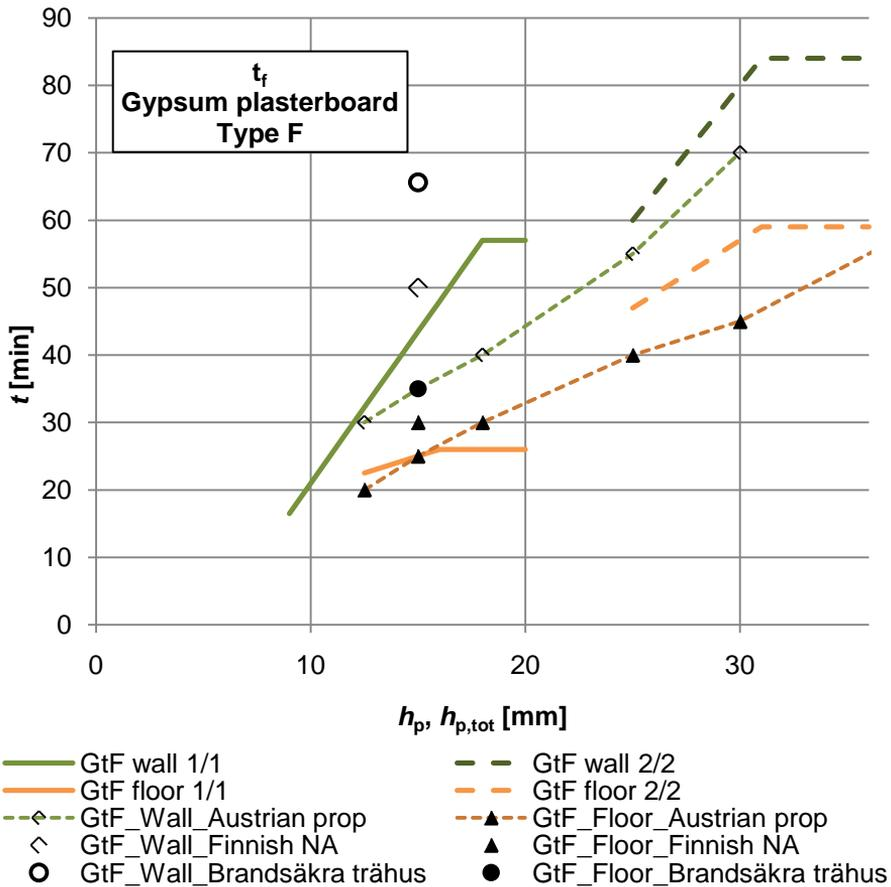
Figure 4.3. Failure times of Type F gypsum plasterboards. Comparison of present research with other resources
