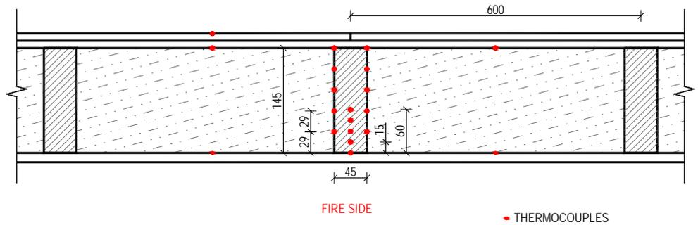
Figure 2.5. Location of thermocouples inside and on sides of cross-section with cladding on the fire exposed side
