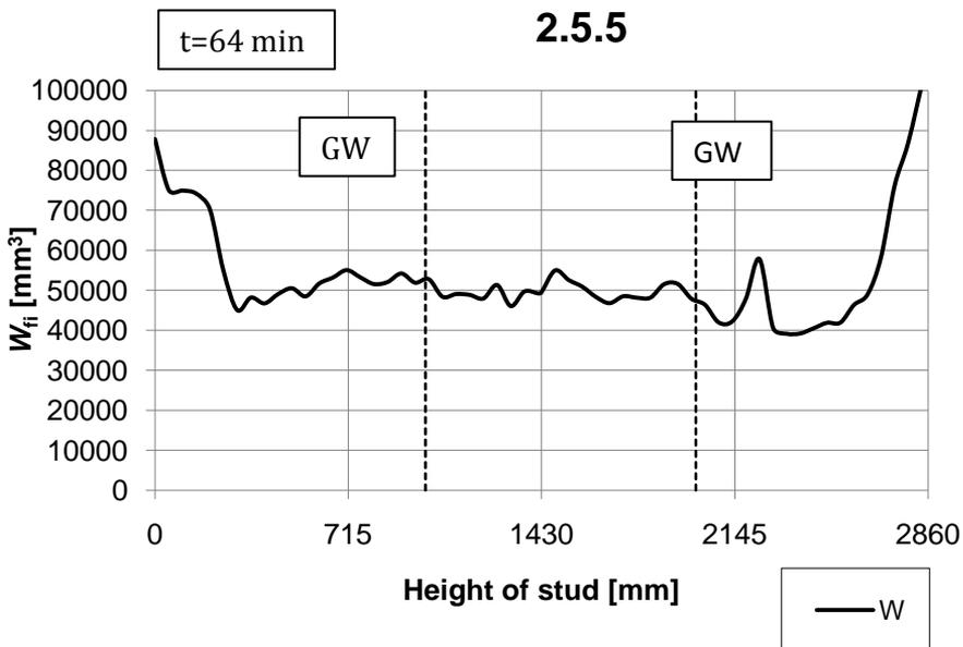
Figure 3.13. Variability of charring along a wooden stud insulated by glass wool and covered by Type F, gypsum plasterboard
