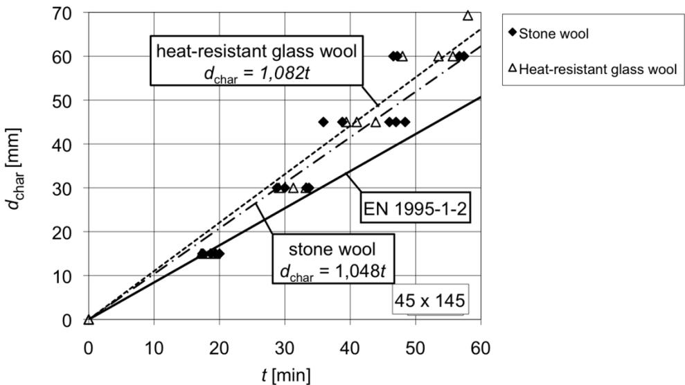
Figure 5 – Linear explanation of the charring rates for studs insulated by heat-resistant glass wool and stone wool.
