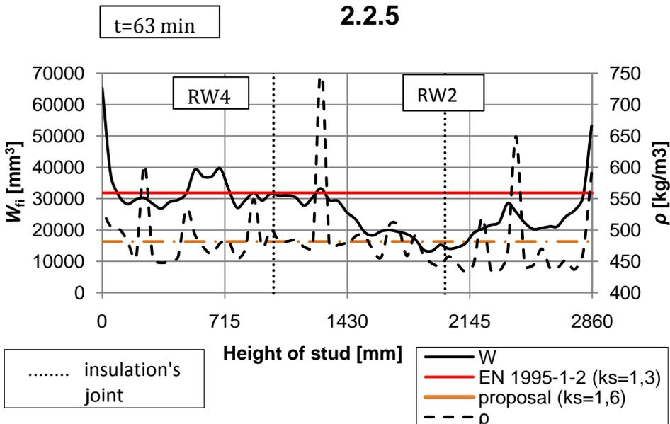
Figure 3.11. Variability of charring along a wooden stud insulated by two different stone wools
