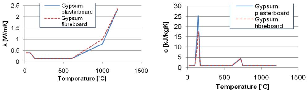
Figure 1.6. Relationship between thermal conductivity,  $\lambda$ , and specific heat,  $c$ , of gypsum boards, and temperature [16]
