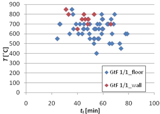
Figure 3.3. Relationship between fall-off temperatures behind the board and failure times of single layer claddings in wall structures with GtF boards
