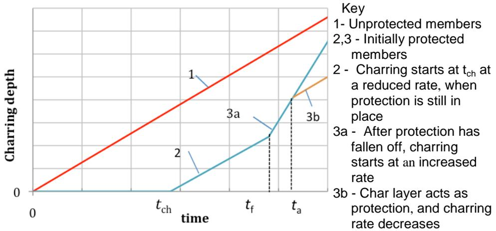
Figure 1.3. Charring of unprotected and protected timber members
