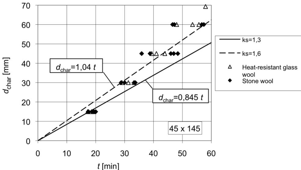
Figure 6 – Proposal for cross-section factor for heat-resistant insulations.
