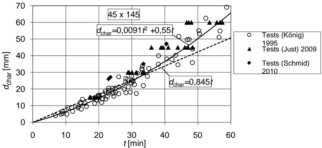
Figure 3 – Comparison of charring depths from [7] insulated by stone wool with new results of charring depth of wall studs insulated with heat-resistant mineral wool.
