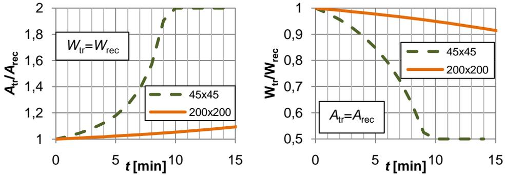
Figure 3.6. Comparison of change of section properties of trapezoidal and rectangular cross sections during fire development
