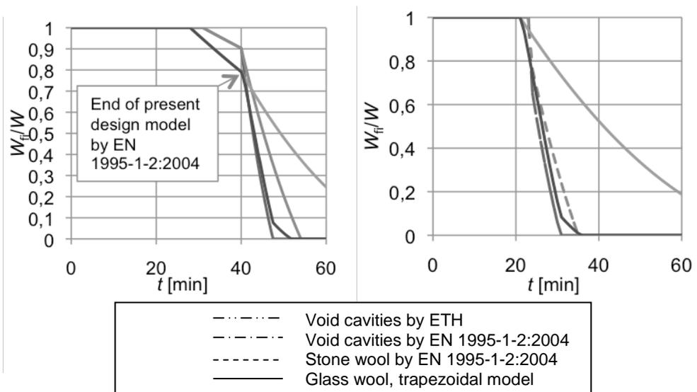
Figure 4. Example of existing and new design models for timber frame assembly with gypsum plasterboard type A (left) and type F (right) with timber studs 45x145 mm<sup>2</sup>.
