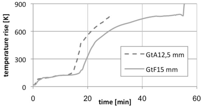
Figure 3 – Temperature rise behind gypsum claddings type A and F in standard fire test (example)
