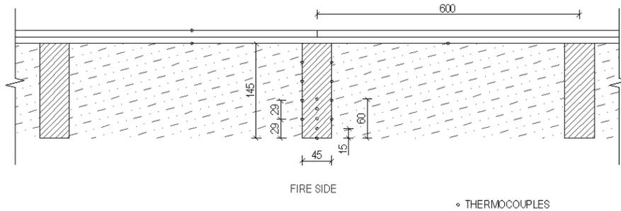
Figure 2 – Location of thermocouples on timber member
