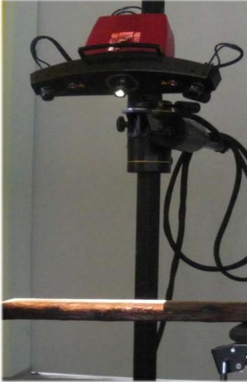
**Figure 6** – 3 dimensional scanner ATOS II.
