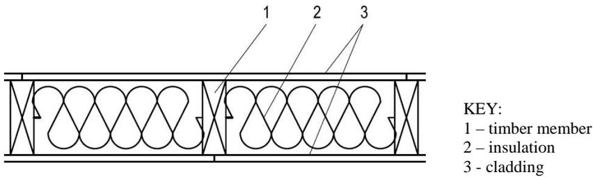
**Figure 1** – Typical timber frame assembly
