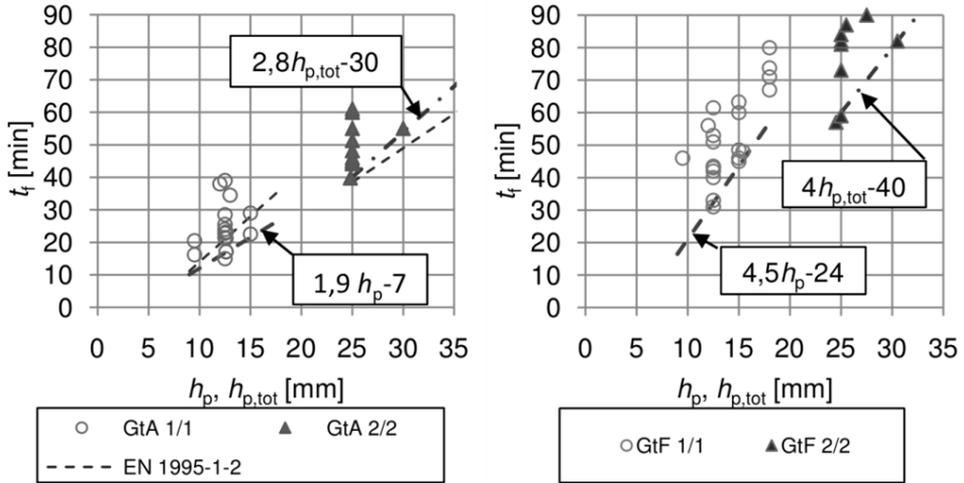
Figure 3. Equations for failure times of floor claddings of gypsum plasterboards type A (left) and type F (right).
