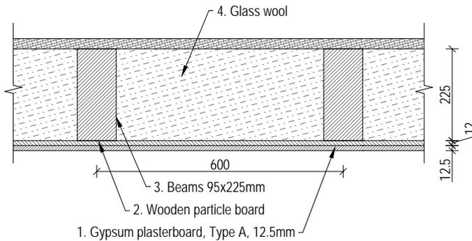
Figure 4.10. Cross-section of wall assembly
