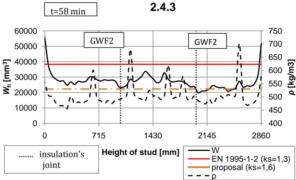
Figure 3.10. Variability of charring along a wooden stud insulated by heat-resistant glass wool
