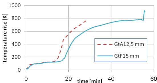
Figure 1.7. Temperature rise behind Type A and Type F gypsum claddings in standard fire tests (example)
