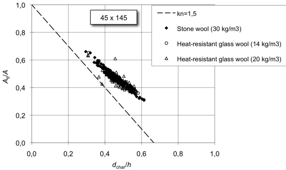
Figure 10 – Reduction of cross-section area versus charring depth ratio. Test results.
