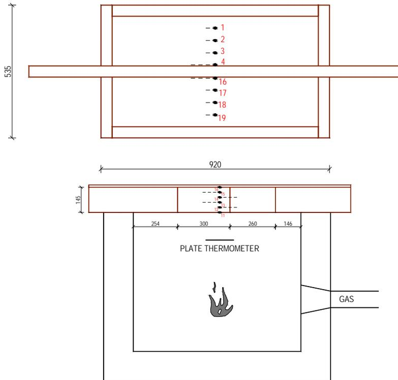
Figure 2.2. Medium scale floor test sample with location of thermocouples. Layout (upper) and view from side (lower).
