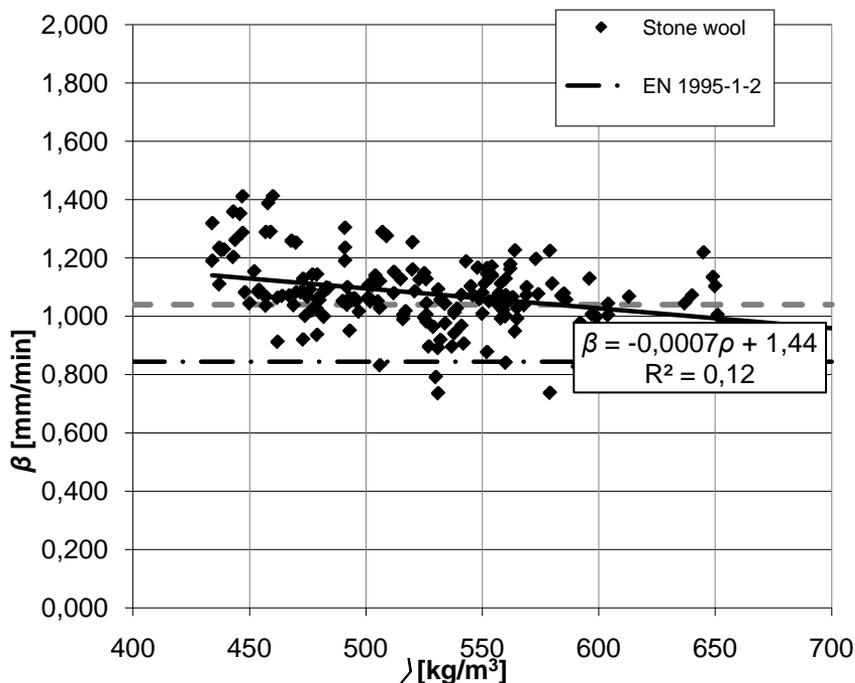
**Figure 12** – Relation between density and charring rate of timber members insulated by stone wool
