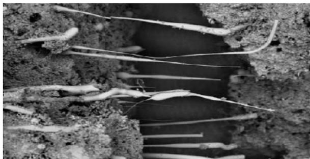
Figure 1.5. Glass fibres in fire-rated gypsum plasterboard
