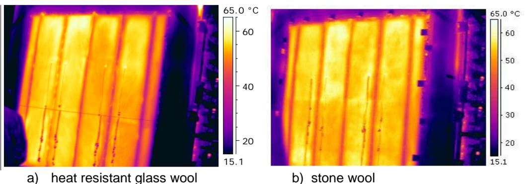
Figure 3.7. Temperature distribution at unexposed side in fire test after 60 minutes
