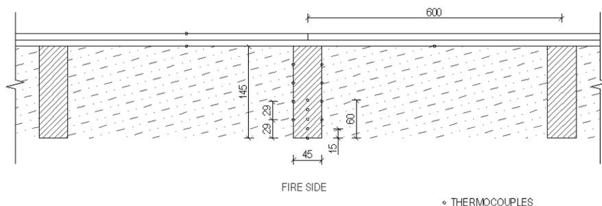
Figure 2 – Location of thermocouples on timber member
