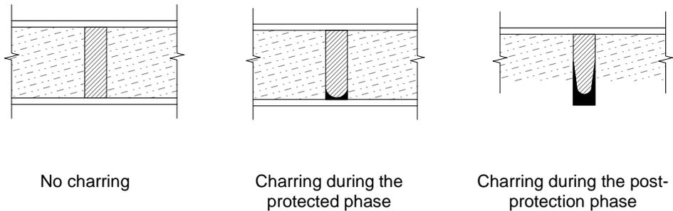
Figure 1.2. Protection phases of timber frame assemblies in fire
