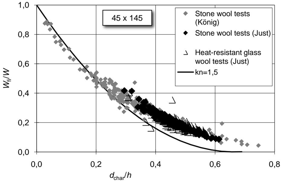
Figure 9 – Reduction of section modulus versus charring depth ratio. Comparison of test results.
