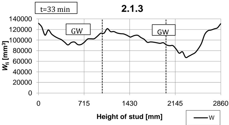
Figure 3.12. Variability of charring along a wooden stud insulated by glass wool and covered by Type A gypsum plasterboard
