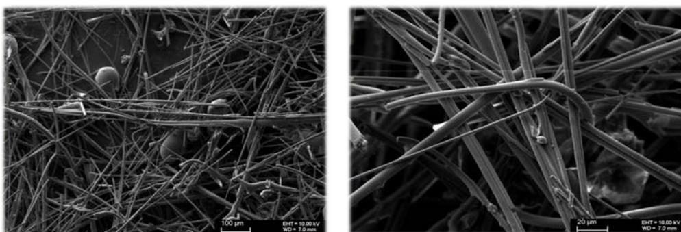
Figure 1.8. Structure of stone wool at 100 μm (left) and 20 μm scale (right)
