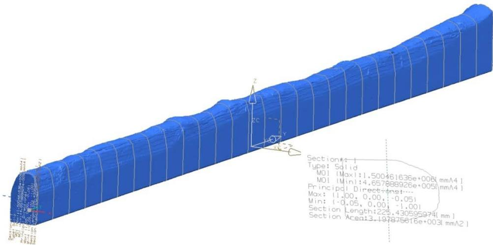
**Figure 8** – Digitized 3 dimensional model with example of cross-section data.
