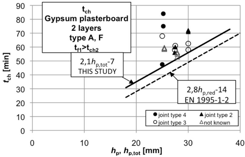
Figure 6 – Start time of charring for cladding of two layers of gypsum plasterboards when first layer does not fall off before the charring starts. Equation provided by this work is compared to EN 1995-1-2.
