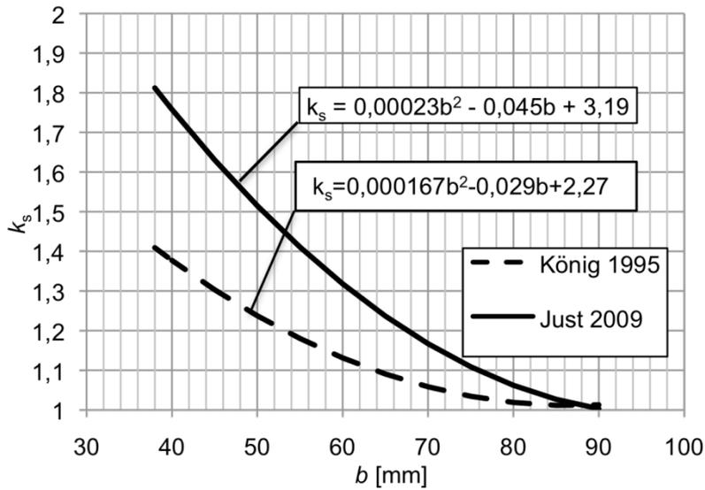
Figure 7 – Coefficient  $k_s$  depending on cross-section width.
