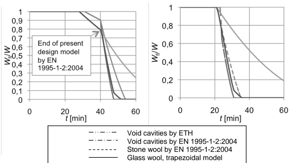
Figure 4. Example of existing and new design models for timber frame assembly with gypsum plasterboard type A (left) and type F (right) with timber studs 45x145 mm<sup>2</sup>.
