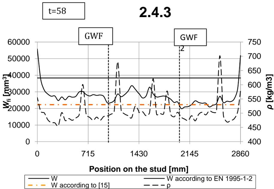
**Figure 11** – Variability of section modulus of charred cross-sections and density for stud 2.4.3.
