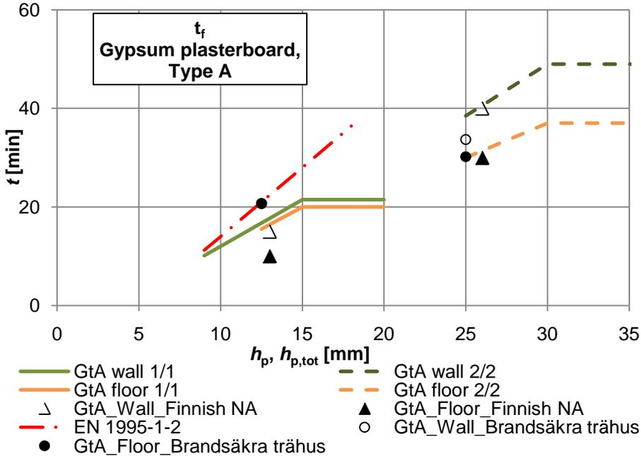
Figure 4.2. Failure times of Type A gypsum plasterboards. Comparison of present research with other resources
