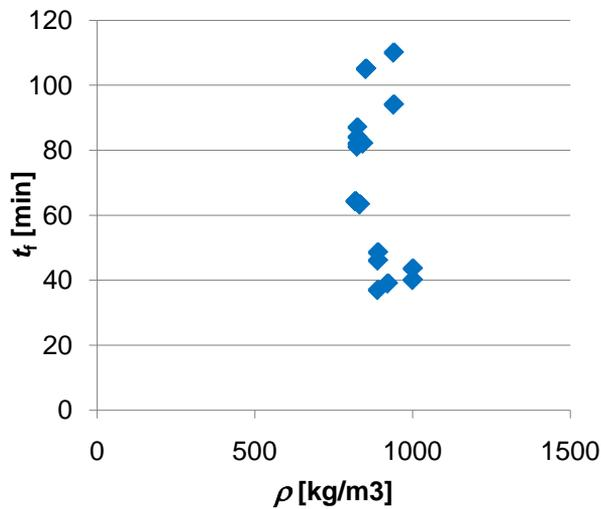
Figure 3.2. Relationship between density of board and failure time of single-layer claddings in wall structures with GtF boards
