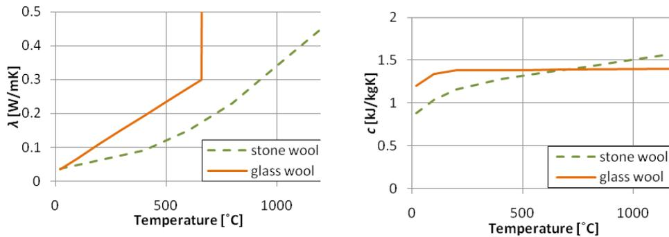
Figure 1.10. Effective thermal conductivity,  $\lambda$ , and specific heat,  $c$ , of stone wool and glass wool [16]
