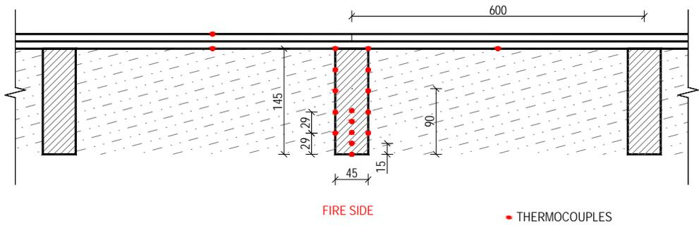
Figure 2.4. Location of thermocouples inside and on sides of cross-section without cladding on the fire exposed side
