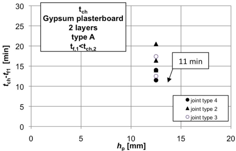
Figure 7 – Start time of charring after fall off of first layer for gypsum plasterboard type A
