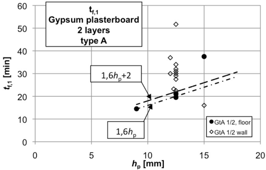
Figure 9 – Fall off of first layer of two for gypsum plasterboards type A. Equations provided for wall and floor structures by this study.
