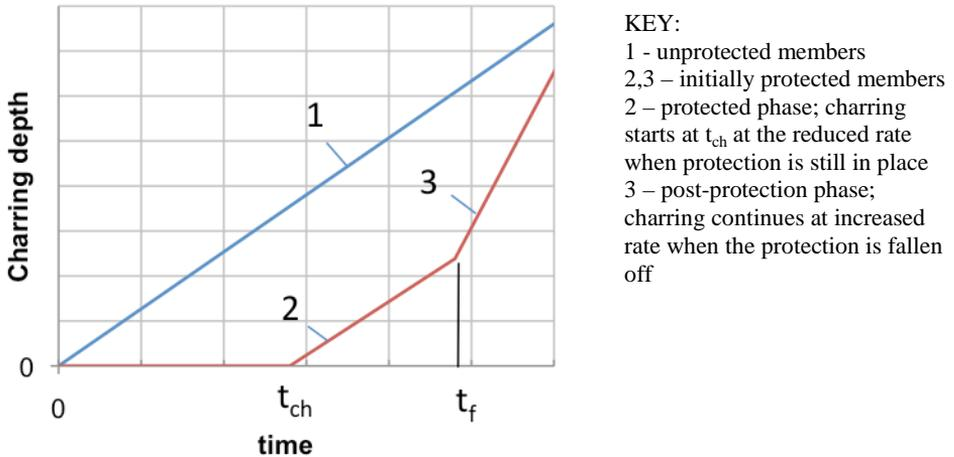
Figure 2 – Charring of timber studs with and without protection
