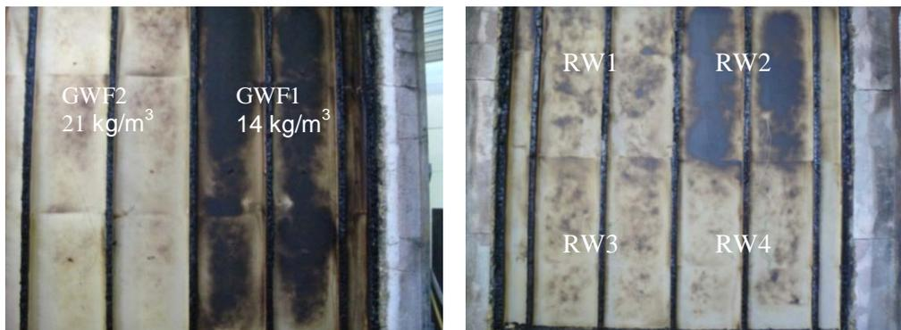
Figure 4.5. Surface behind heat-resistant glass wool (left) and different stone wools (right)
