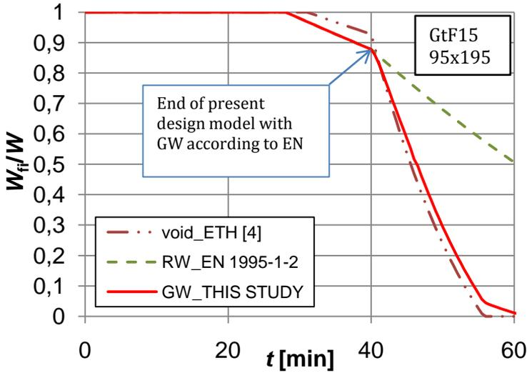
Figure 4.7. Example of the new design model for a structure with Type F gypsum plasterboard and 95x195 mm timber studs
