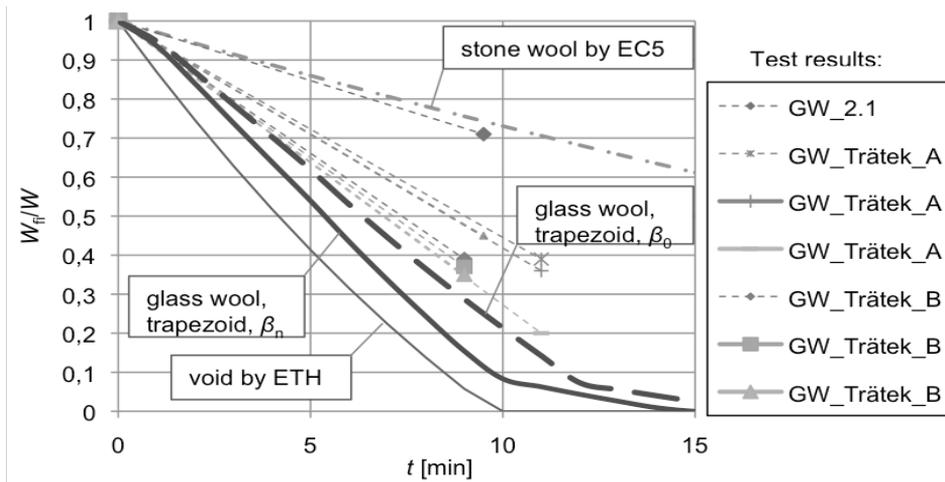
Figure 5. Comparison of calculation method with the test results.
