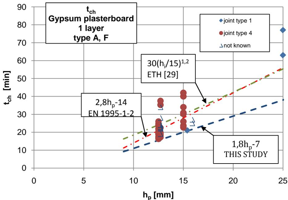
Figure 4.1. Start times of charring  $t_{ch}$  from database. Comparison of different methods
