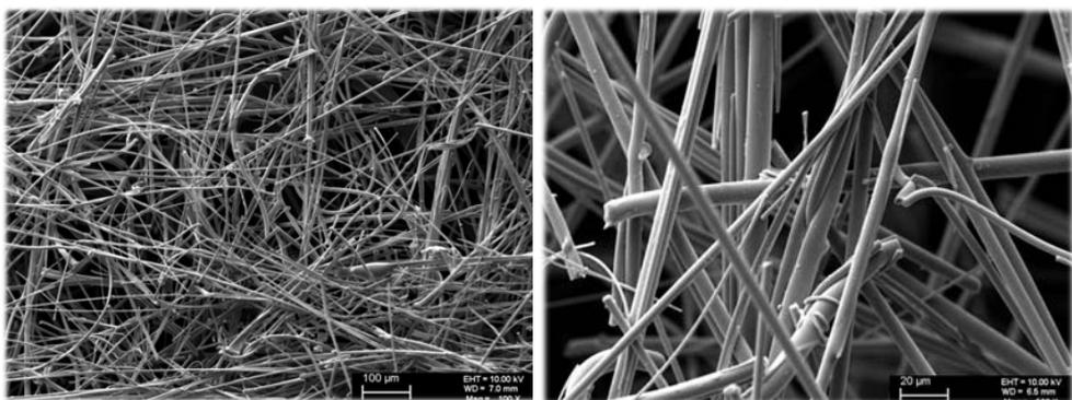
Figure 1.11. Structure of the heat-resistant glass wool at 100µm (left) and 20 µm scale (right)
