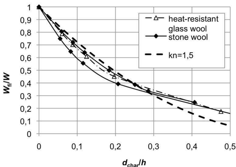
Figure 8 – Change of section modulus versus charring depth ratio during the test.
