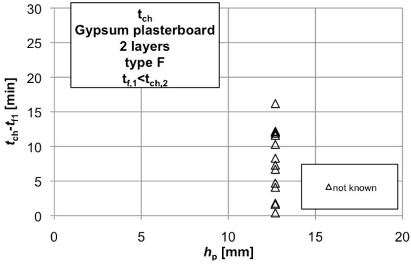
Figure 8 – Start time of charring after fall off of first layer for gypsum plasterboard type F
