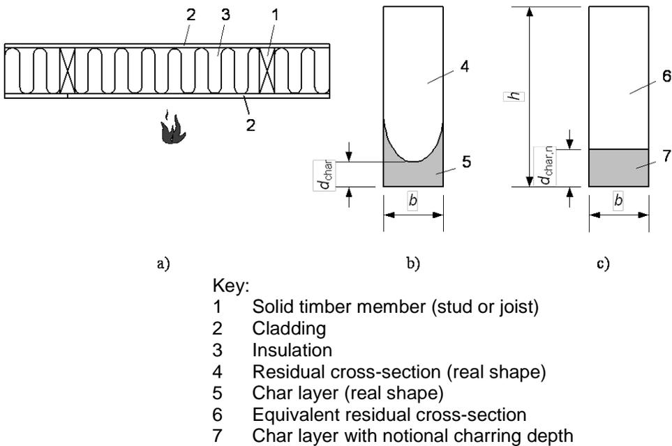
Figure 1 – Charring of timber frame member (stud or joist): a. Section through assembly. b. Real residual cross-section and char layer. c. Notional charring depth and equivalent residual cross-section
