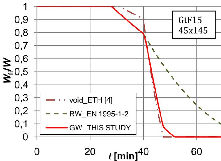
Figure 4.6. Decreasing of section modulus. Example of existing and new design models for timber frame assembly with Type F gypsum plasterboard and 45x145 mm timber studs. Comparison with test results
