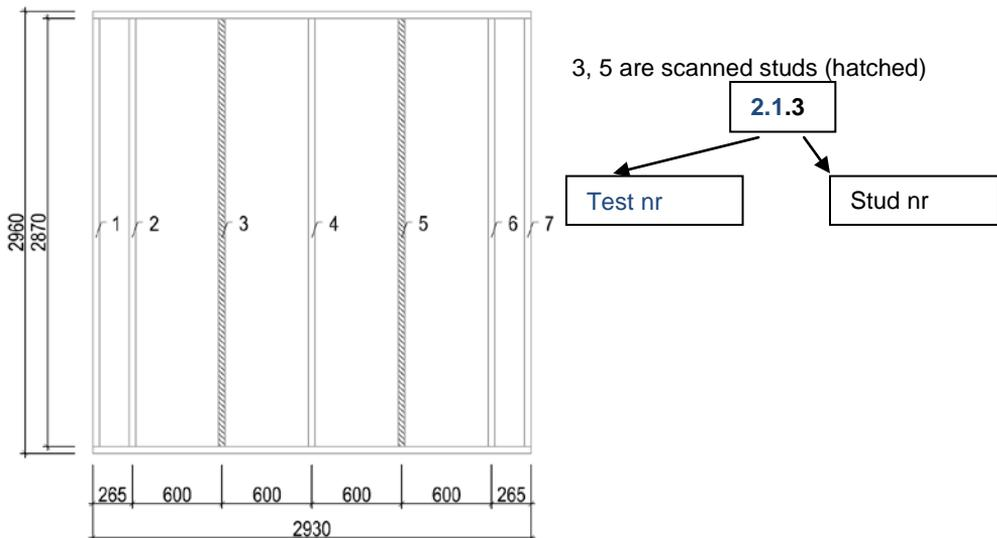
Figure 2.1. Definition of stud numbers of tested full-scale walls. View from the fire side
