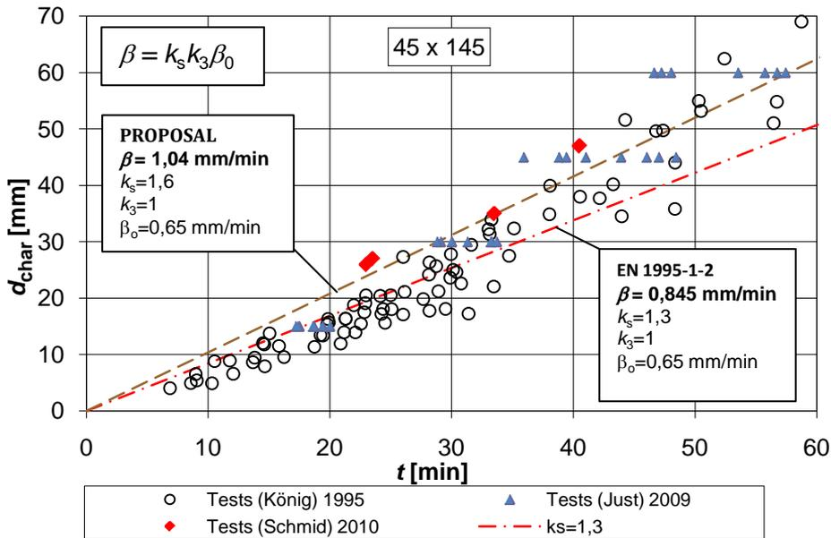
Figure 4.4. Charring rate of tested timber members insulated with heat-resistant glass wool. Comparison of results from the past with recent findings
