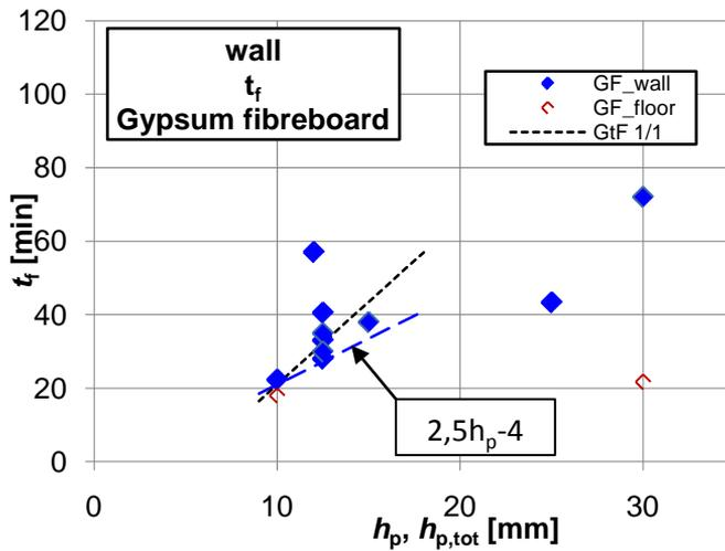
Figure 3.1. Failure times of gypsum fibreboards in wall assemblies
