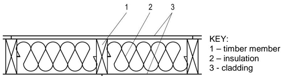
Figure 1 – Typical timber frame assembly
