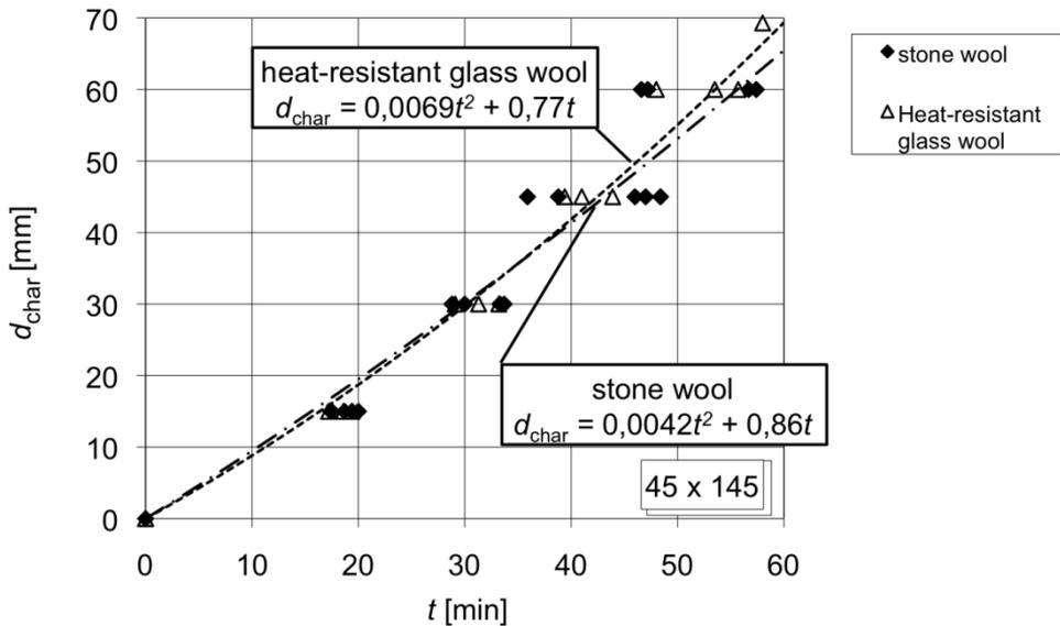
Figure 4 – Charring depth for studs protected by stone wool and heat-resistance glass wool respectively. Polynomial trendlines.
