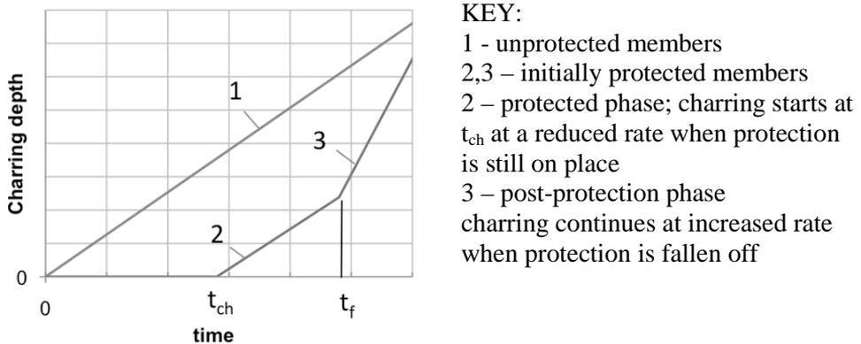
Figure 2 – Charring of timber studs with and without protection
