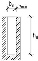
Figure 4.9. Notional effective cross-section
