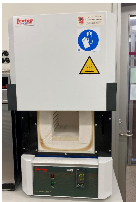
Figure 2.6. Furnace used for selenium crystallisation
