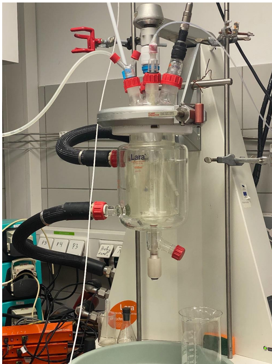
Figure 11 LARA™ controlled lab reactor used for leaching and carbonation experiments.
