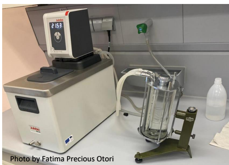
Figure 8 Hoppler viscometer with Julabo heating circulator used for measuring liquid viscosity.
