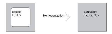
Figure 1.5 Homogenization of explicit structure to equivalent homogenized media.
