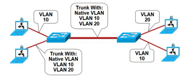
Figure 11: Basic VLAN hopping attack [38, p. 13].
