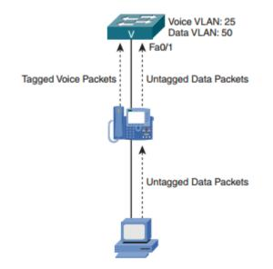
Figure 8: Separating voice and data traffic using VLANs [28, p. 58].
