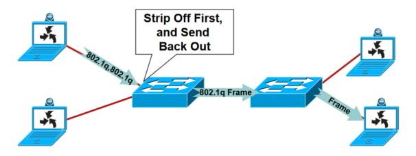
Figure 13: Double 802.1Q encapsulation VLAN hopping attack [38, p. 14].
