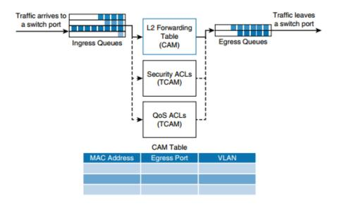
Figure 4: Layer 2 switch operation mechanics [20, p. 26].
