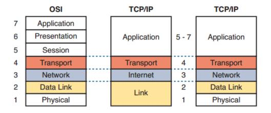
Figure 1: OSI model compared to the two TCP/IP models [8, p. 33].
