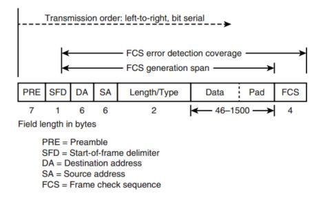
Figure 2: The basic IEEE 802.3 MAC data frame format [20, p. 4].
