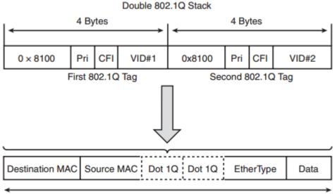
Ethernet Frame with Two 802.1Q Tags (Not to scale)
