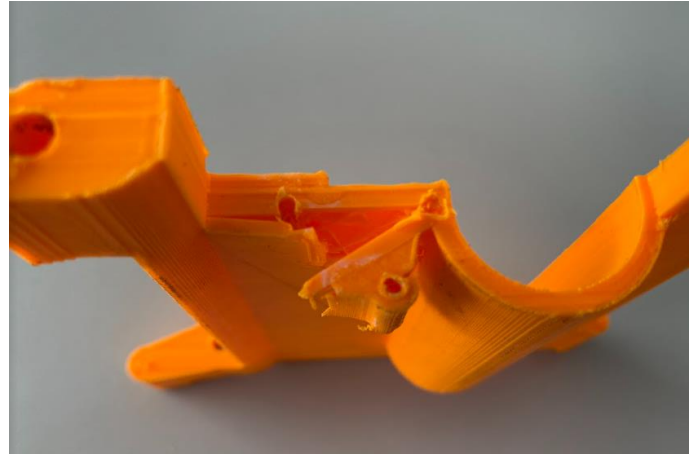
Figure 6.2 Front plate damaged during the tests
