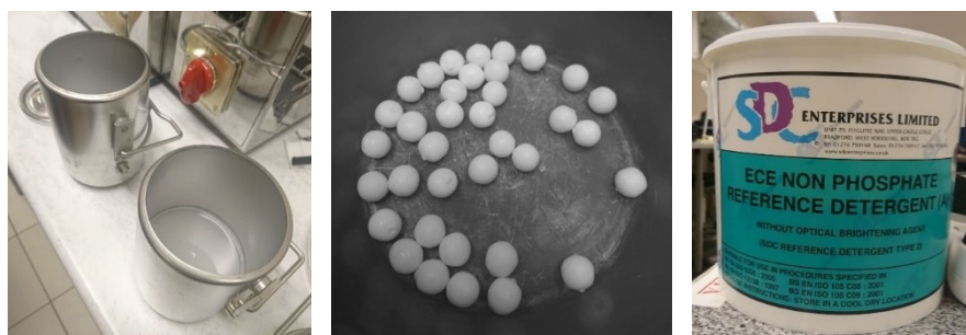
Figure 7.3.2.1. Materials used for testing from the left: stainless steel containers, teflon balls, standard detergent.
