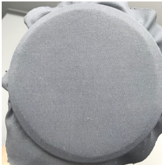
Figure A4.2. Fabric 4A. Grey knitted Rec PA after 2000 rubs
