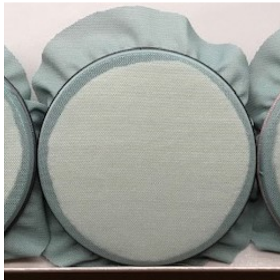
Figure A4.4. Fabric 4A. Green mesh Rec PA after 2000 rubs
