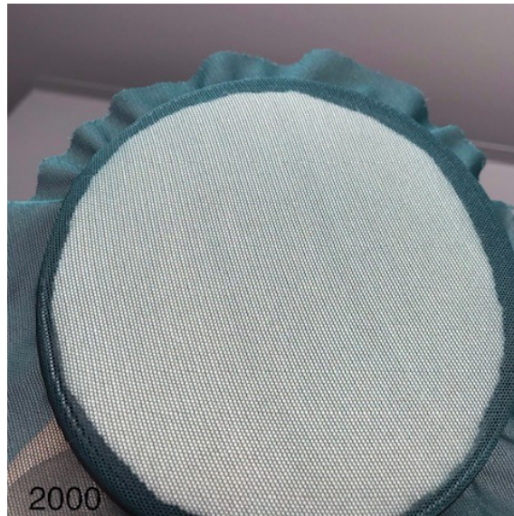
Figure A4.3. Fabric 2C. Green mesh PA after 2000 rubs
