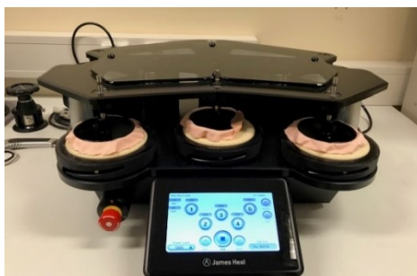
Figure 7.3.4.1. James Heal Martindale abrasion and pilling tester
