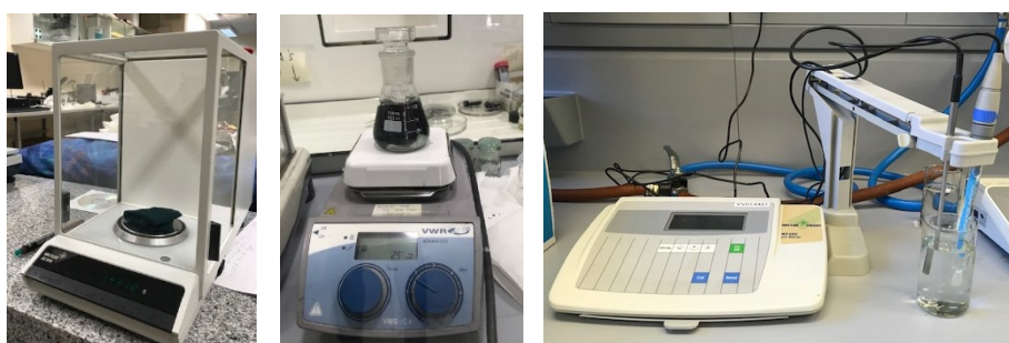
Figure 7.3.6.1. Machinery for pH testing, from the left: balance, magnetic stirrer, pH- meter.
