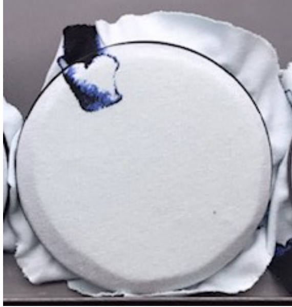
Figure A4.7. Fabric 7A. Blue printed Refibra after 2000 rubs
