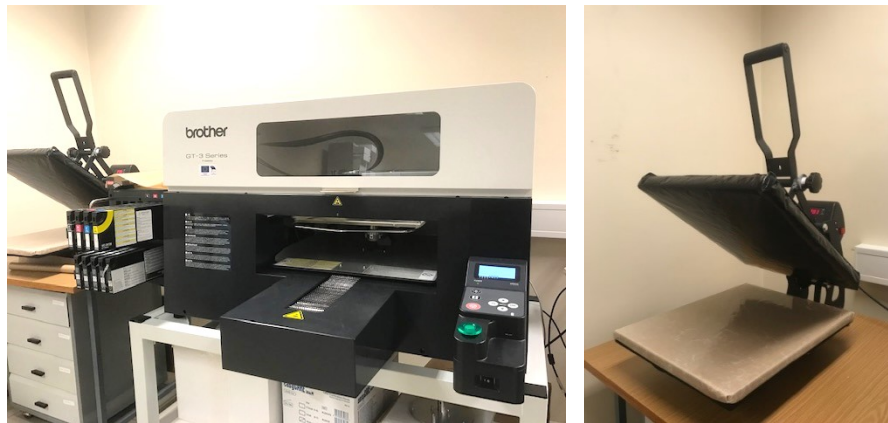
Figure 7.4.1.1. From the left: Brother GT-341 Series textile printer and Stahls MAXX® Clam Heat Press
