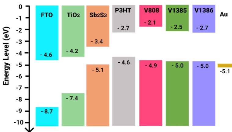
Figure 3.11. Band energy diagram of  $Sb_2S_3$  solar cell stack with different HTMs (P3HT, V808, V1385 and V1386).
