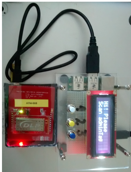
Figure 9, Complete prototype with the RFID reader
