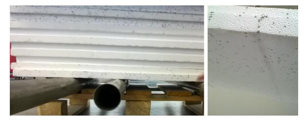
Figure 34 – One of the surface strength tests of the EPS plates: with loading in excess of 160 kg on rollers of 30 mm in diameter spaced at 300 mm
