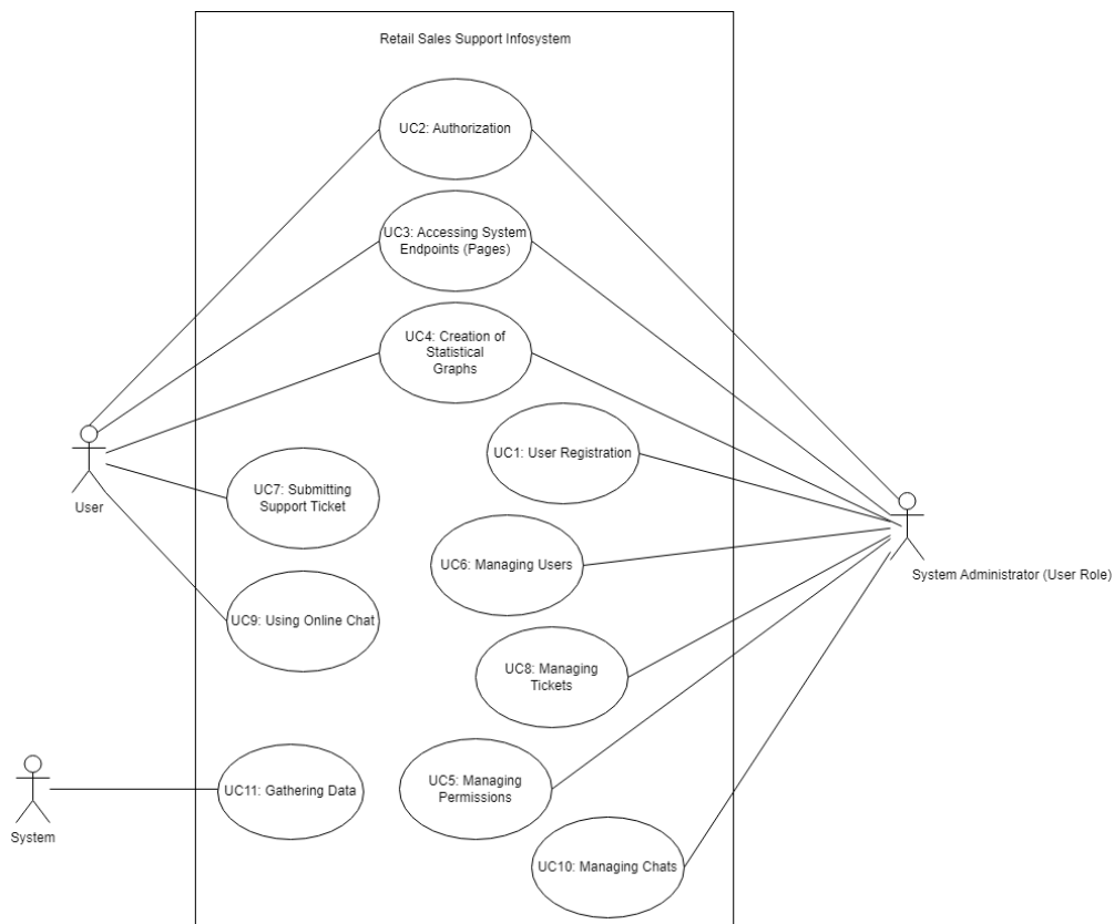
Figure 18. Use Case Model of Retail Sales Support Infosystem. Source: composed by the Author.
